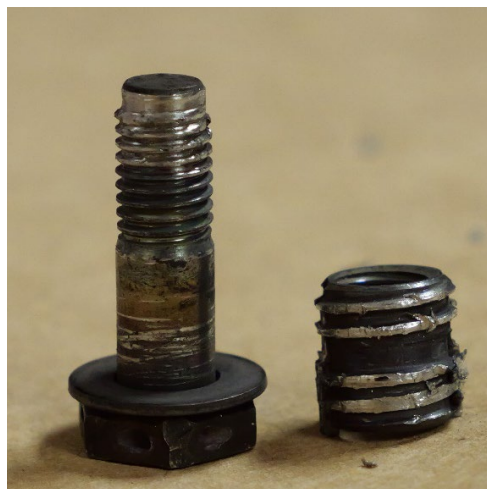
Figure 17: Bolt and insert after removal
