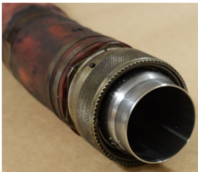
Figure 11: Quick disconnect end of the hose
