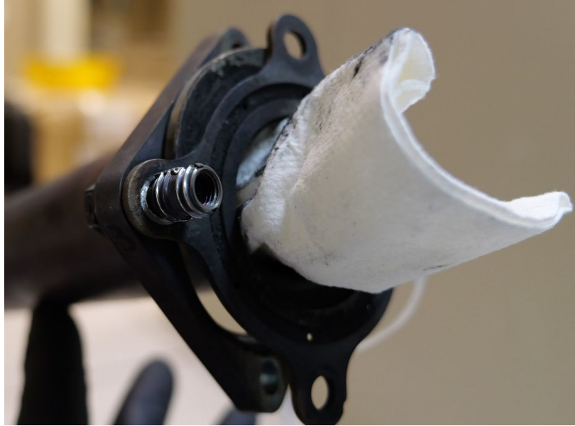
Figure 5: Flanged end of the hose with gasket and insert as received
