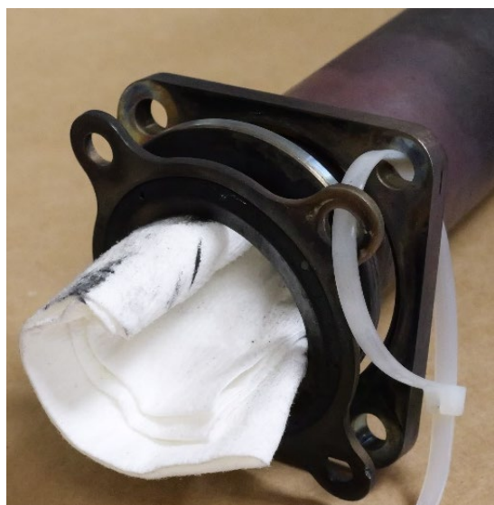
Figure 10: Flanged end of hose with gasket
