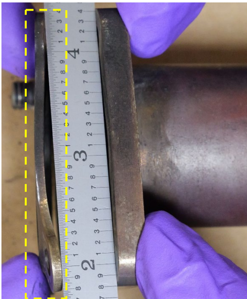
Figure 13: Gasket warped (between holes 1-4)
