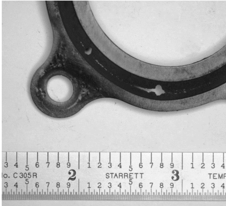
Figure 2. Optical photograph showing the region of the gasket with cracking and material absent.
