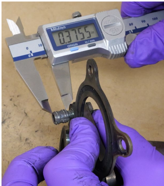
Figure 15: Threaded insert length measured
