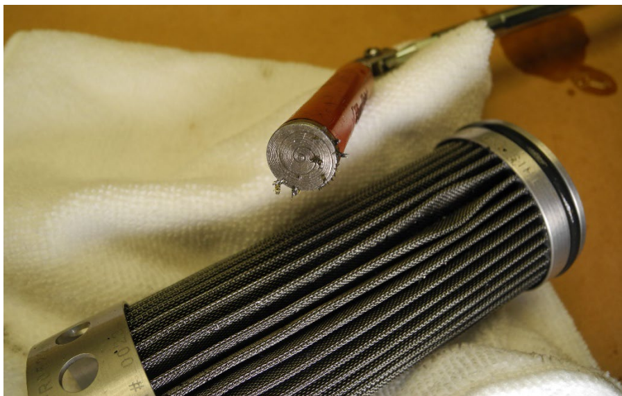
Photo 9 - Oil Filter and Magnet Containing Metal Chips
