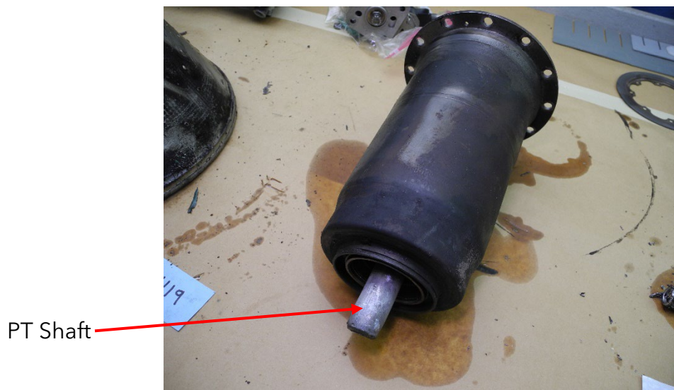
Photo 15 - PT Shaft Housing
