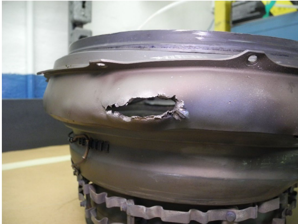
Photo 13 - Power Turbine Stator Housing - Breach in 2 nd Stage PT Plane
