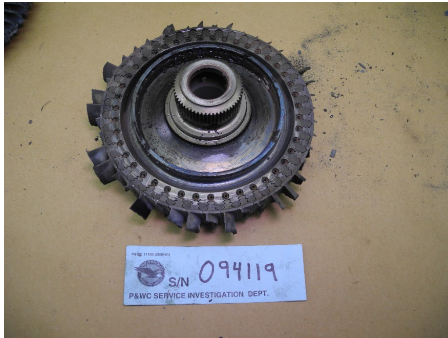
Photo 14 - 1 st Stage PT Rotor
