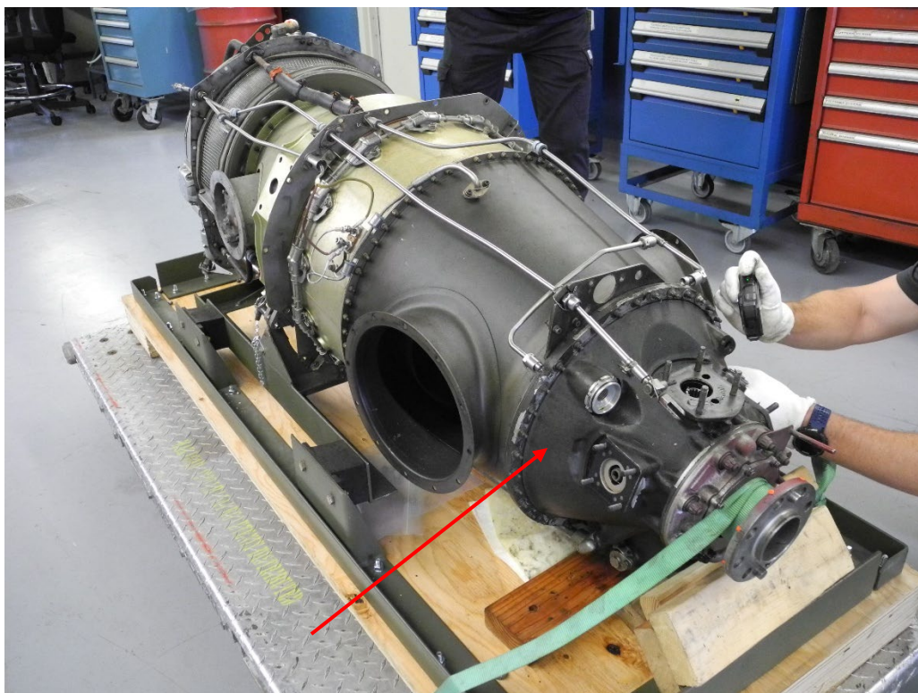
Photo 3 - PT6A-42 S/N 94119 - RGB Missing Silver Colored Protective Coating
