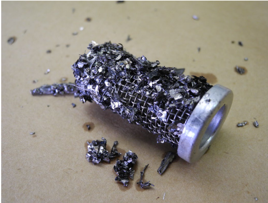
Photo 10 - RGB Oil Screen - Heavily Contaminated with Metal Chips
