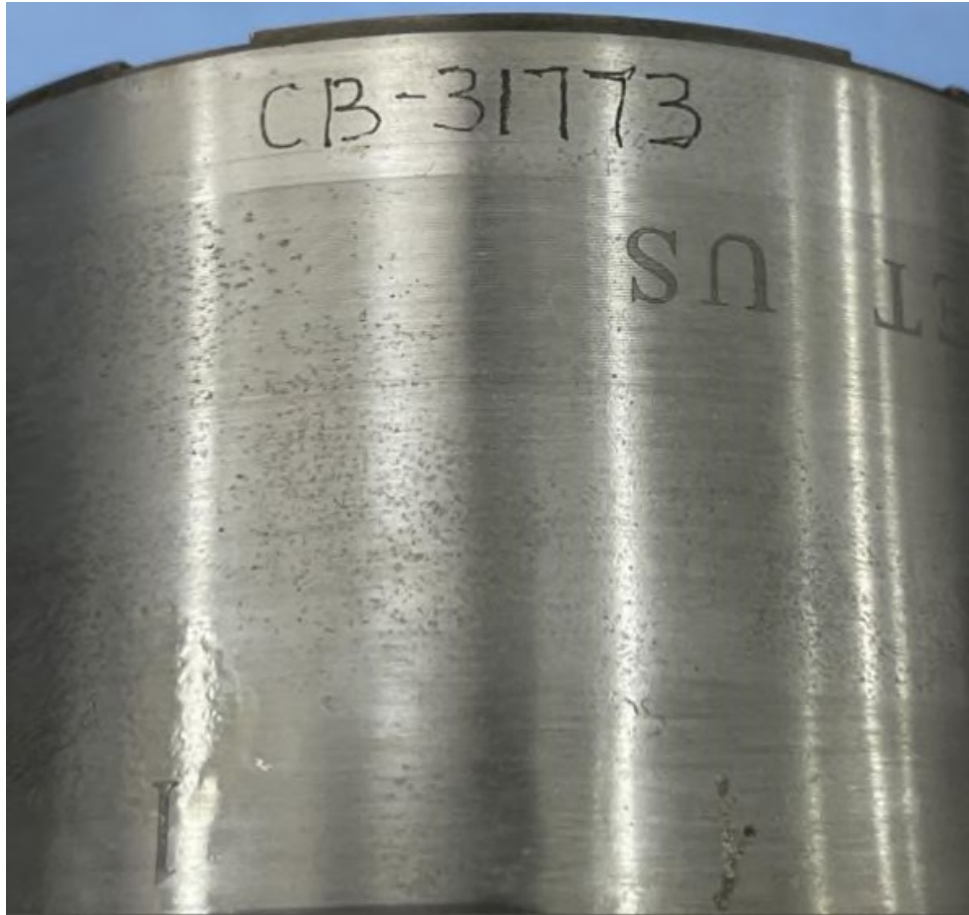
Figure 13. Exterior of the number 2 IDG fixed cylinder block, showing the etched number corresponding to an FAA-approved block re-sleeving process. (Photograph courtesy of Collins Aerospace)
