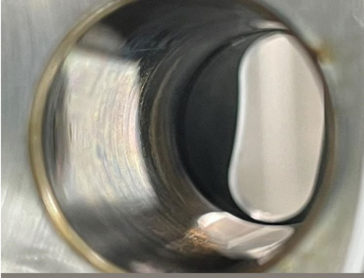
Figure 17. The bottom of variable block bore number 5, showing minimal wear. (Photograph courtesy of Collins Aerospace)
