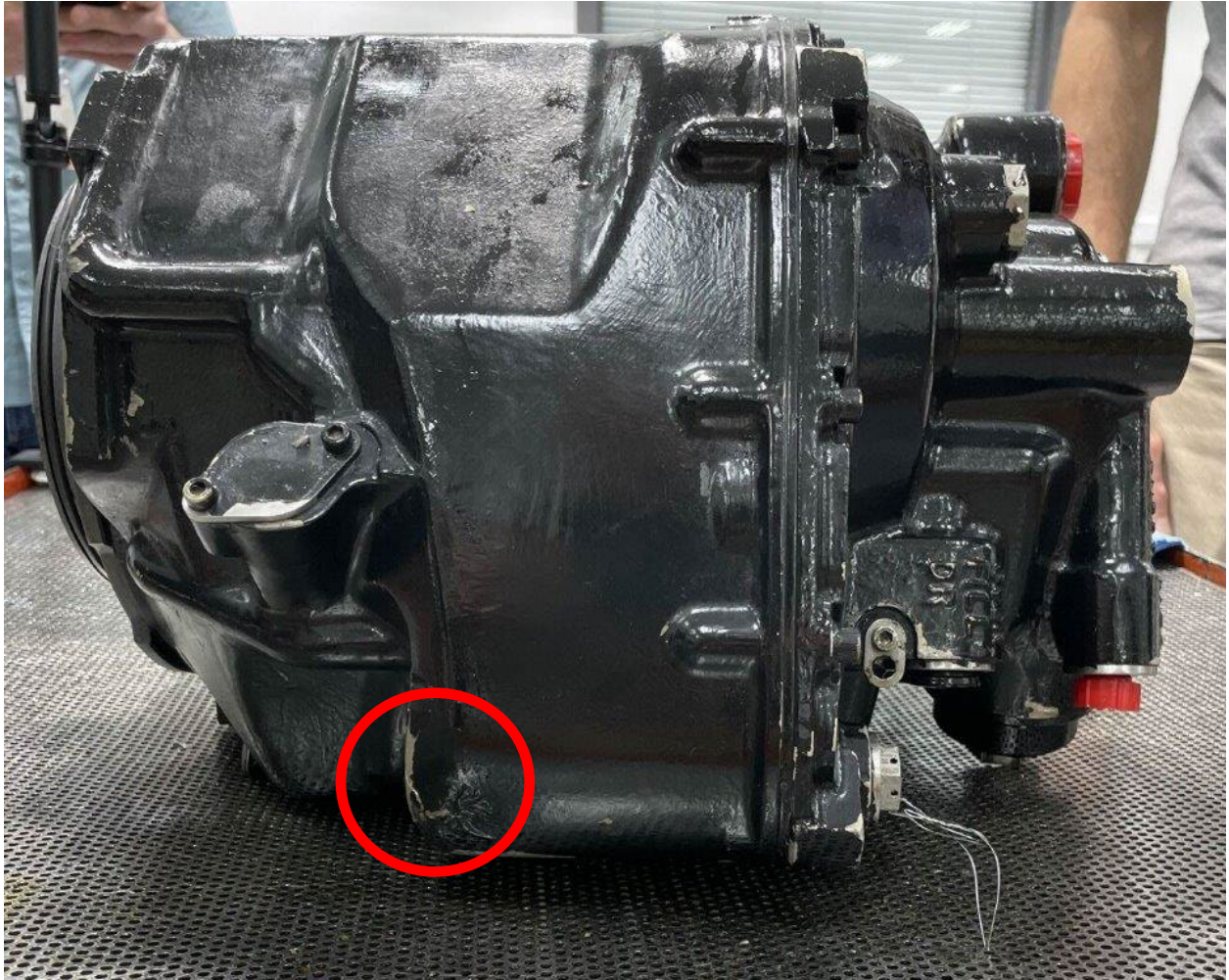
Figure 11. View of the IDG housing with a crack, in the red circle. (Photograph courtesy of Collins Aerospace)
