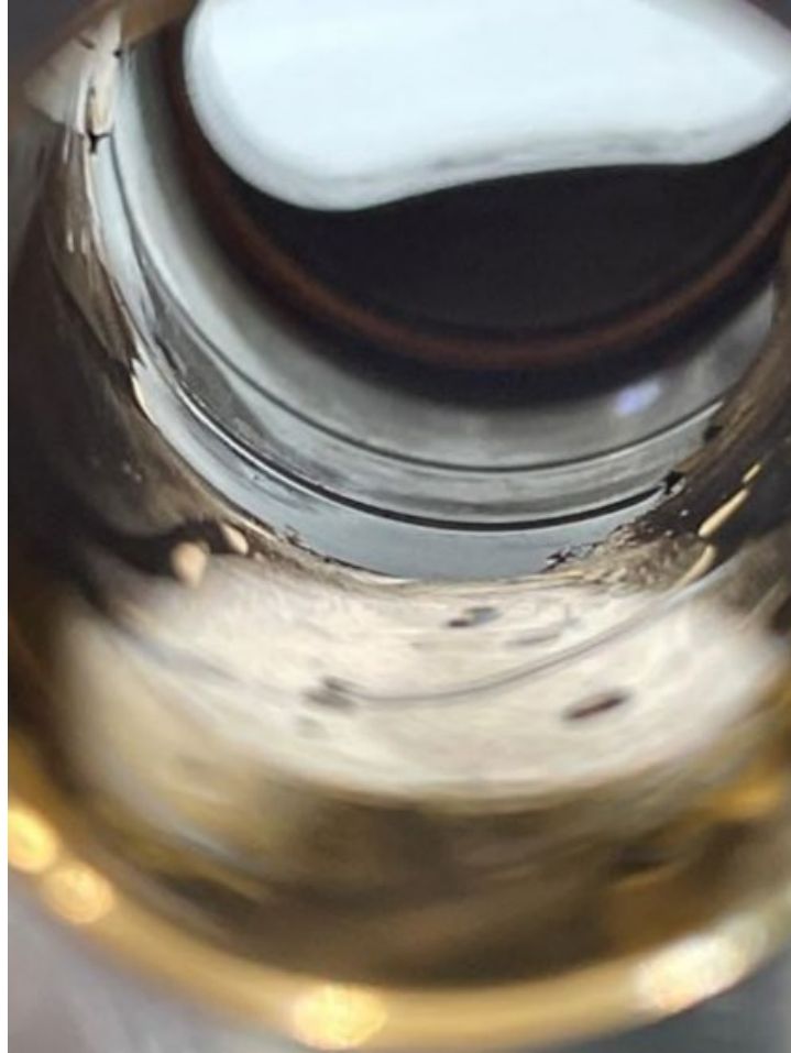
Figure 6. Fixed block bore number 3, showing wear at the bottom of the bore through the sleeve, to the cylinder block steel. (Photograph courtesy of Collins Aerospace)
