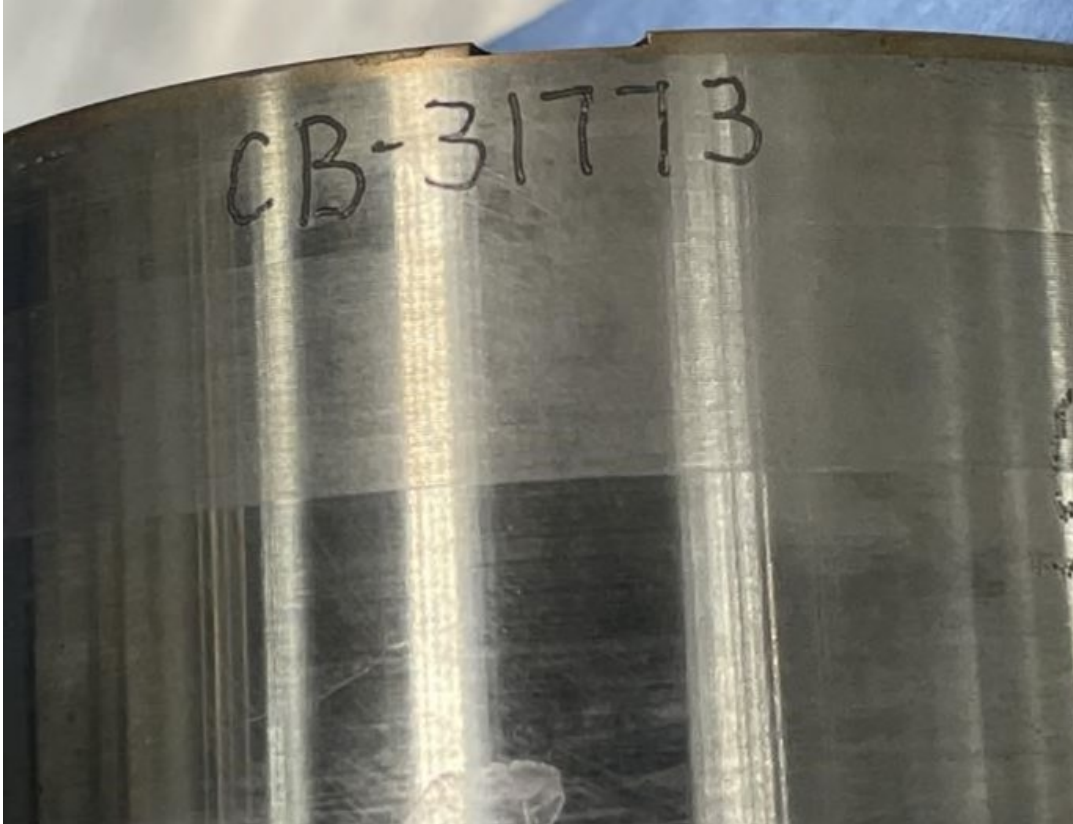
Figure 5. The etched number, indicating the cylinder block had been re-sleeved. (Photograph courtesy of Collins Aerospace)
