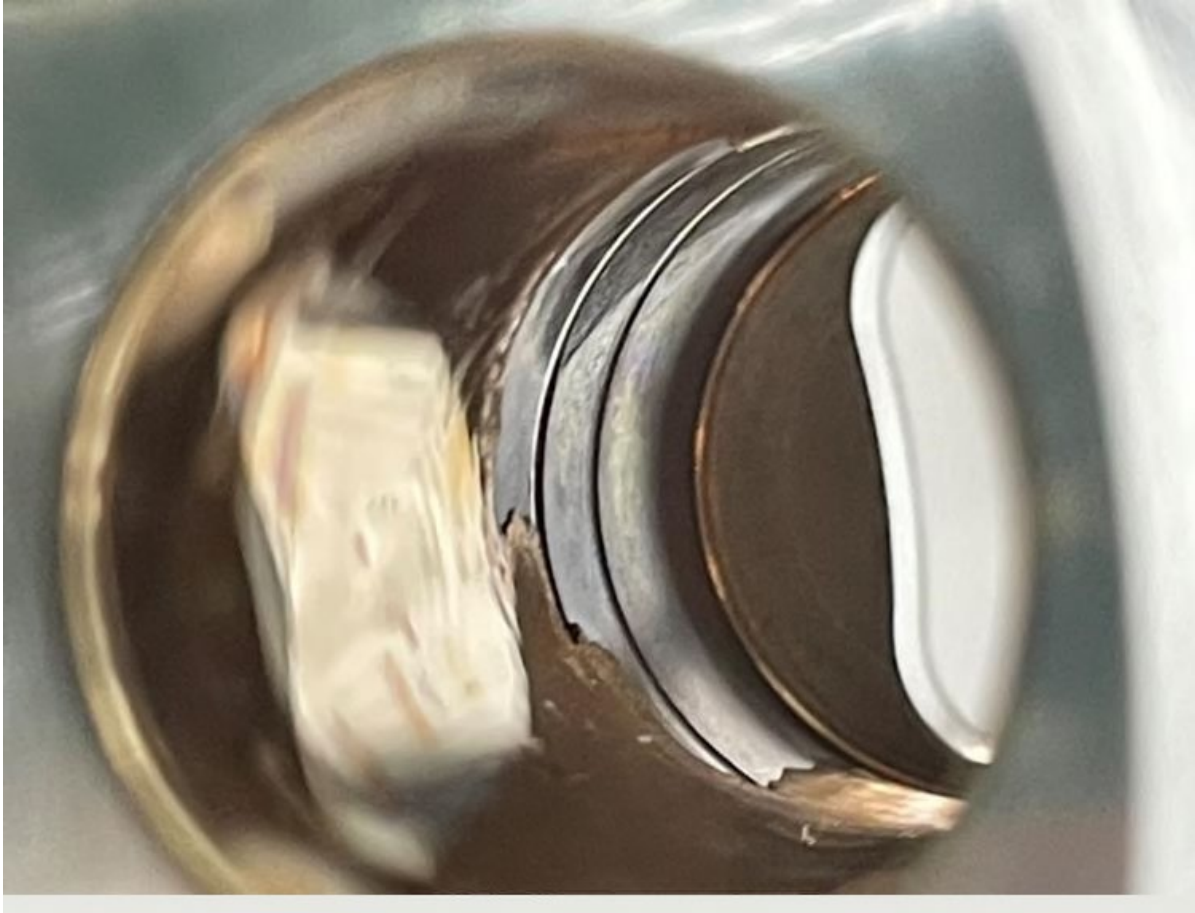
Figure 14. Fixed cylinder block bore number 1, showing wear through the sleeve bushing to the cylinder block steel. (Photograph courtesy of Collins Aerospace)
