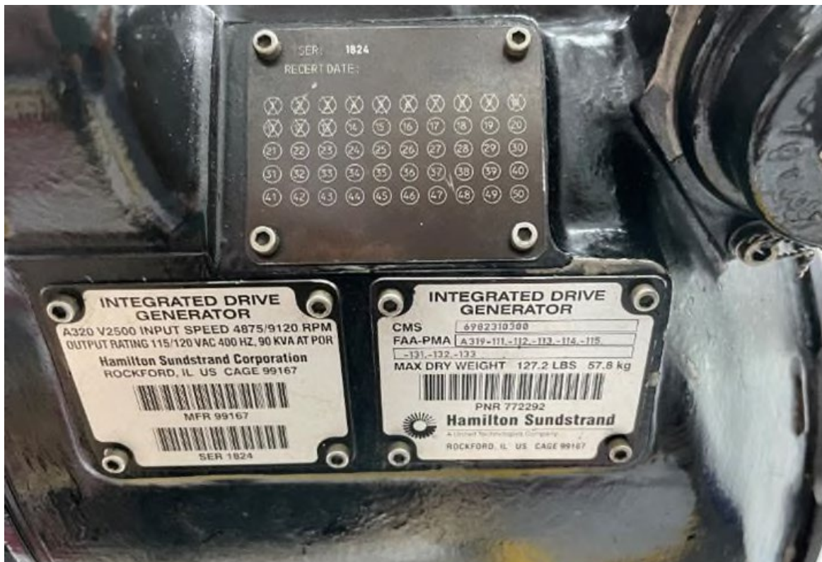
Figure 9. IDG #2 (Serial Number 1824) nameplate. (Photograph courtesy of Collins Aerospace)
