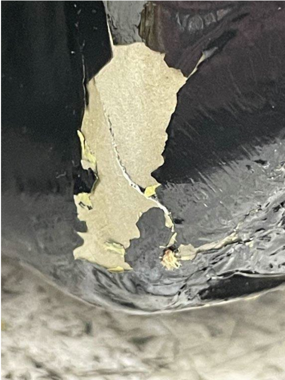
Figure 12. A close-up photograph of the crack found in the IDG housing. (Photograph courtesy of Collins Aerospace)
