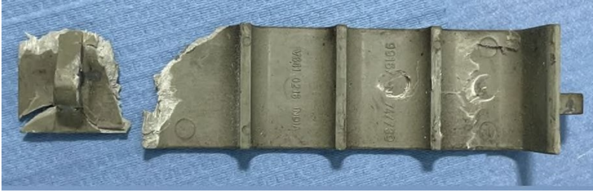
Figure 10. Damage to the terminal block. (Photograph courtesy of Collins Aerospace)
