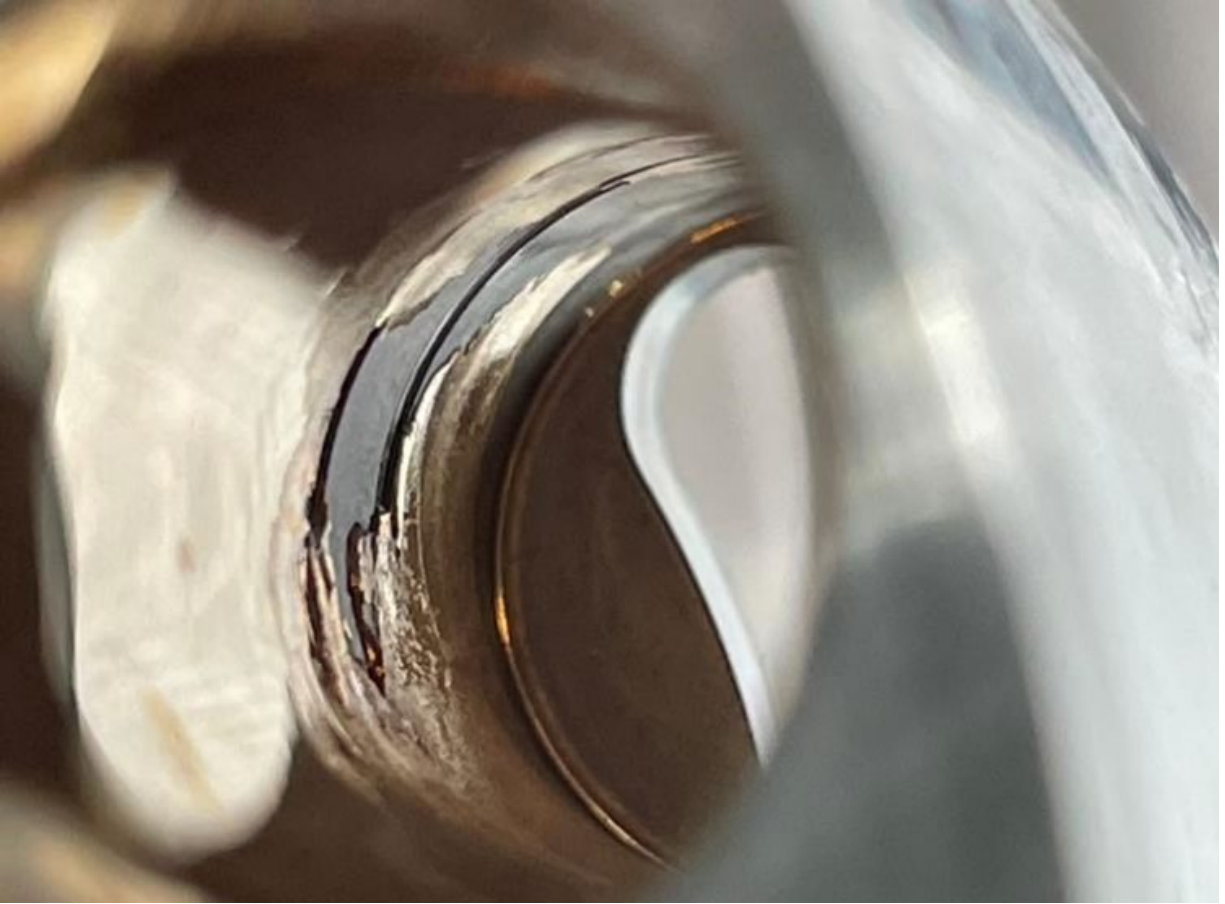
Figure 15. Fixed cylinder block bore number 7, showing wear through the re-sleeved bushing to the cylinder block steel. (Photograph courtesy of Collins Aerospace)
