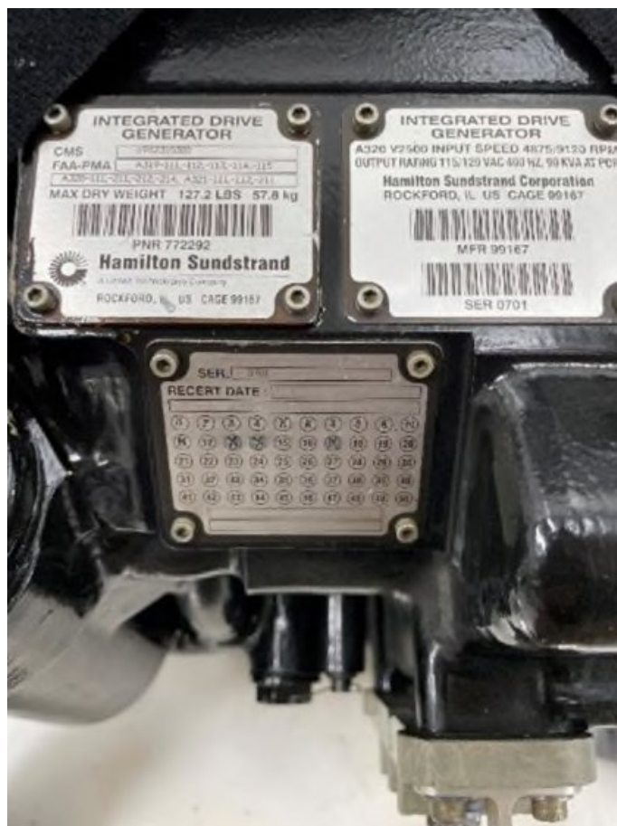
Figure 4. The number 1 IDG, Serial Number 0701 nameplate. (Photograph courtesy of Collins Aerospace)
