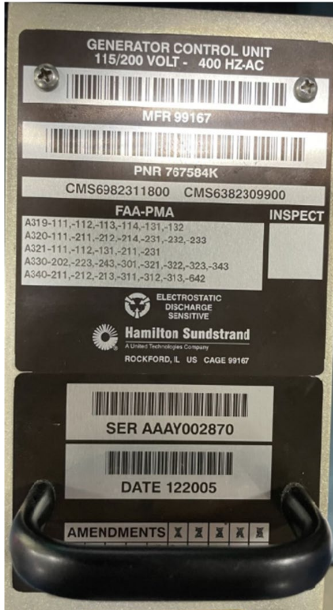
Figure 2. Front data plate of the number 2 GCU. (Photograph courtesy of Collins Aerospace)
