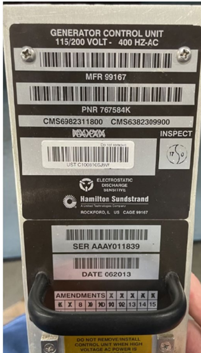
Figure 1. The number 1 GCU, front data plate. (Photograph courtesy of Collins Aerospace)
