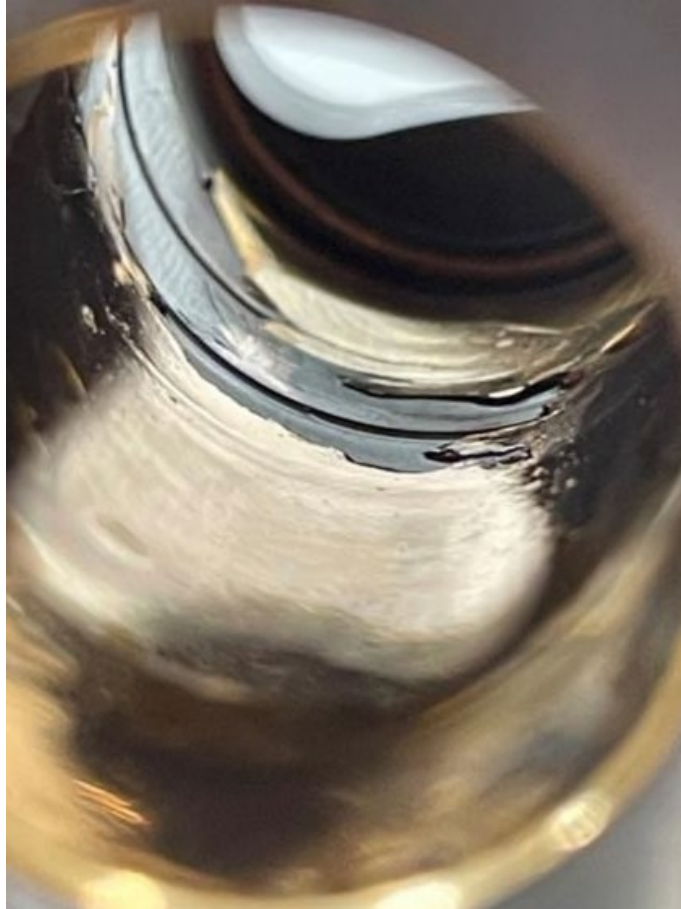
Figure 7. The fixed cylinder block bore number 5, showing typical wear through the bushing sleeve material to the cylinder block steel. (Photograph courtesy of Collins Aerospace)
