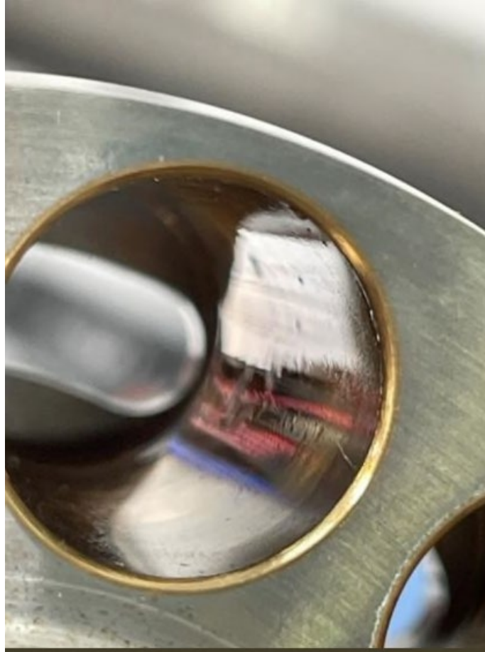
Figure 8. One of the variable cylinder block bores, showing minimal wear. (Photograph courtesy of Collins Aerospace)
