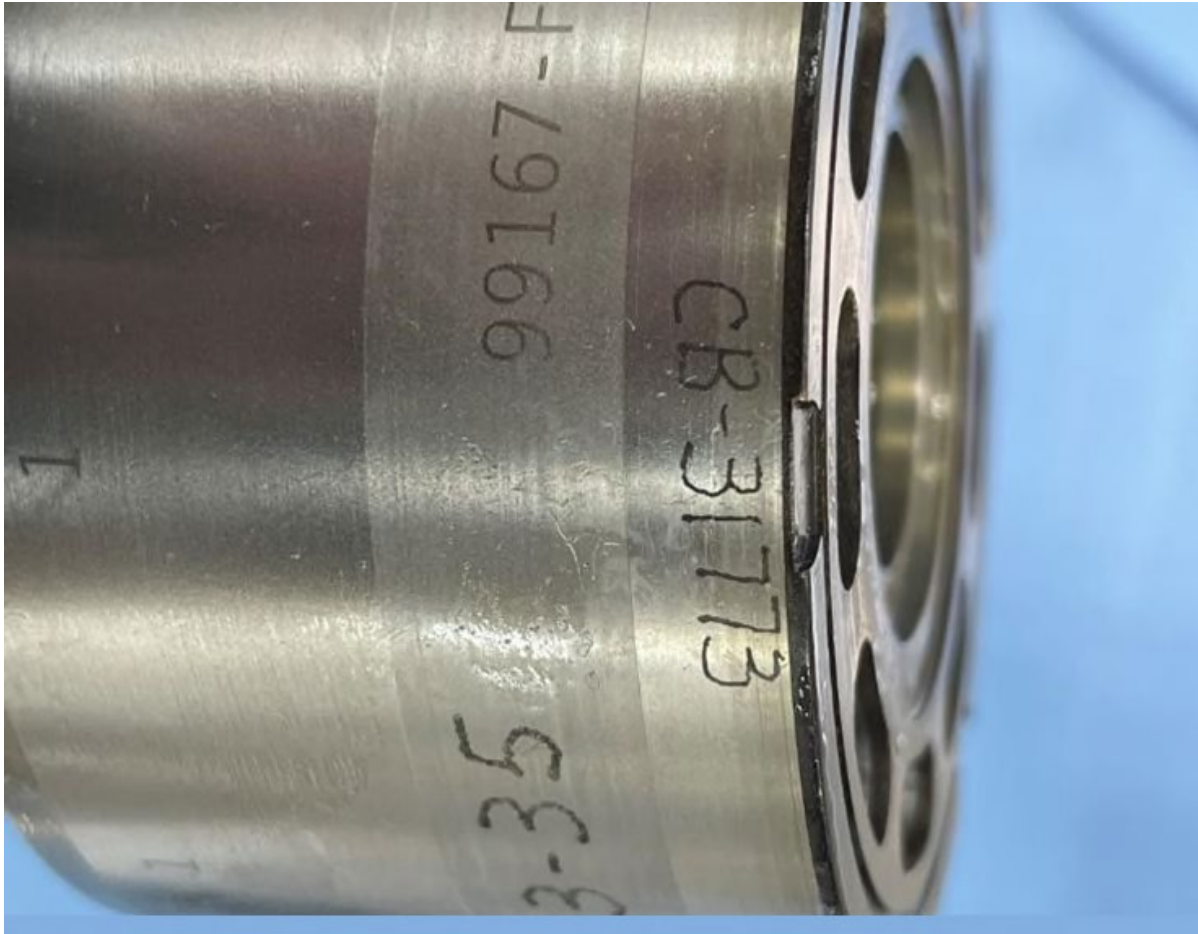
Figure 16. Etching on variable block exterior indicating the block was modified by an FAA-approved re-sleeving process. (Photograph courtesy of Collins Aerospace)
