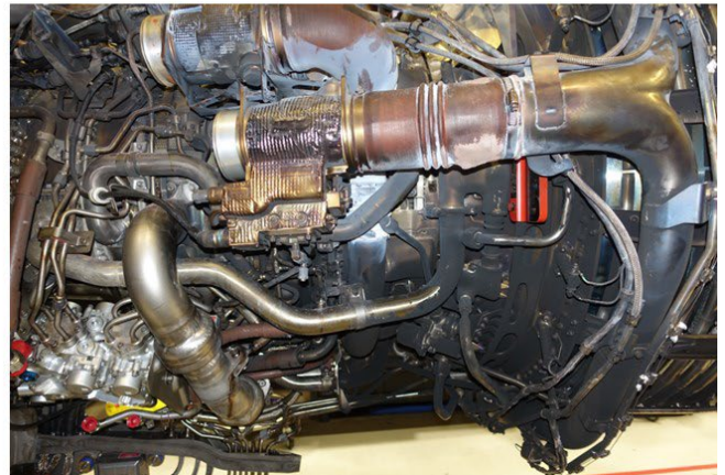
Photo 7- Left Side of Engine, Lower Core Discoloration
