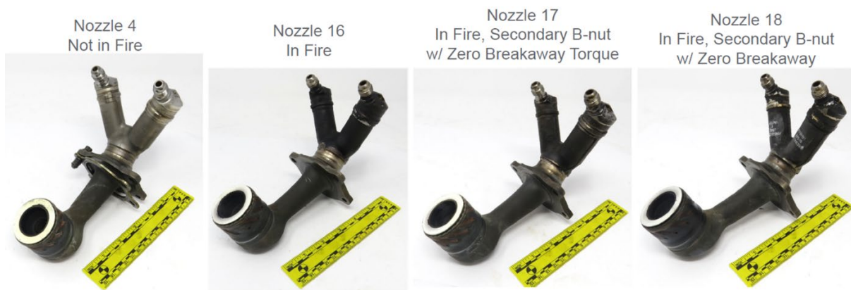
Photo 13- Fuel Nozzles 4, 16, 17, and 18 as Received at the GE Aerospace FA Laboratory
