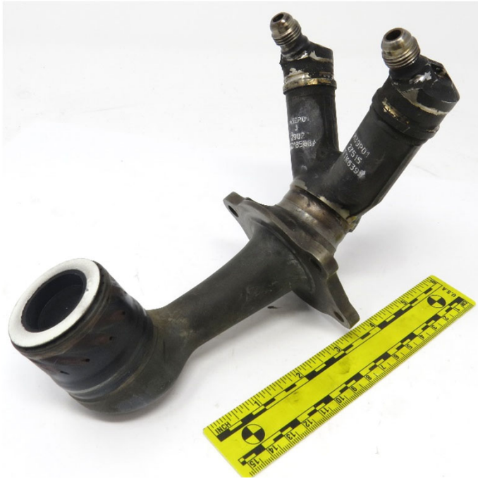
Nozzle 18 In Fire, Secondary B-nut w/ Zero Breakaway
