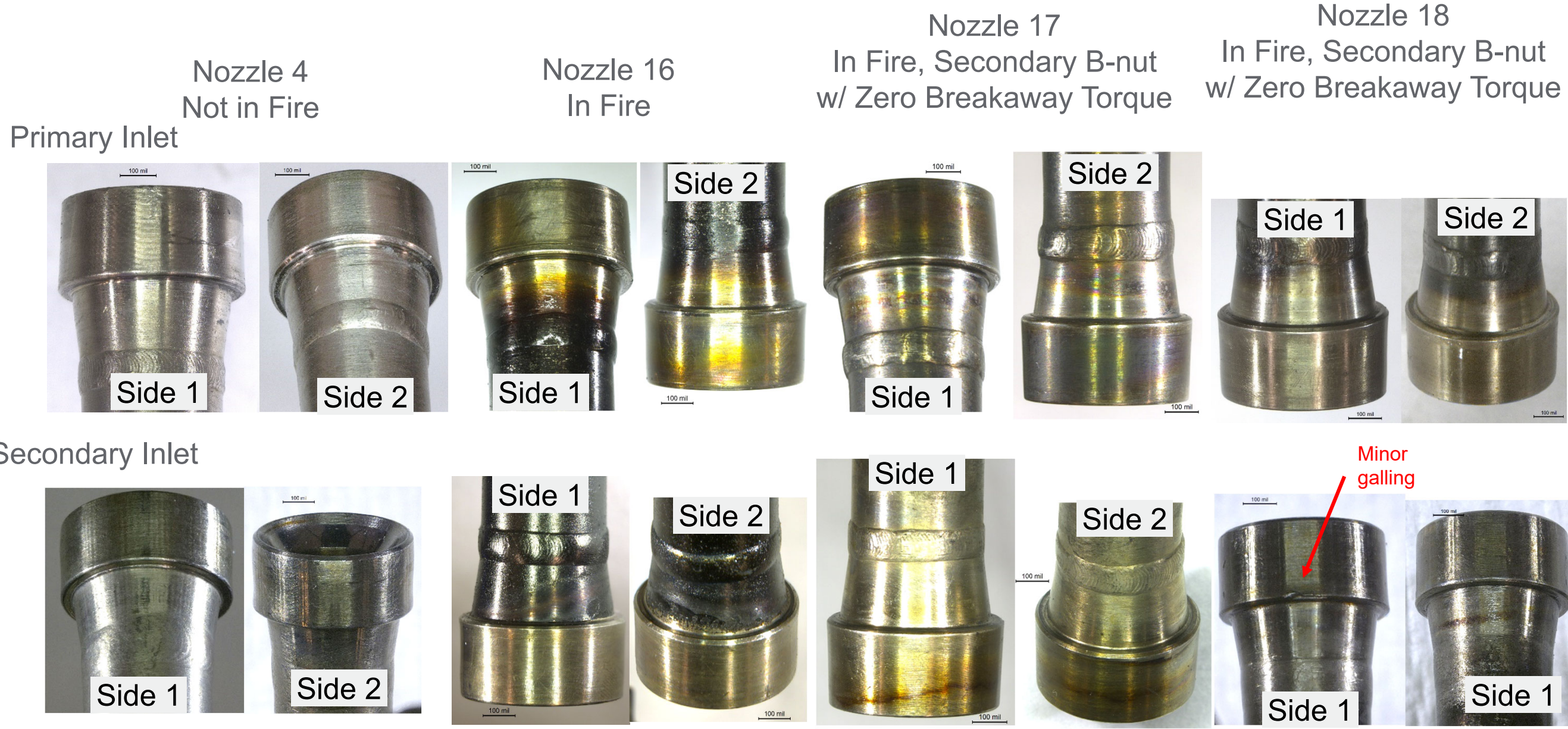
Figure 6: The fuel manifold ferrules were inspected for damage that would result in a lack of sealing. Macrographs show no indication of galling, cracking, or mechanical deformation present at fuel manifold ferrules.
