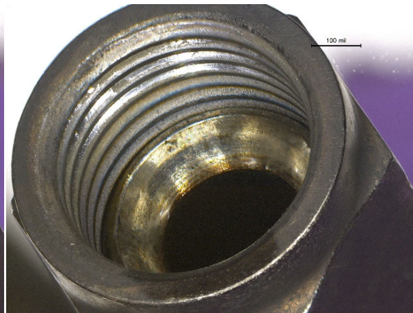
Nozzle 17 In Fire, Secondary B-nut w/ Zero Breakaway Torque
