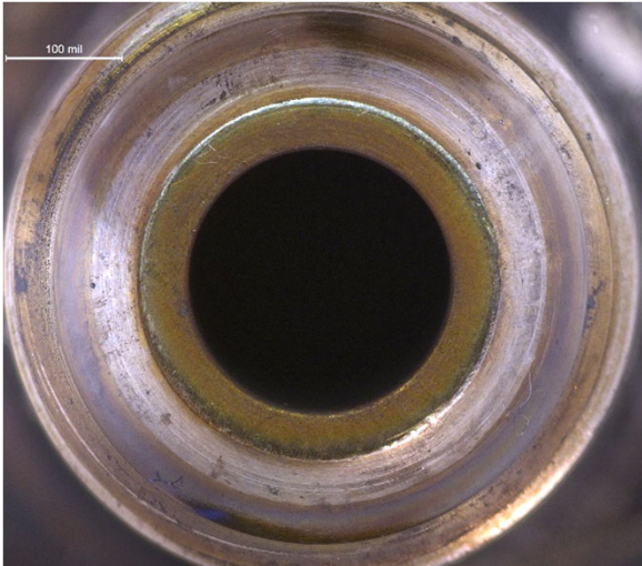
Nozzle 17 In Fire, Secondary B-nut w/ Zero Breakaway
