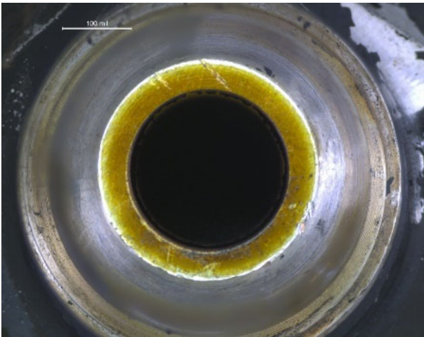
Nozzle 18 In Fire, Secondary B-nut w/ Zero Breakaway Torque
