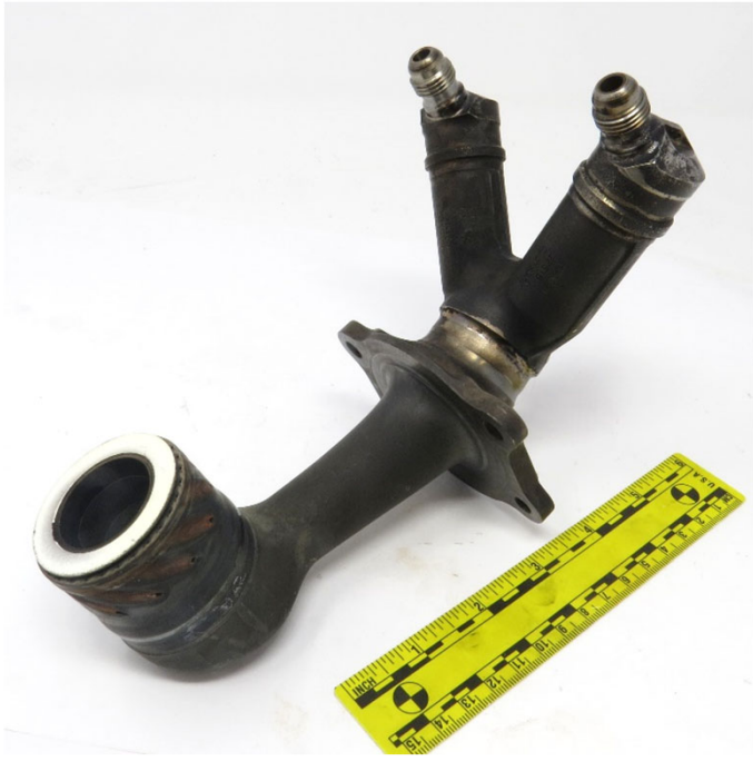
Nozzle 17 In Fire, Secondary B-nut w/ Zero Breakaway Torque
