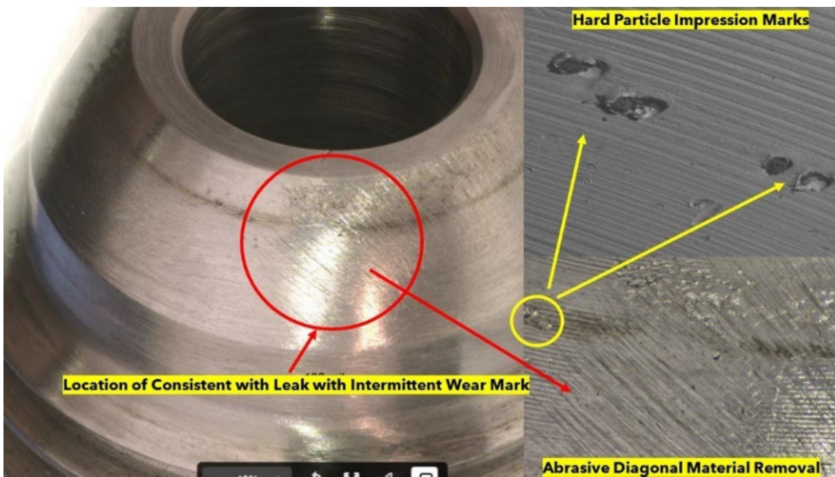
PHOTO 18: No. 18 FN MALE BULLNOSE WITH ABRASIVE MARKS AND PARTICLE IMPRESSION
