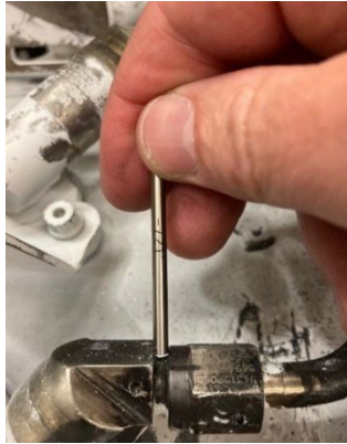
PHOTO 5: B-NUT GAP CHECK AND TORQUE MEASUREMENT
