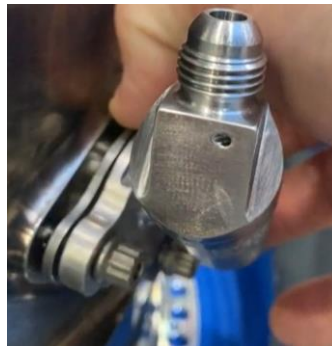
Fuel nozzle being assembled
