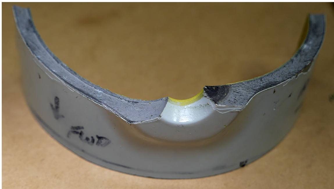
Figure 18: Forward portion after sectioning
