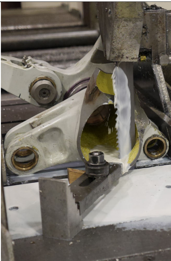
Figure 15: Aft portion mounted during sectioning by bandsaw
