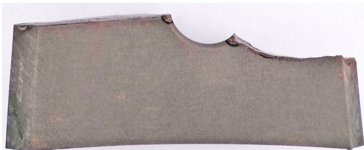
Figure 35: Portion F4 after stripping and nital etch
