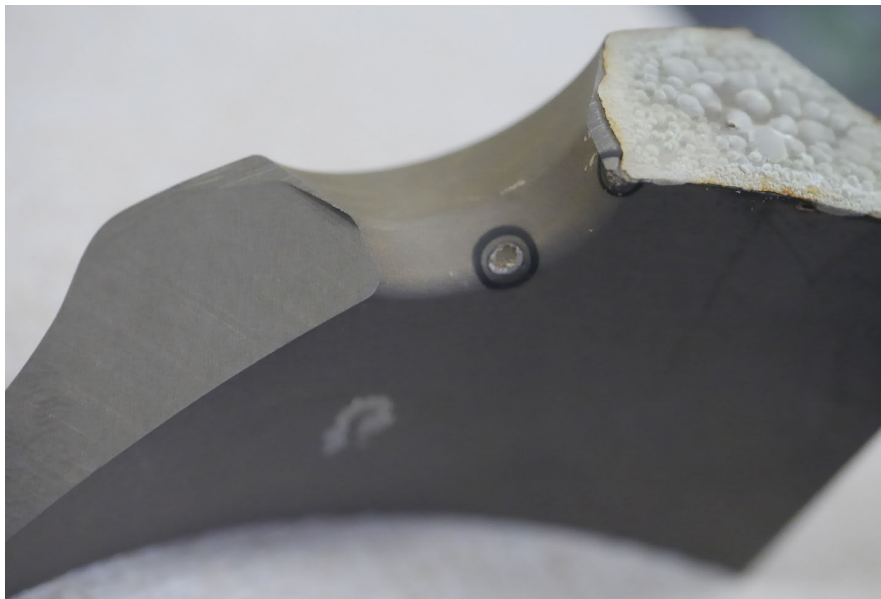
Figure 34: A2C portion after stripping and nital etch
