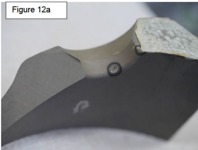
Figures 12a and 12b. Nital Etch inspection of section Aft section A2b (from cut out shown above) and the Forward section showing presence of under tempered (light etching at the center of the indication) and overtempered martensite (dark etching rings). (Close up of etch inspection indication shown in Figure 13)
