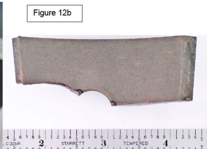
Figures 12a and 12b. Nital Etch inspection of section Aft section A2b (from cut out shown above) and the Forward section showing presence of under tempered (light etching at the center of the indication) and overtempered martensite (dark etching rings). (Close up of etch inspection indication shown in Figure 13)
