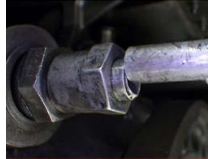
Broken Oil Tube on AGB
