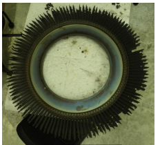
4a. LPT S1,2,3 Severe rubs, airfoil cracking at midspan
