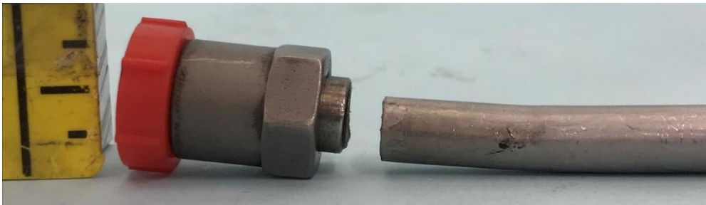
Fractured oil tube showing plastic deformation and a planar fracture consistent with fatigue/cyclic tensile.
