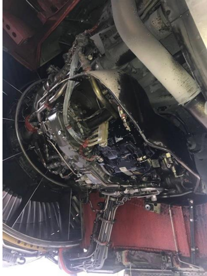
Distress observed on engine and Cowl doors from engine fire
