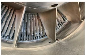
4b. Exhaust nozzle, TRF cracking
