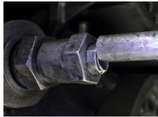
5. Broken Oil Line
