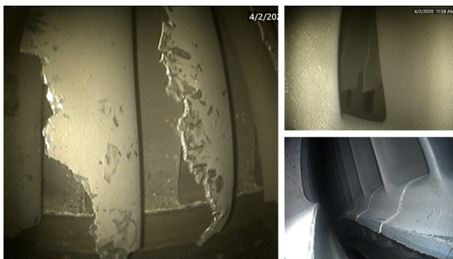
PHOTO 27: LPT STAGE 1 BLADE DAMAGE
