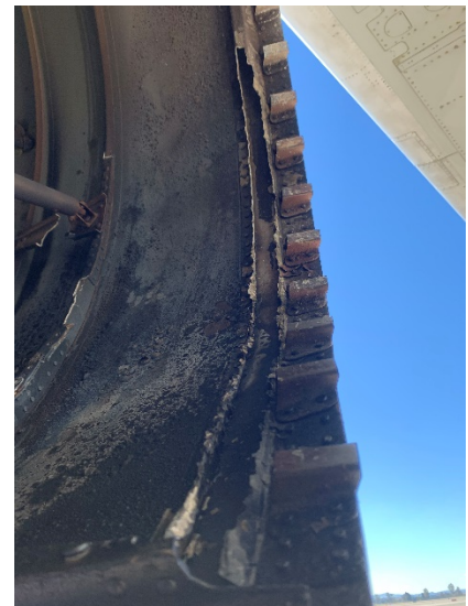
PHOTO 11: AFT END THERMAL DISTRESS
