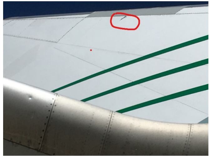
PHOTO 14: VERTICAL STABILIZER DAMAGE
