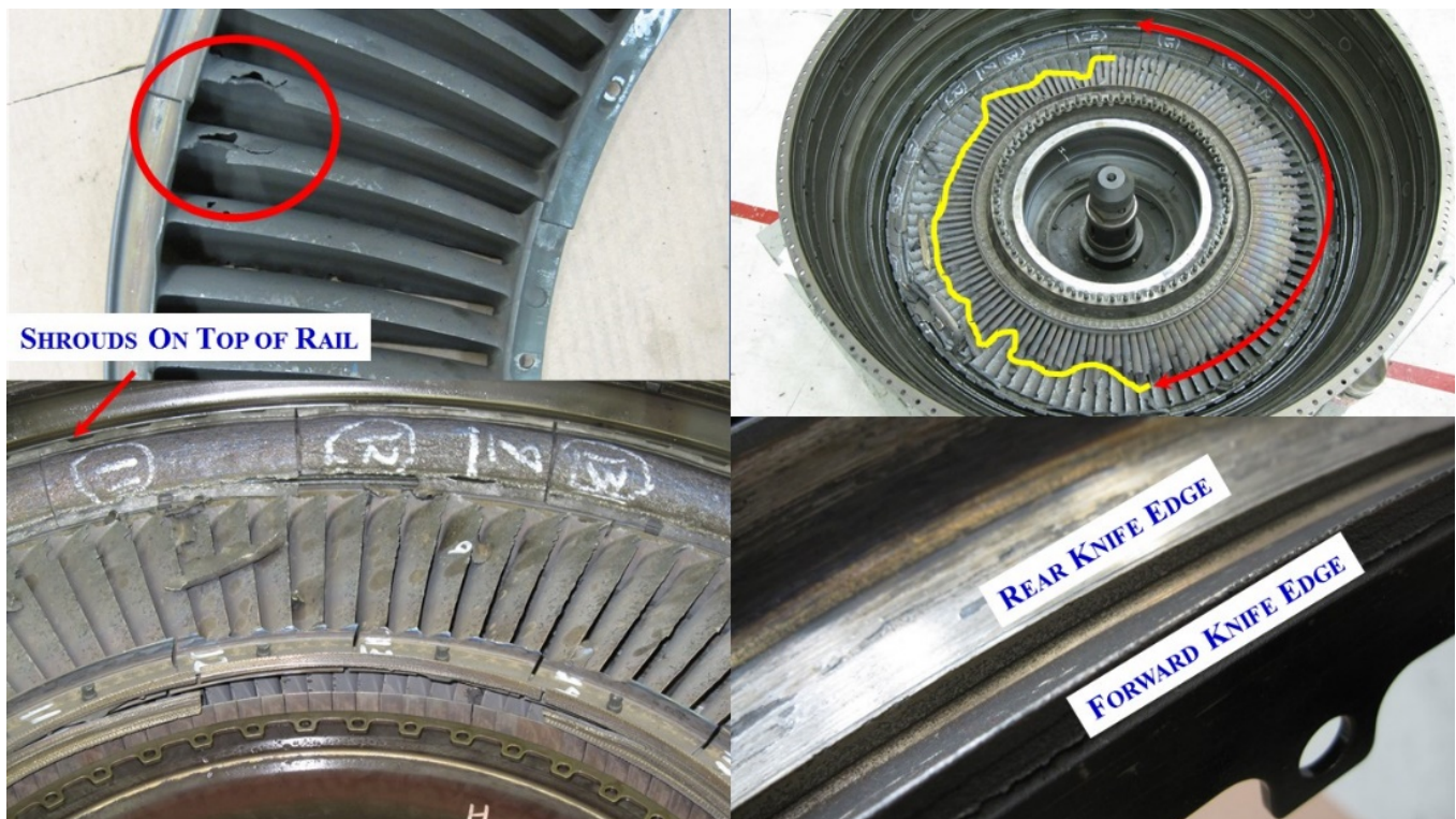
PHOTO 40: LPT STAGE 2 DAMAGE
