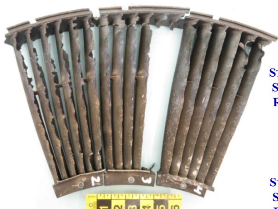
STAGE 5 NOZZLE SEGMENTS NOS. 2-4
