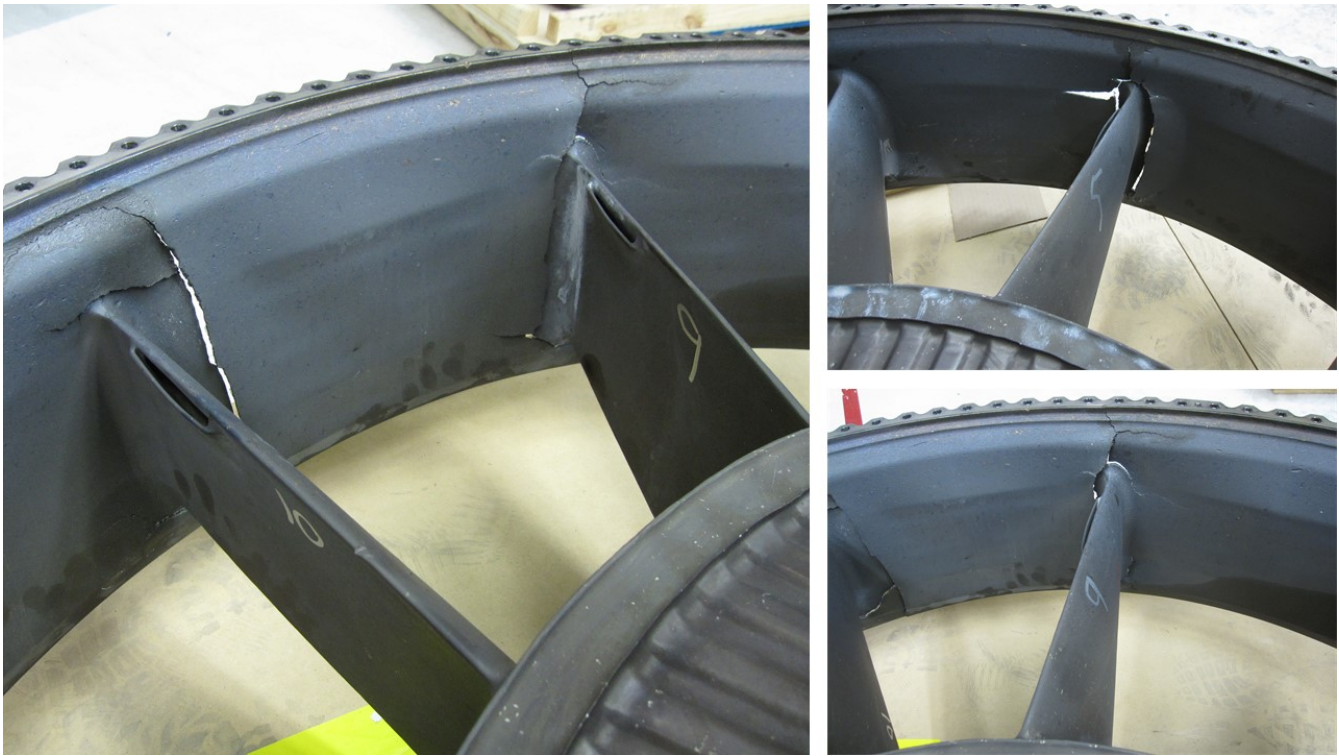
PHOTO 34: TRF CASE OPENINGS AT STRUTS NO. 5, 9, AND 10
