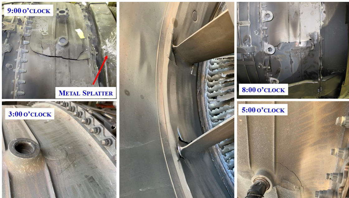
PHOTO 20: TURBINE REAR FRAME DAMAGE
