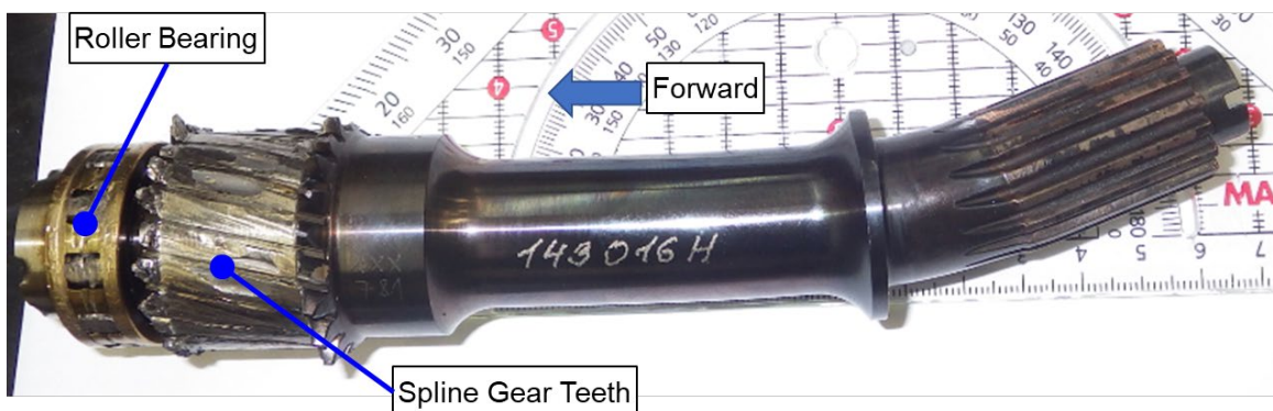
Photo 12: Quill Shaft As-Received
