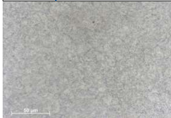
PT shaft (representative microstructure)
