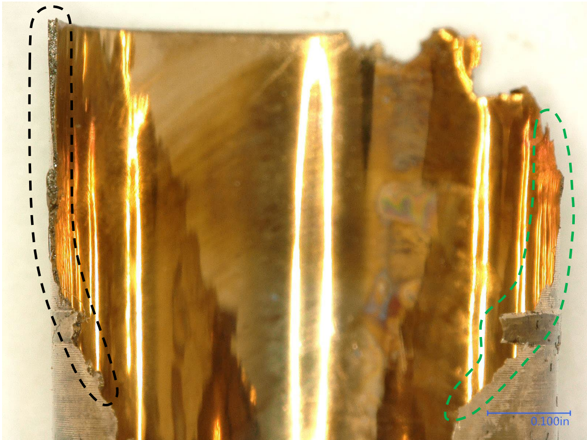
Figure 11: Digital microscope image showing the edges along the missing segment in the liner removed from bore 5 in fixed cylinder block S/N Y10-245-19. One edge (green dashed line) had thinned down to a knife edge. The other edge (black dashed line) was thicker and had features consistent with the liner separating in pieces.
