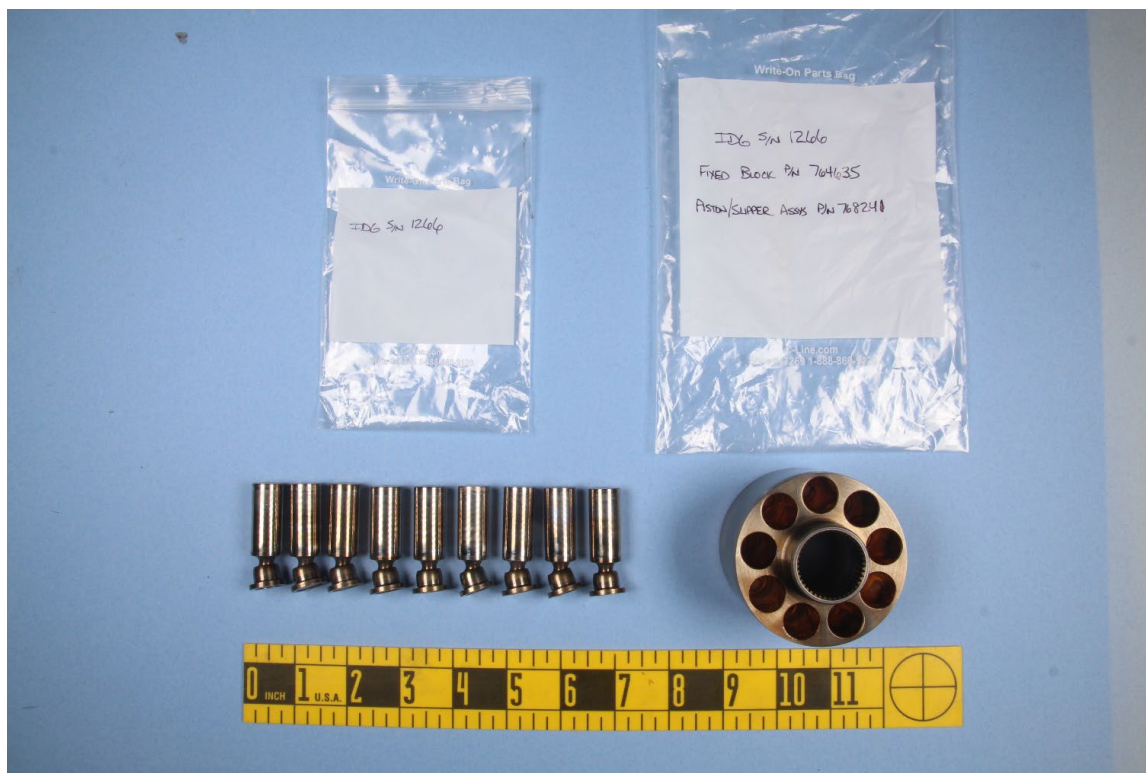
Figure 1: Overall photo showing the packaging with identifying information and the components from the IDG from engine S/N 1266.
