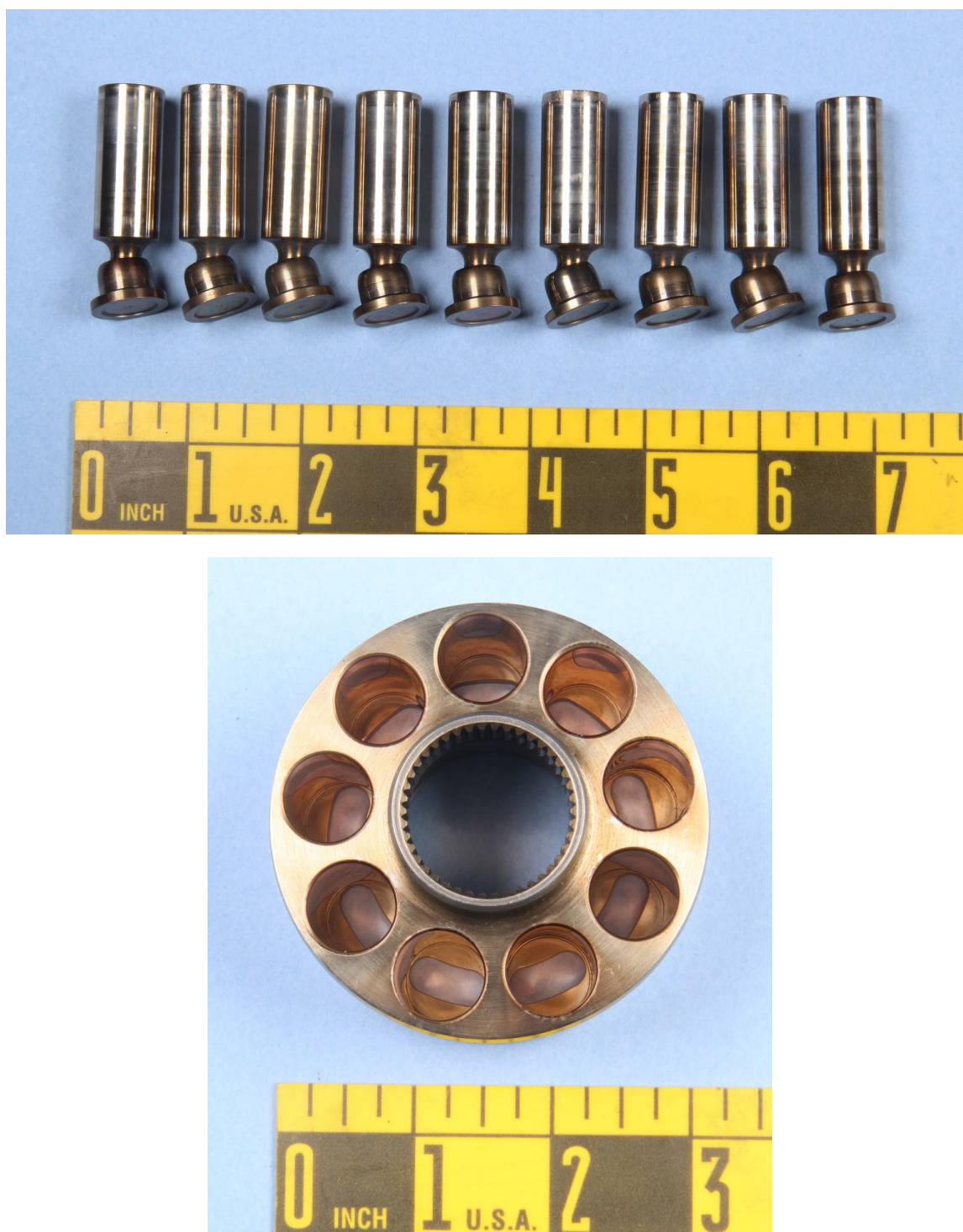
Figure 2: Close up photos of the pistons (top) and fixed cylinder block from engine S/N 1266. The fixed cylinder block was labeled S/N Y10-245-19.
