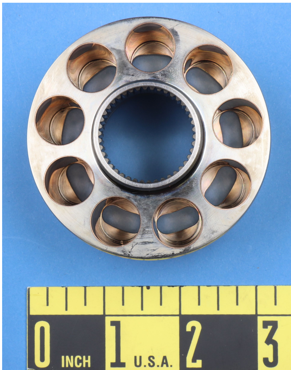
Figure 35: Overall photo of the exemplar fixed cylinder block submitted by the OEM.
