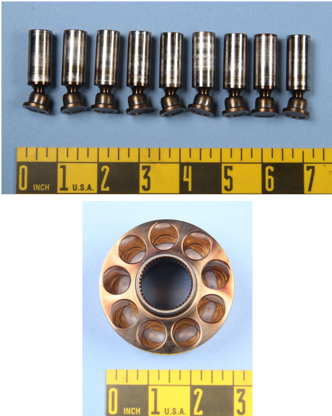
Figure 28: Close up photos of the pistons (top) and fixed cylinder block from engine S/N 1157. The fixed cylinder block was labeled S/N Y04-232-49.
