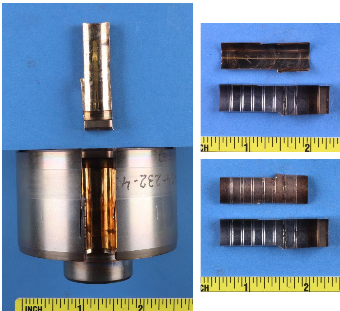
Figure 32: Overall and close-up photos of the pieces of liner and OD block side wall sectioned from bore 7 in fixed cylinder block S/N Y04-232-49.
