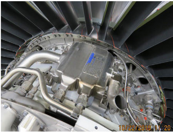
Photo 7- (L) Buffer Air Heat Exchanger on Engine, (R) LPC Mid Case Crack Under Exchanger
