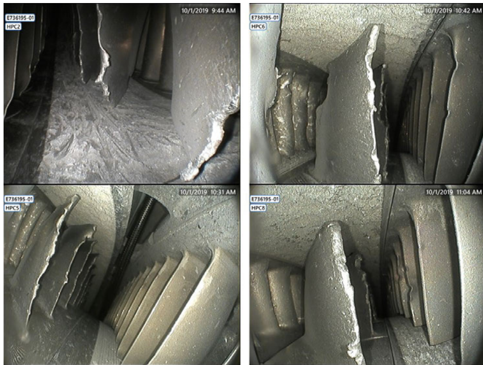
Photo 18- HPC Borescope Photos
