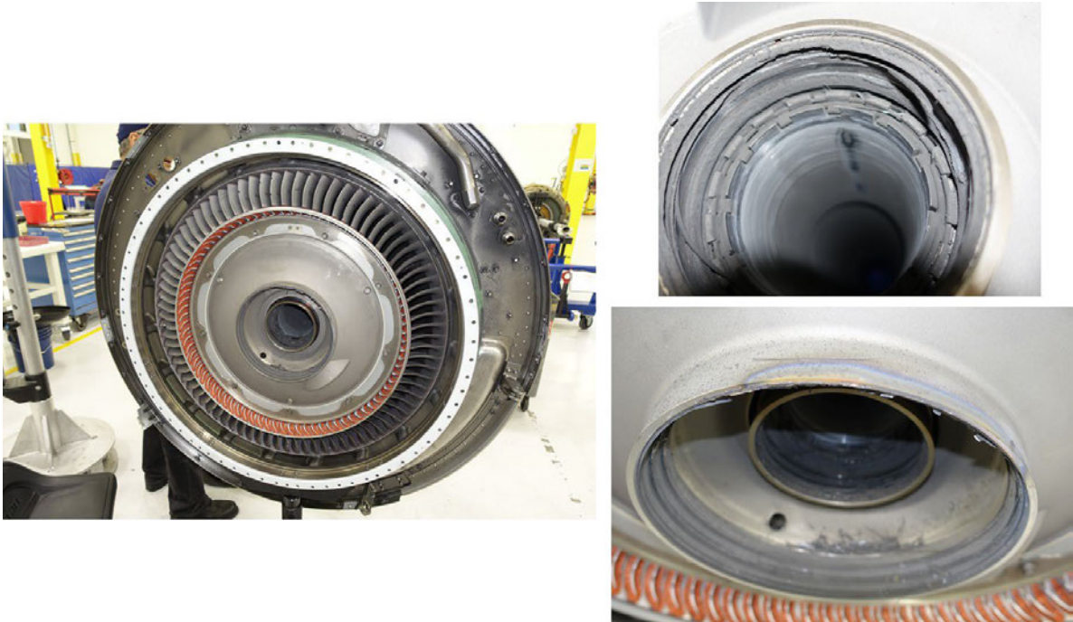
Photo 22- No. 3 Bearing Seal Support and HPC Front Hub Inner Diameter Rub
