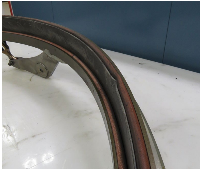
Photo 16- 2.5 Bleed Air Ring Damage
