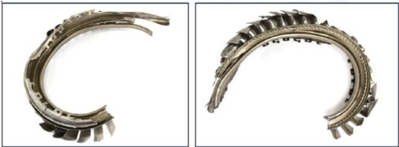
Photo 25- Engine Serial Number P736195 LPC IBR 1, as Received
