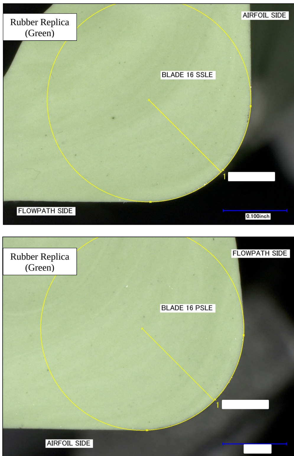
Figure 13. Views showing the root radius measurement at the pressure and suction side leading edge of blade no. 16.
