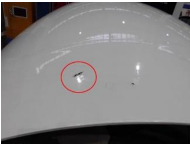
Photo 4- Left Thrust Reverser Sleeve Outer Skin Penetration, 8:30 Position
