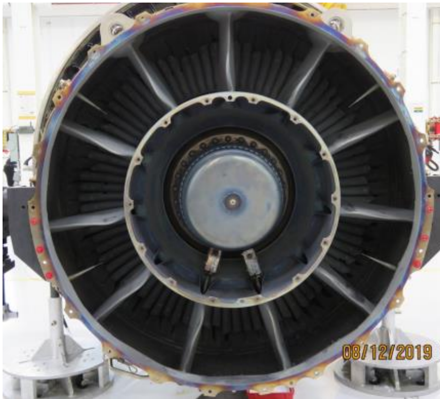
Photo 13- LPT Stage 3 Blades Visible Through TEC
