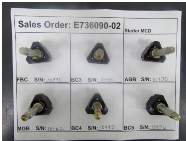
Photo 14- MCDs, as Received at Columbus Engine Center (Photo Courtesy of Pratt & Whitney)
