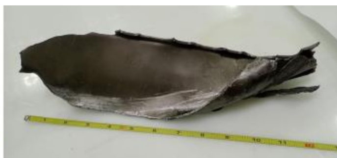
Photo 9- Engine Fragment Recovered in Nacelle
