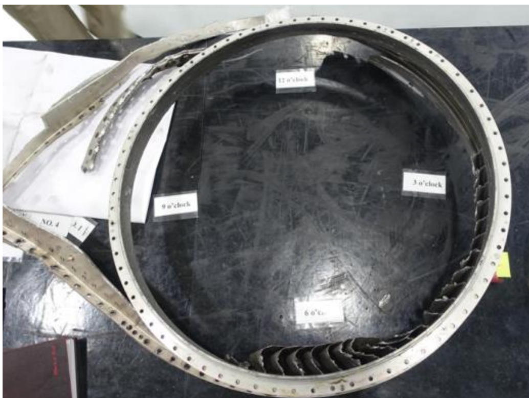
Photo 17- LPC S1 Stator
