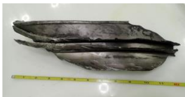
Photo 9- Engine Fragment Recovered in Nacelle
