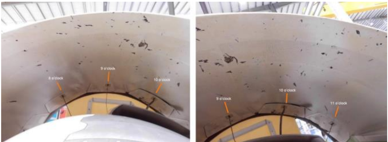
Photo 1- Left Thrust Reverser Sleeve Perforated Skin Impact Damage
