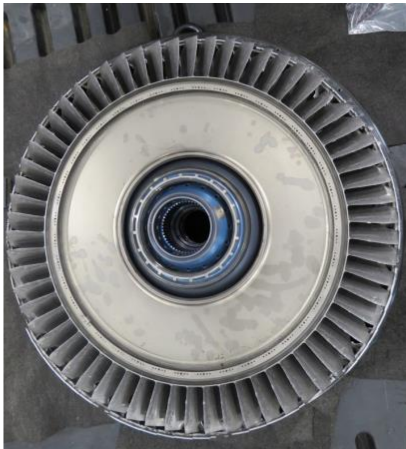
Photo 20- LPC IBR 3, Aft Side
