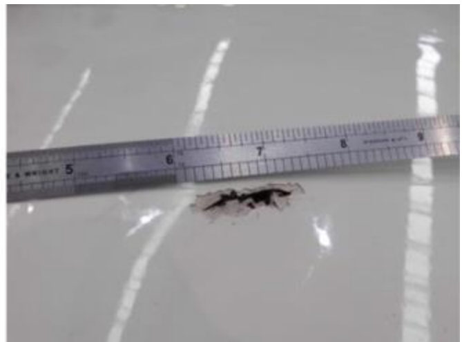
Photo 4- Left Thrust Reverser Sleeve Outer Skin Penetration, 8:30 Position
