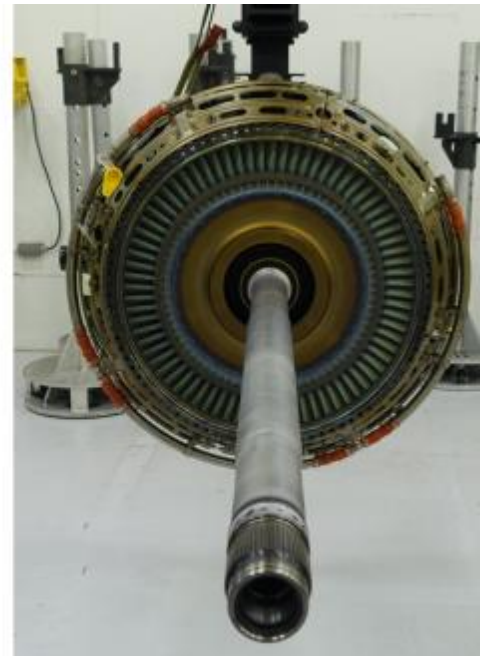
Photo 23- LPT Shaft, (L) Aft End, (R) LPT S1 Blades, Leading Edge
