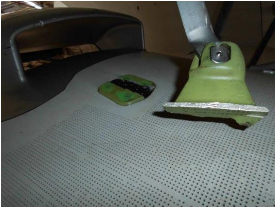
Photo 3- Left Thrust Reverser Blocker Door #9 Drag Link, Pivot Block Sheared at Inner Fixed Structure Attachment
