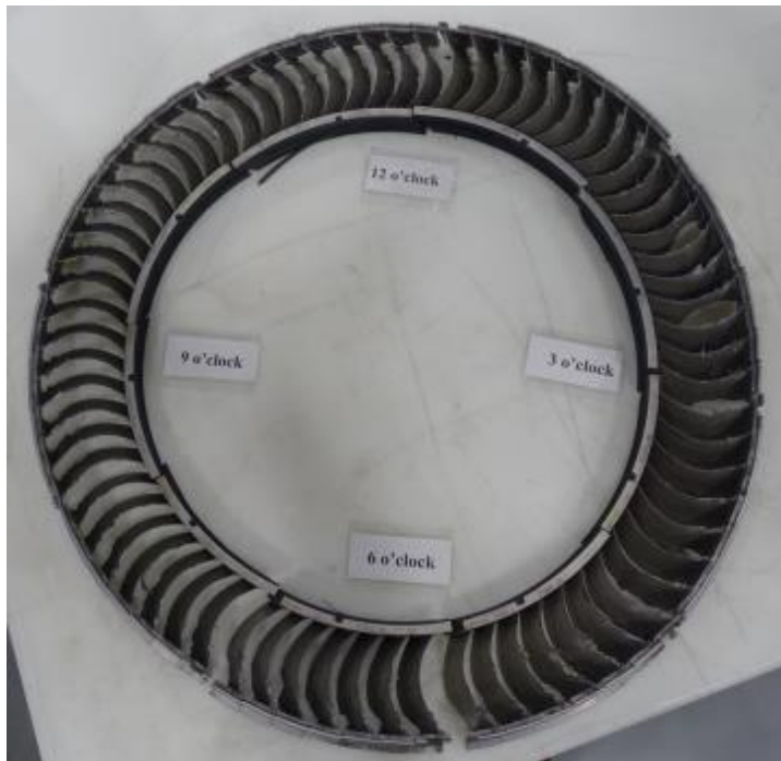
Photo 19- LPC S2 Stator, Aft Side
