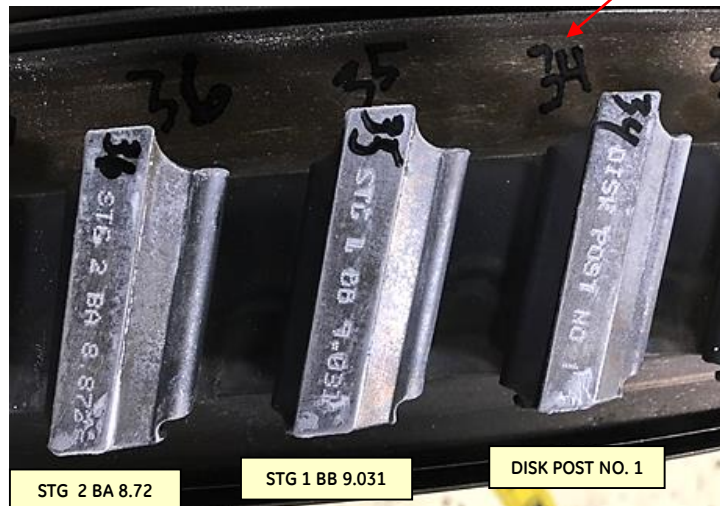
Figure 76. Photographs showing part numbers present on Stg. 1-2 HPC Spool on top surface of Stg. 1 disk posts.
