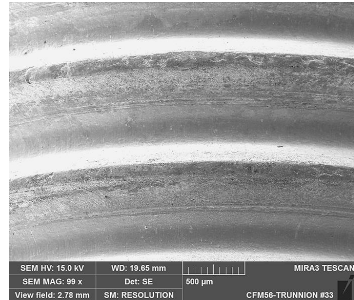
Stg. 1 Vane Trunnion #33 - Lower Thread Contact - SEI
