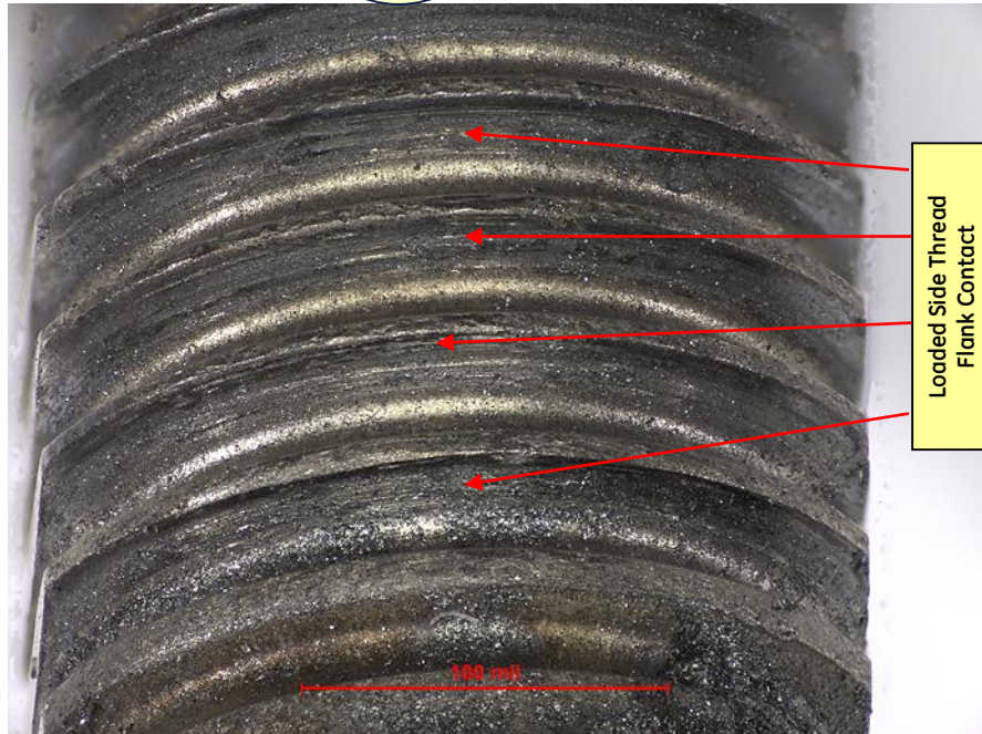
Stg. 1 Vane Trunnion #32 - Loaded Thread Flank Side - Lower Threads
