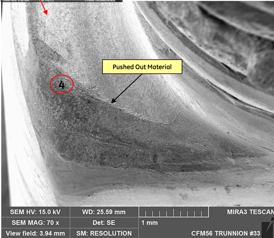
Stg. 1 Vane Trunnion #33 – Damaged Corner - SEI
