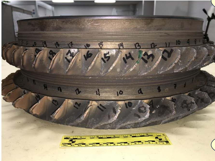
Stg. 1-2 HPC Spool – Radial View
