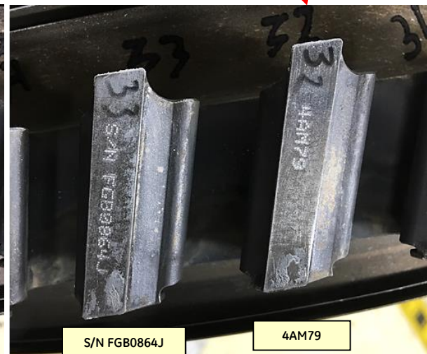
Stg. 1-2 HPC Spool – Blades Removed
