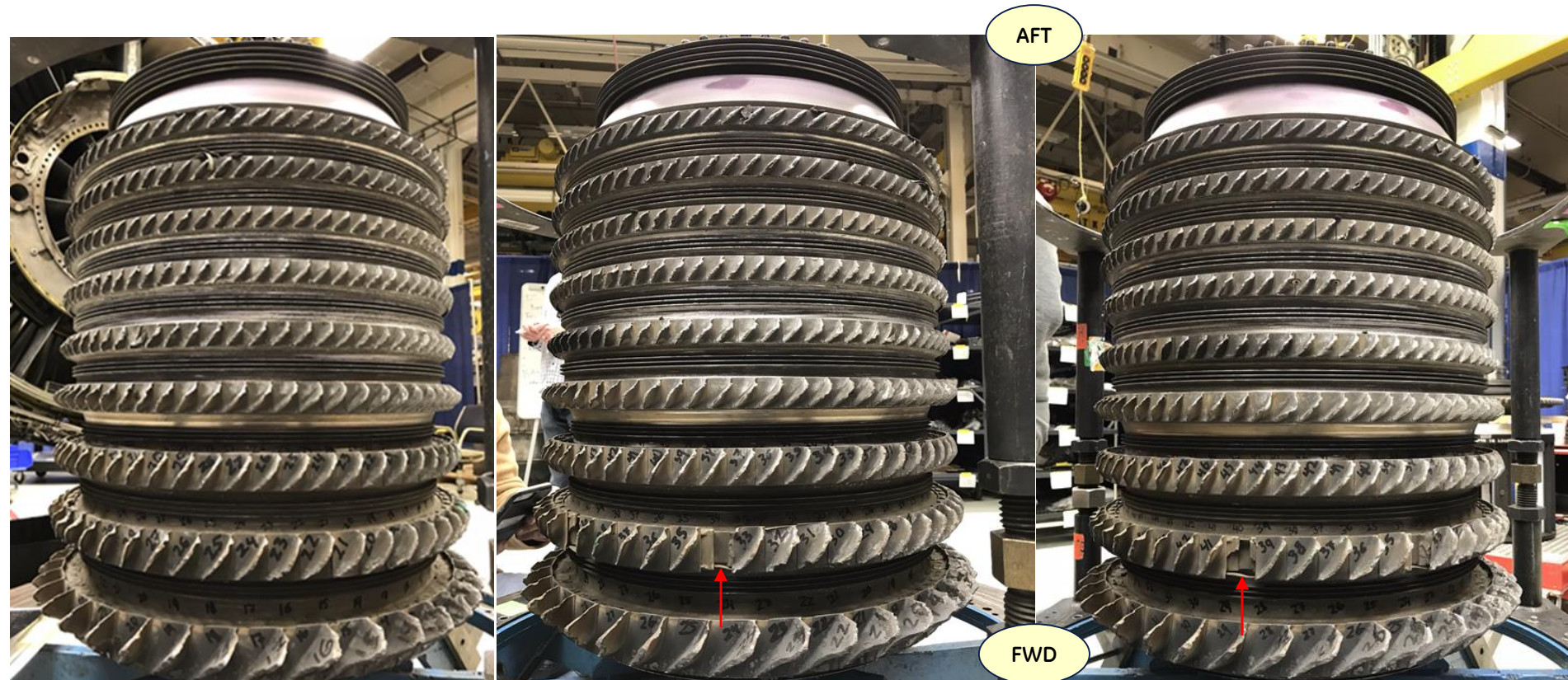
HPC Rotor Condition
