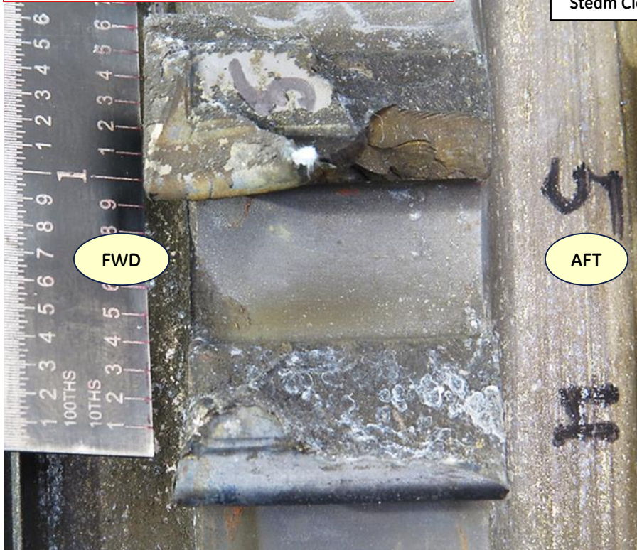
Stg. 2 HPC Disk Posts #4 and #5
