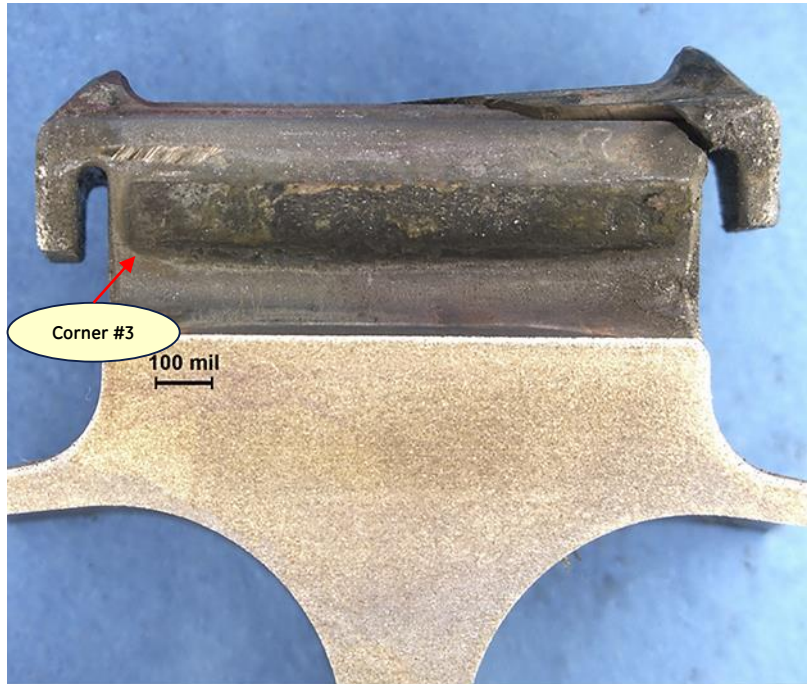
Stg. 1-2 HPC Spool Stg. 2 Disk Post #44 – Corner #3 Crack
