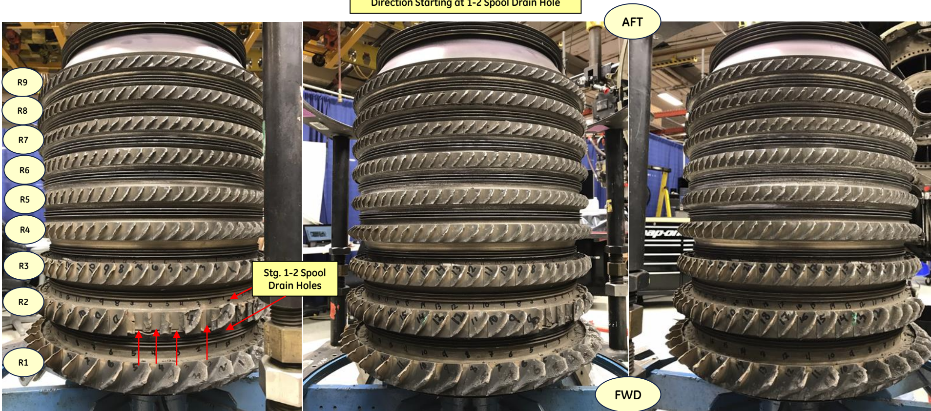
HPC Rotor Condition
