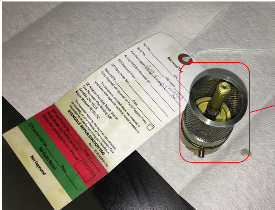
Fwd Sump MCD and Attached Debris
