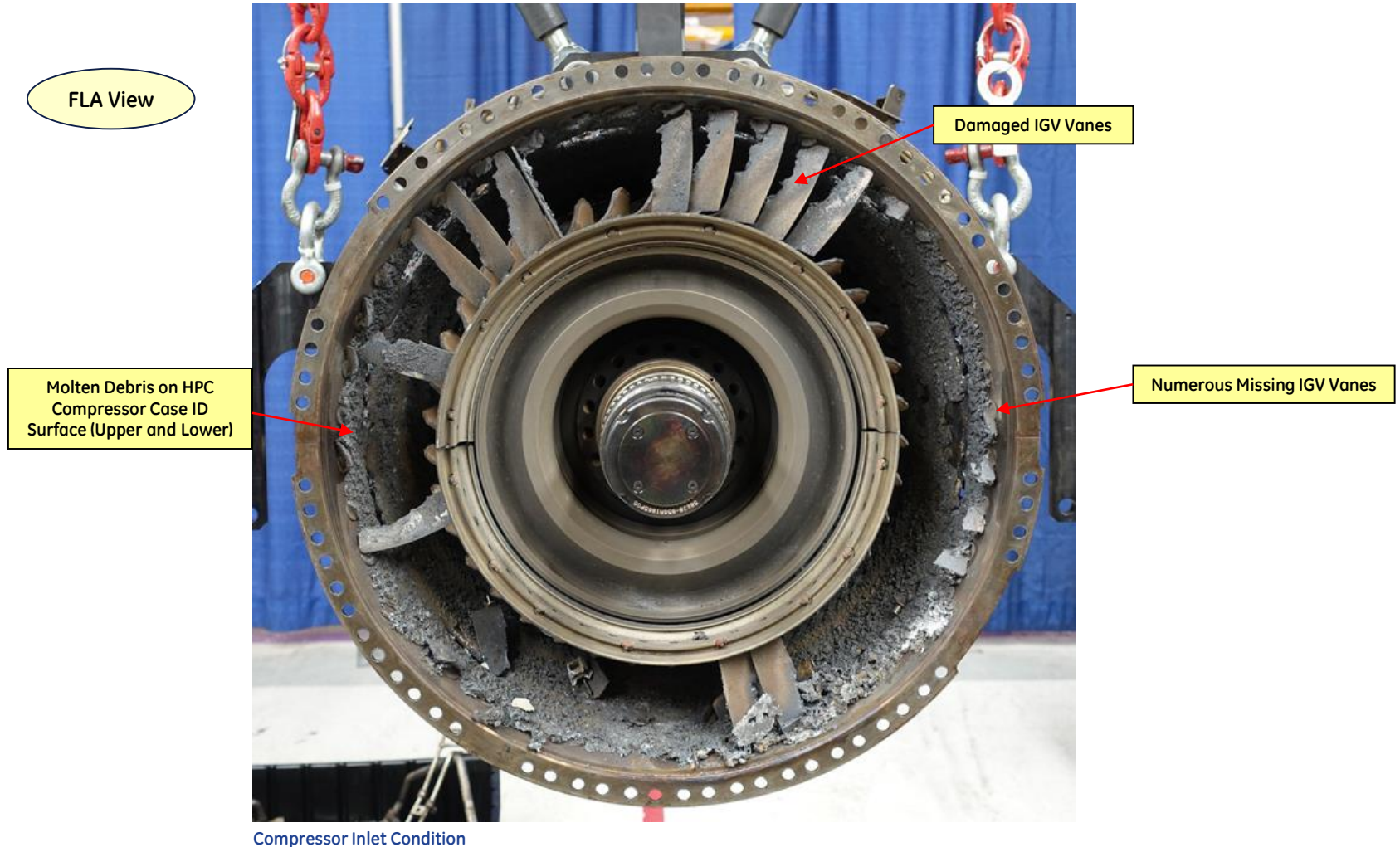
Figure 1. Photograph looking into compressor inlet (FLA). Numerous missing IGV's and abundant molten metal splatter observed on HPC Case ID surface.
