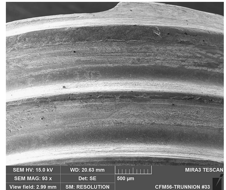
Stg. 1 Vane Trunnion #33 – Upper Thread Contact – SEI
