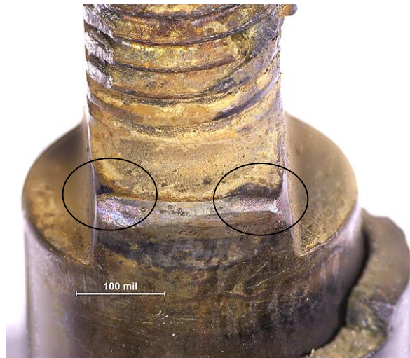
Stg. 1 Vane Trunnion #33 – Corner Damage
