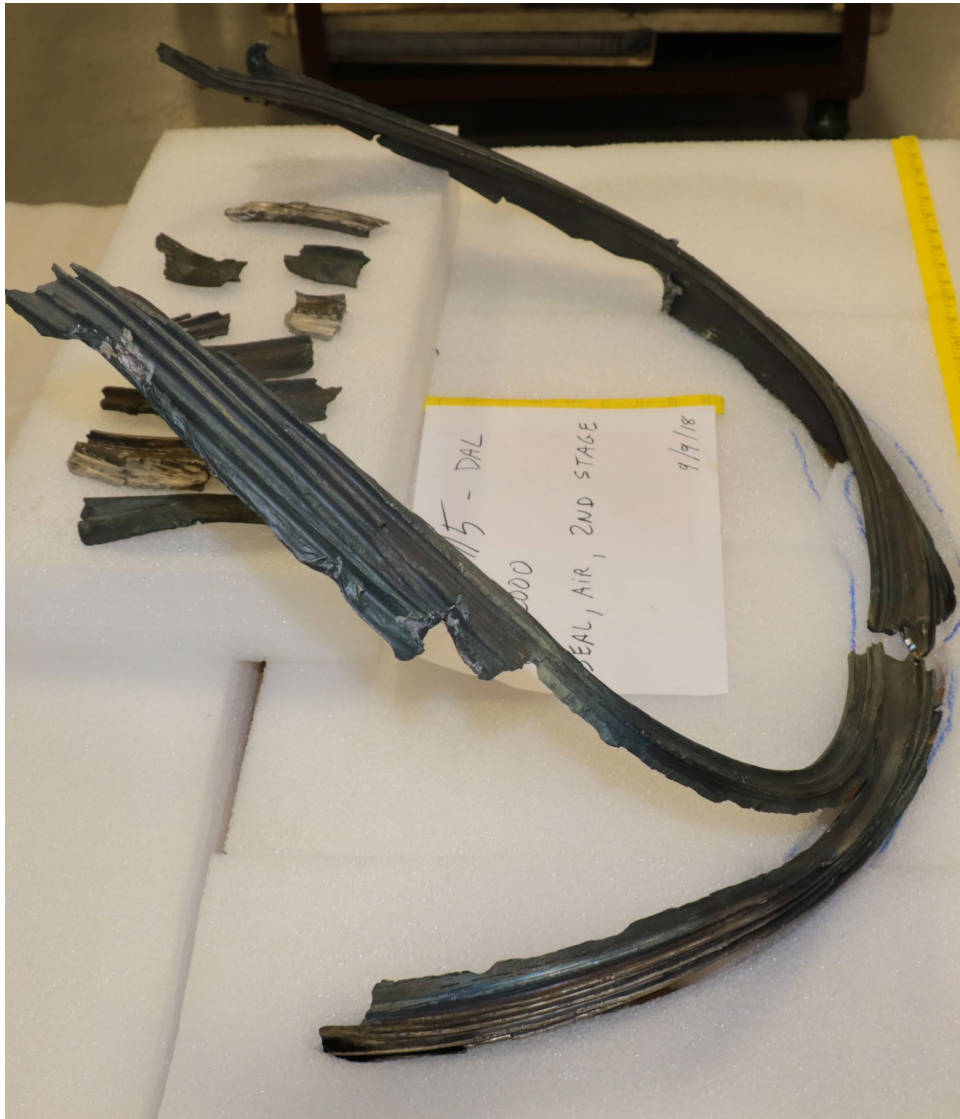
Figure 35. Eleven recovered lenticular seal fragments
