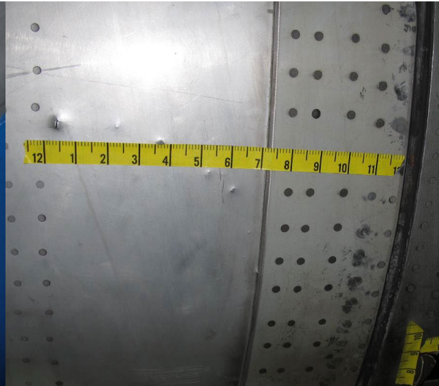
Figure 12. Row of dents in outboard core cowl
