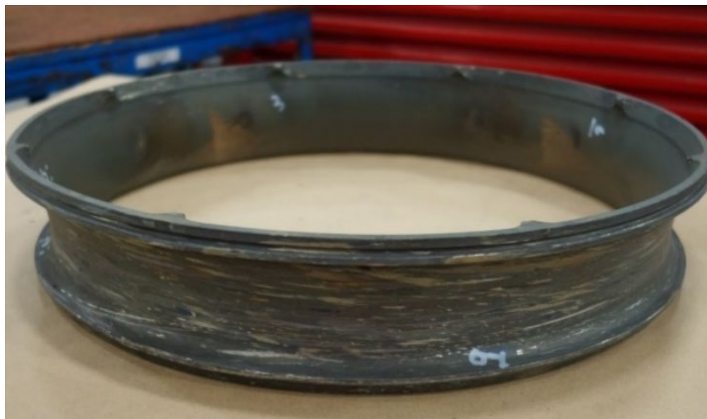
Figure 34. Lenticular seal inner brace piece
