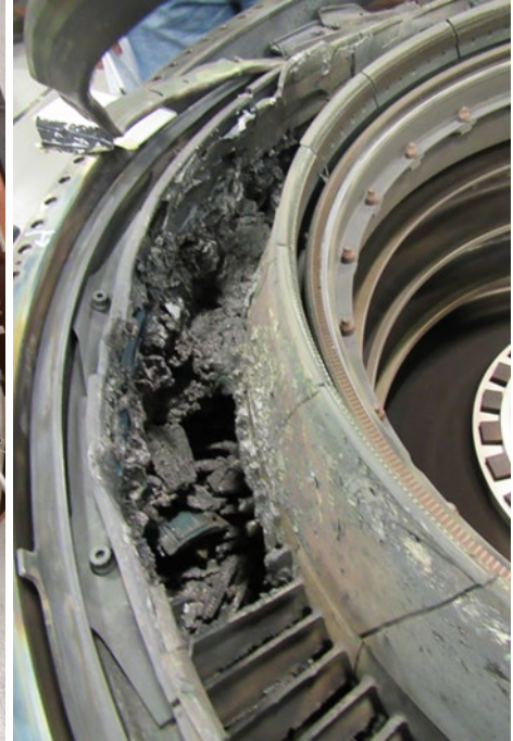
Figure 21. LPT gas path thermal damage
