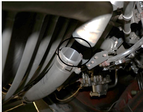
Figure 8. LPT TCC plenum tube manifold with liberated coupling
