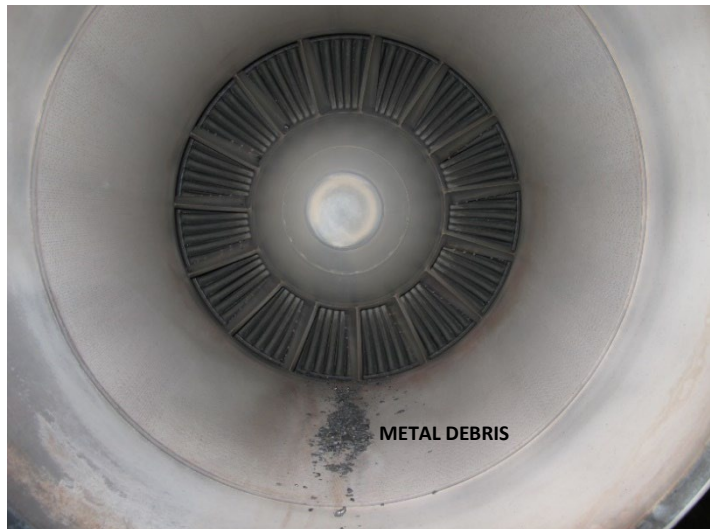
Figure 17. Engine exhaust with intact S7 airfoils
