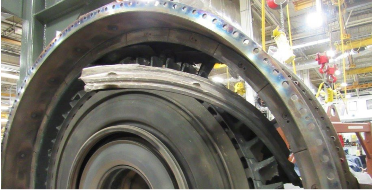
Figure 25. Air seal fragment protruding from forward end of the HPT module
