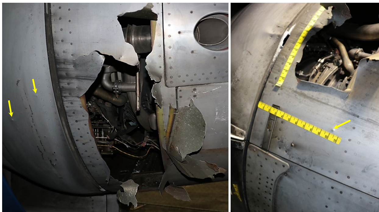
Figure 3. Two photographs of the right nacelle showing hole through inboard side with local dents noted
