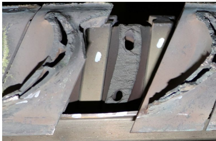
Figure 22. HPT S2 blade below-platform fracture surface
