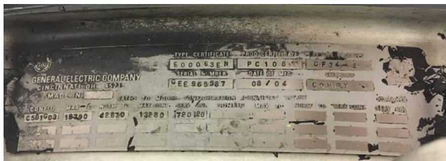
Photo 5- Engine Data Plate
