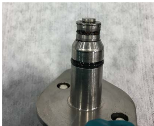
Photo 8- Master Chip Detector Plug
