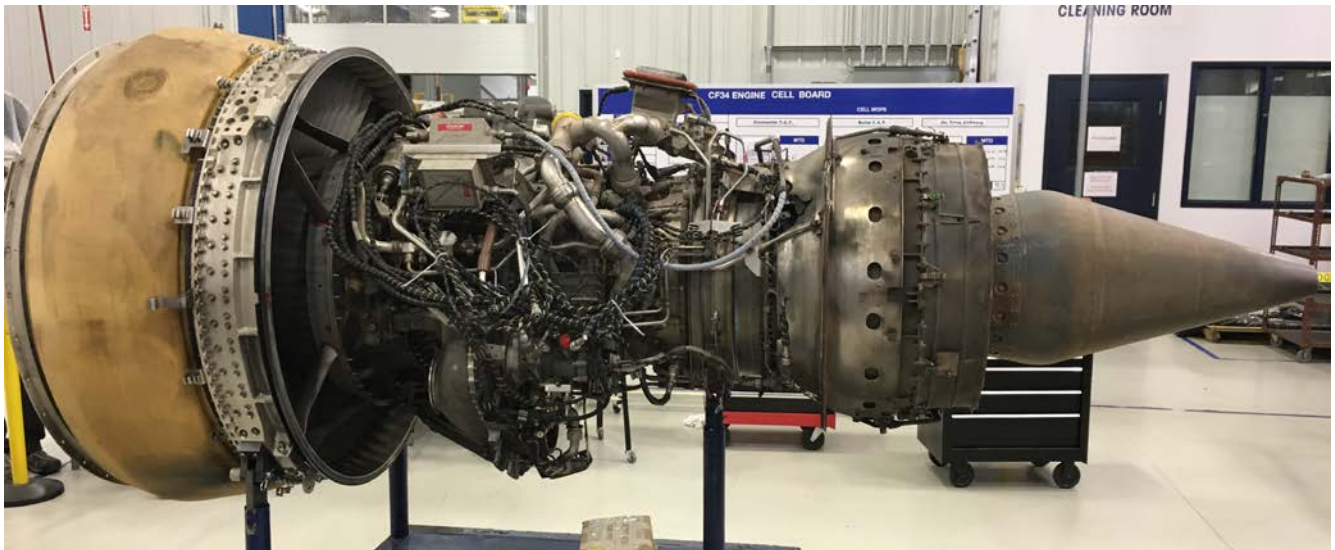
Photo 3- Left Side of Engine
