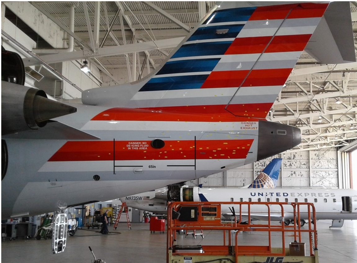
Photo 1- Empennage Damage Map, Impacts Marked with Yellow Tape
