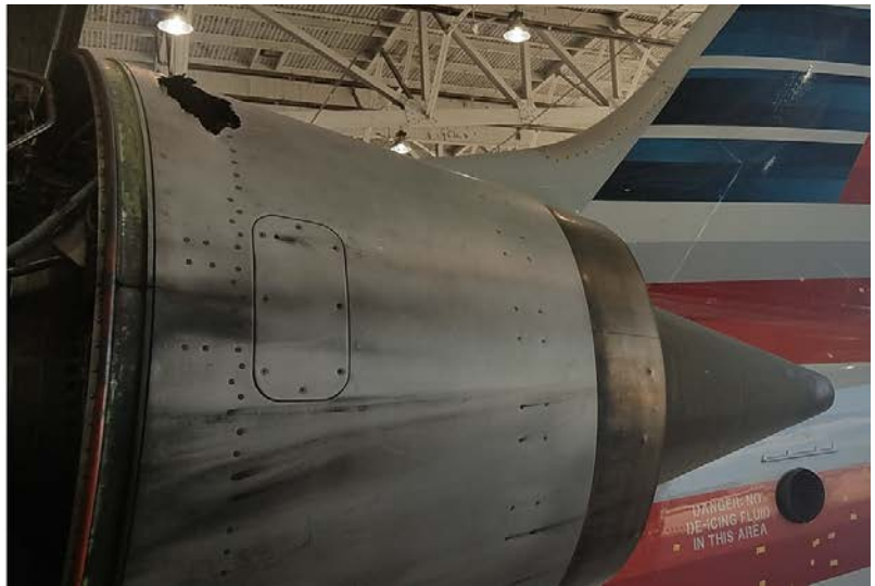
Photo 2- Aft Core Cowl Damage
