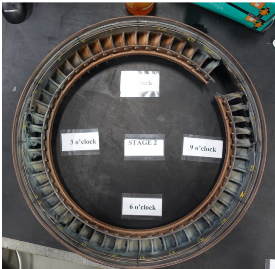
Photo 15- HPT 2 nd Stage Nozzle (L) Pressure Side, (R) Suction Side
