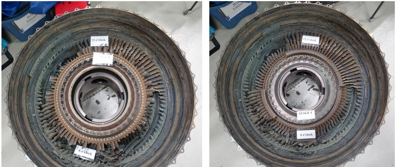
Photo 11- (L) LPT 4th Stage Rotor, (R) LPT 4th Stage Nozzle
