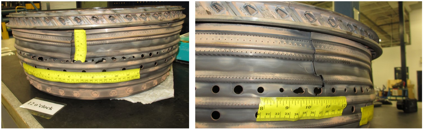
Photo 18- Combustion Outer Liner Cracks (L) 12 o'clock, (R) 2 o'clock
