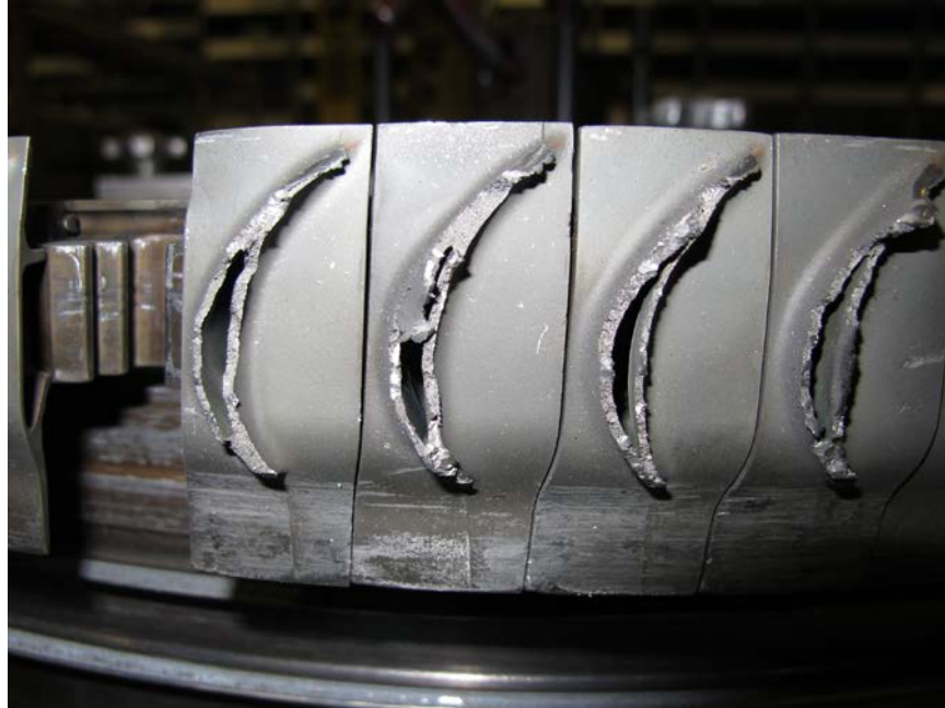
Photo No. 61: Close up view of 6th stage turbine blades showing coarse fracture surface. (P&W)
