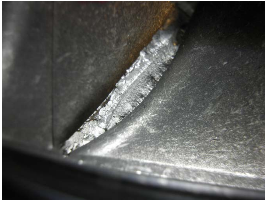
Photo No. 7: Close up view of a 9th stage compressor blade showing elliptical-shaped area on the convex side of the fracture surface. (P&W)
