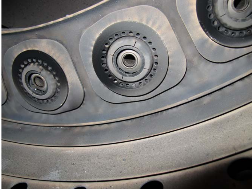
Photo No. 39: Close up of fuel nozzles showing no thermal distress and the sooted splash plates. (P&W)
