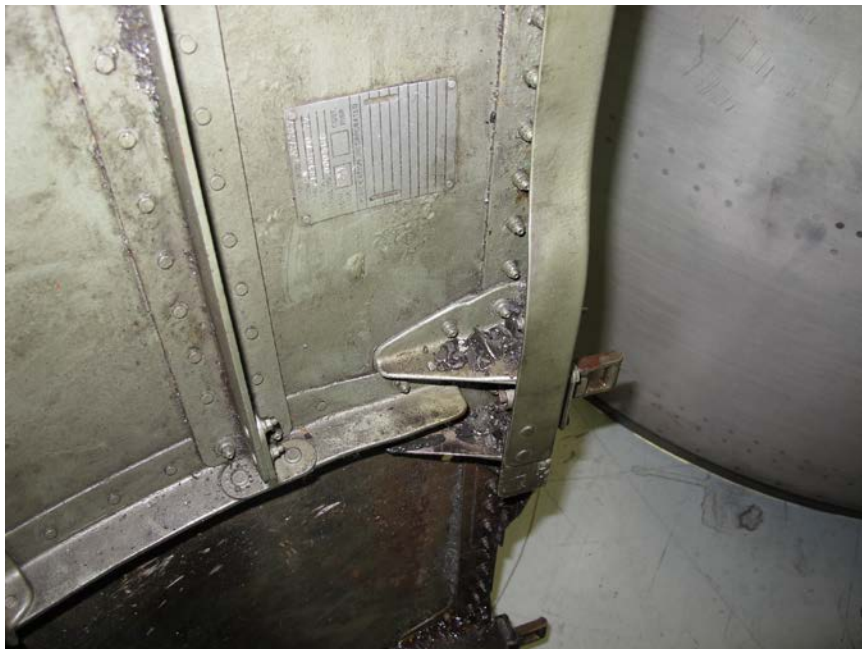
Photo No. 76: Close up view of airfoil debris on the inside of the outboard core cowl. (P&W)
