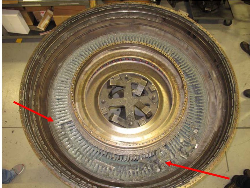
Photo No. 64: View of the 4th stage turbine vanes showing a section was missing between the arrows. (P&W)
