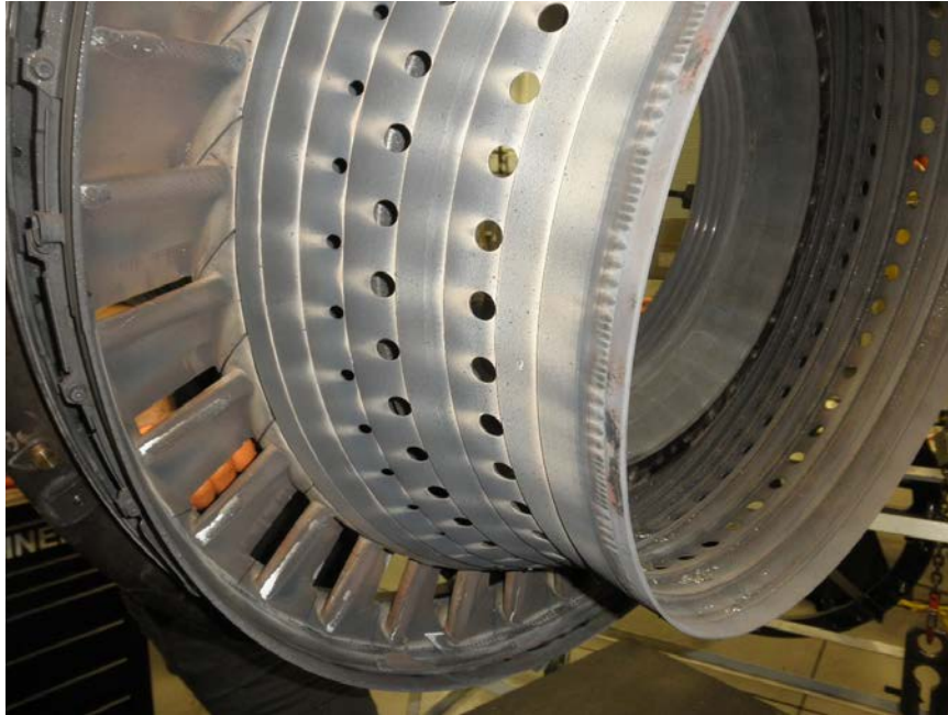
Photo No. 37: View of interior of inner combustion chamber liner showing no thermal distress.
