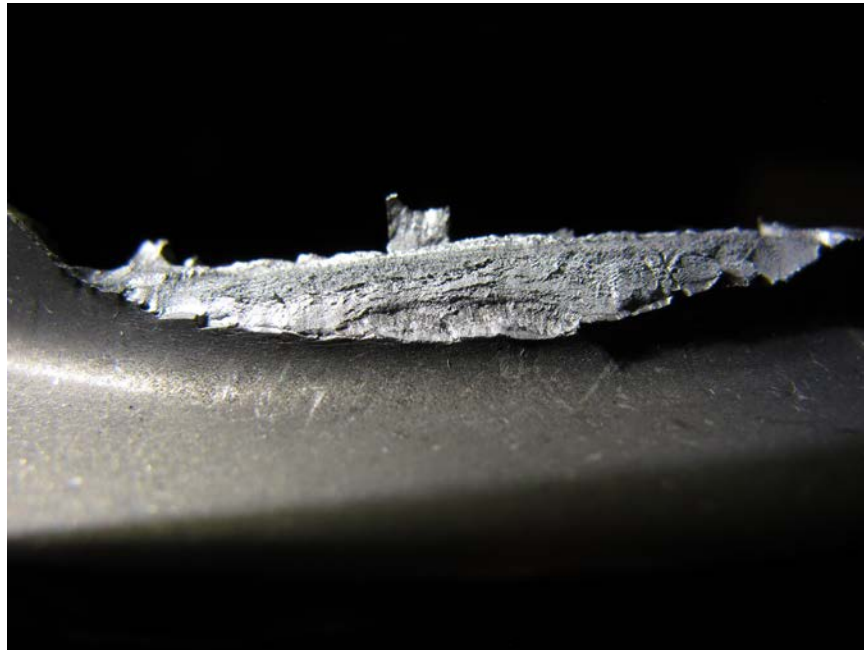
Photo No. 1: Close up view of 5th stage compressor blade fracture surface showing an elliptical shaped area radiating from the convex side of the airfoil. (P&W)
