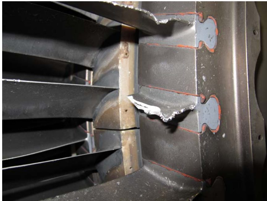
Photo No. 16: Close up view of fractured 4th stage compressor blade. (P&W)
