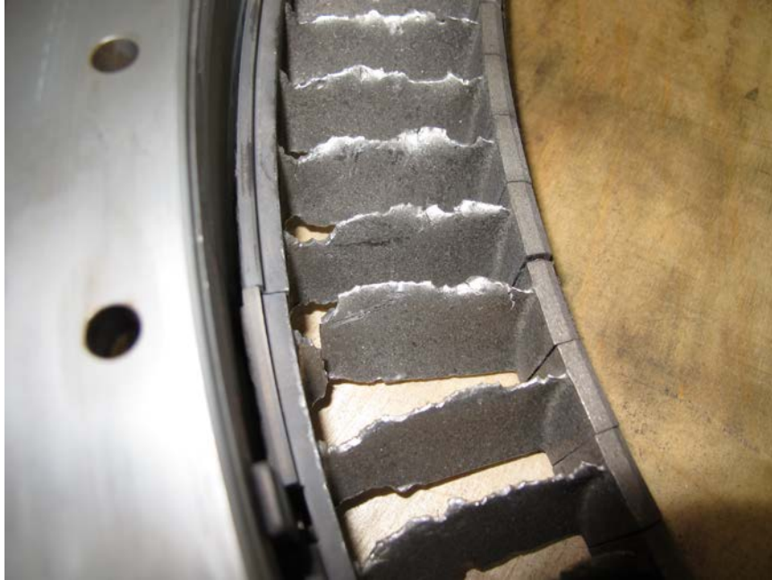
Photo No. 26: Close up view of damaged 11th stage compressor stator. (P&W)
