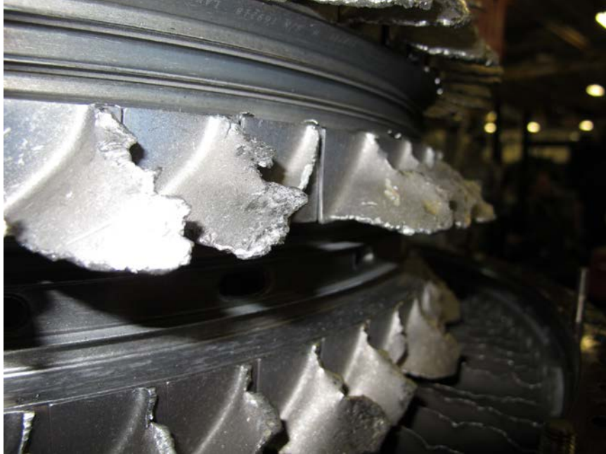
Photo No. 23: Close up view of damaged 10th stage compressor blades. (P&W)
