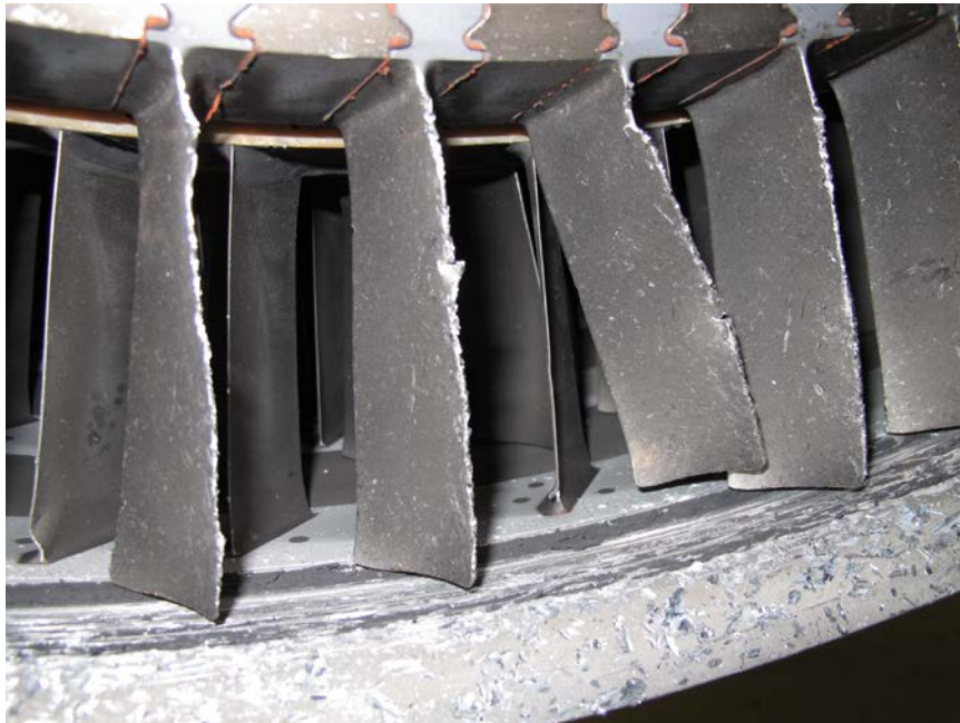
Photo No. 18: Close up view of bent 4th stage compressor blade also showing damage to the trailing edges of the other 4th stage compressor blades. (P&W)
