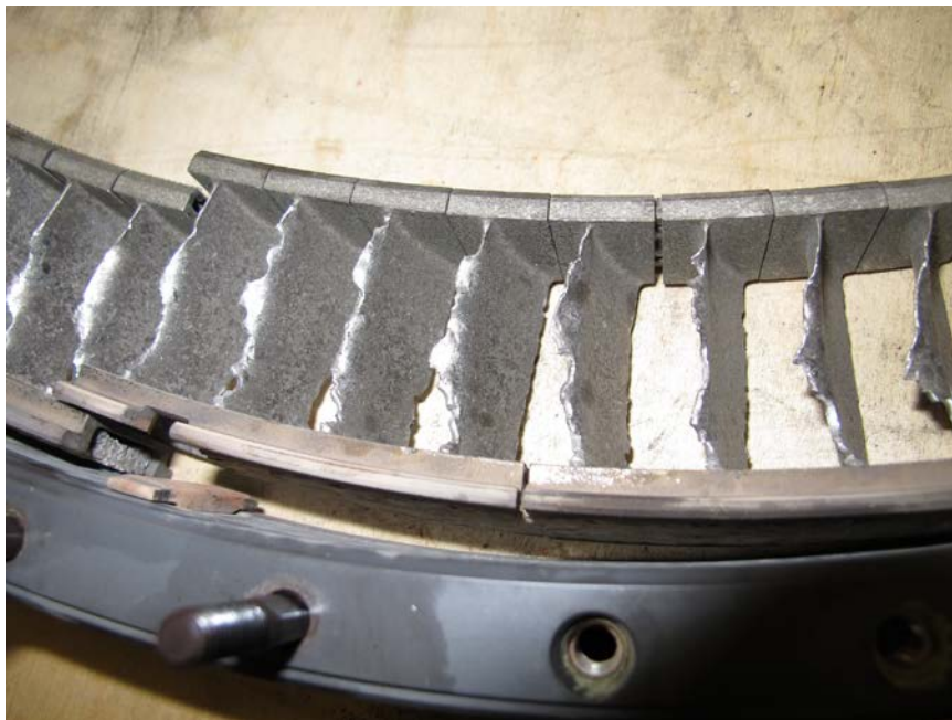
Photo No. 32: Close up view of damaged 14th stage compressor stator. (P&W)
