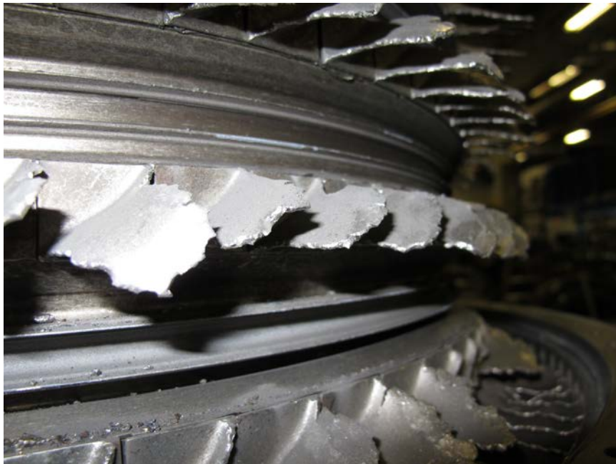
Photo No. 29: Close up view of damaged 13th stage compressor blades. (P&W)
