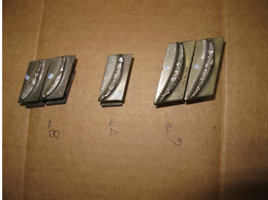
Photo No. 2: 6th, 7th, and 8th stage compressor blades fractured transversely across the airfoil adjacent to the blade root platform. (P&W)
