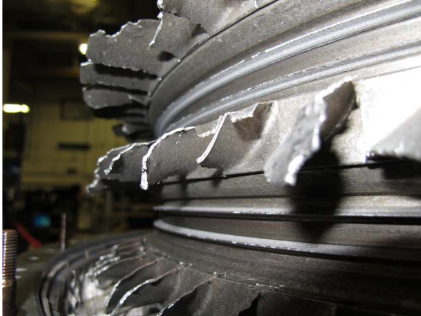
Photo No. 31: Close up view of damaged 14th stage compressor blades. (P&W)
