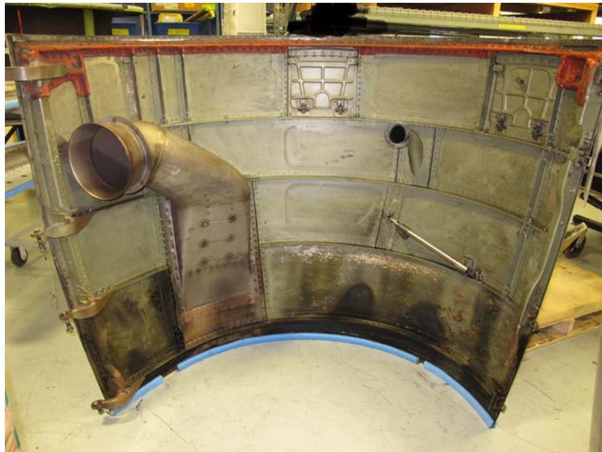
Photo No. 70: View of the outboard core cowl interior showing no penetrations. (P&W)
