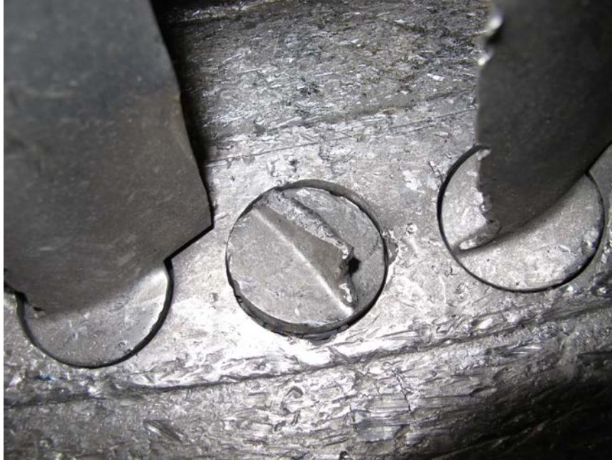
Photo No. 8: View of the fractured outer end of the 5th stage VSV in the upper compressor case half. (P&W)
