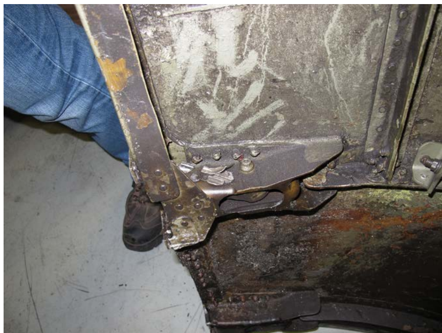
Photo No. 74: Close up view of airfoil debris on the inside of the inboard core cowl. (P&W)
