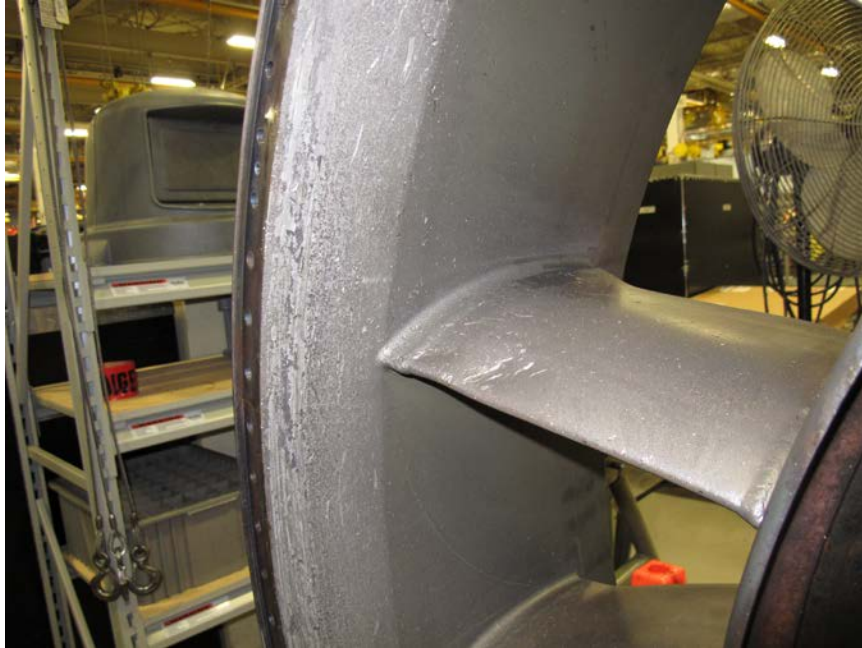
Photo No. 66: View of interior surface of turbine exhaust case and turbine exhaust case strut showing impact nicks, dents, and gouging on both. (P&W)
