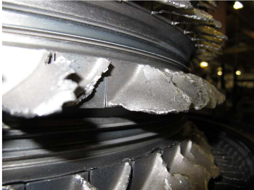
Photo No. 25: Close up view of damaged 11th stage compressor blades. (P&W)
