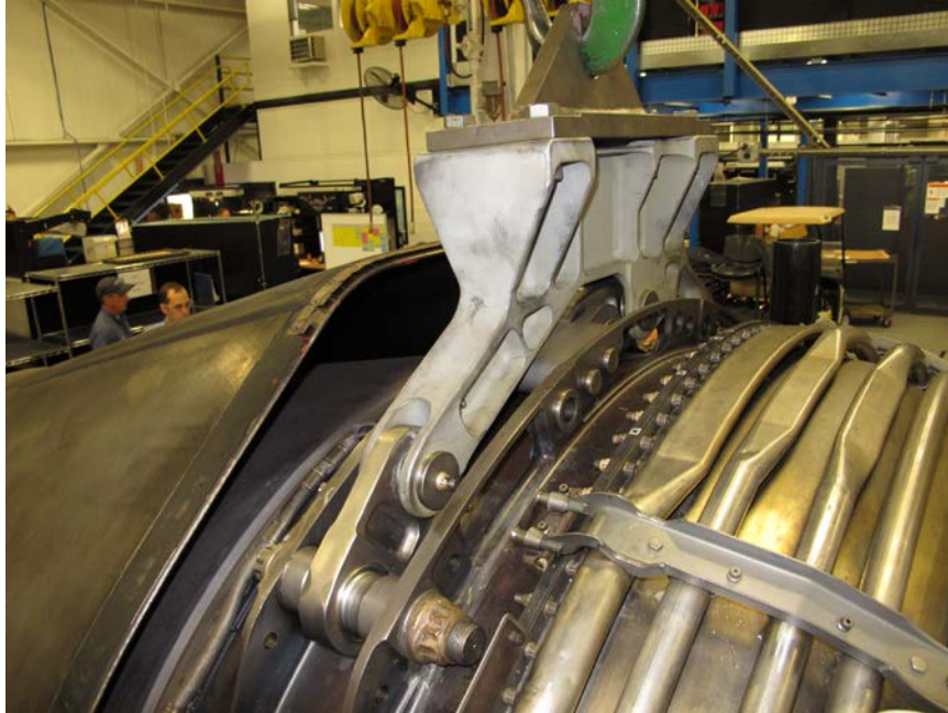
Photo No. 13: View of rear engine mount showing no apparent distress. (P&W)
