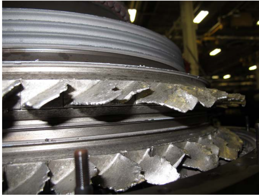
Photo No. 33: Close up view of damaged 15th stage compressor blades. (P&W)
