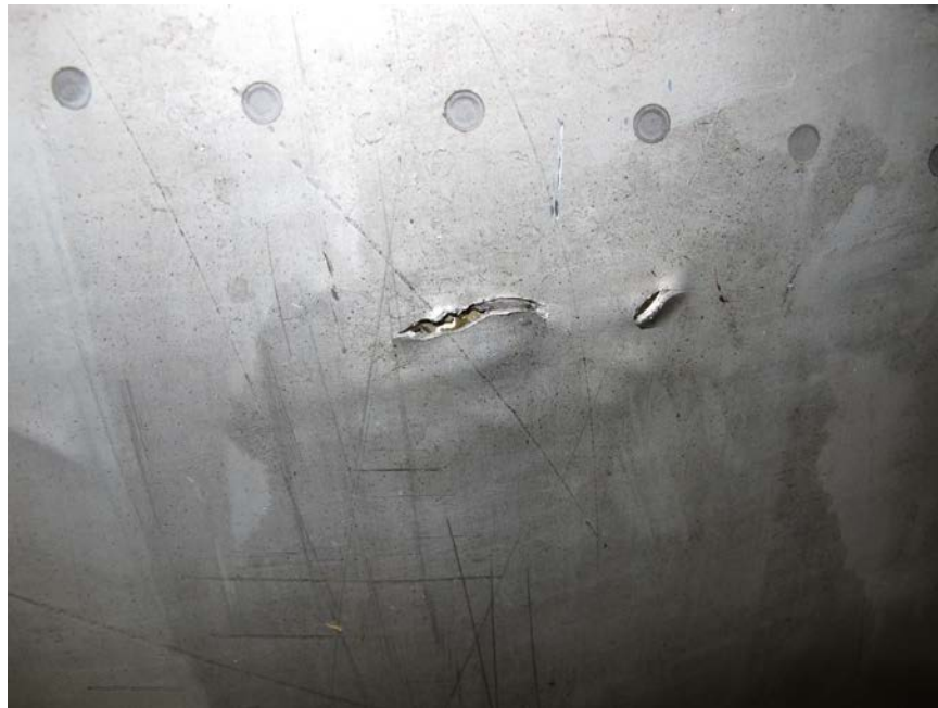
Photo No. 73: Close up view of the two splits in the skin of the inboard core cowl. (P&W)
