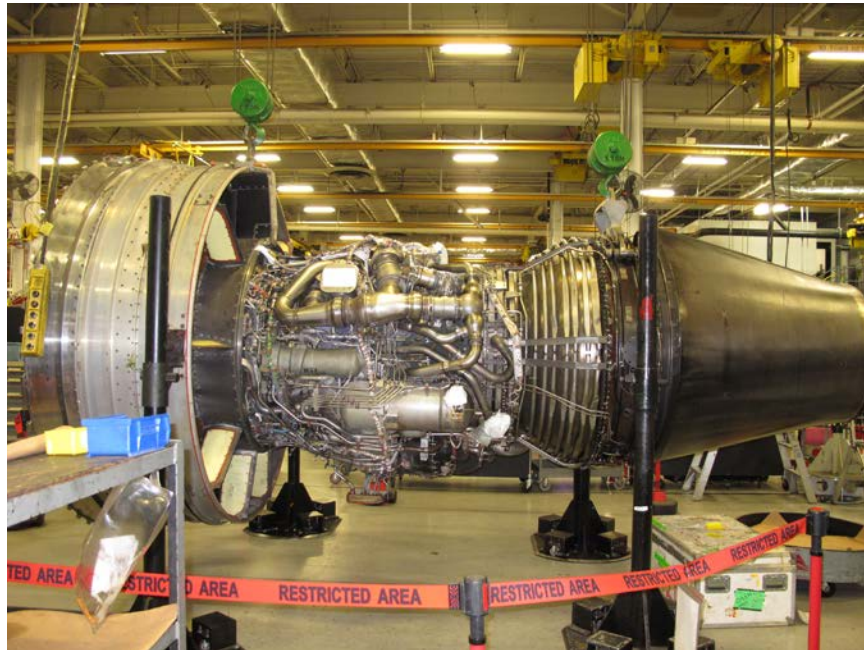
Photo No. 10: View of left side of engine showing no indications of an uncontainment, case rupture or an undercowl fire. (P&W)
