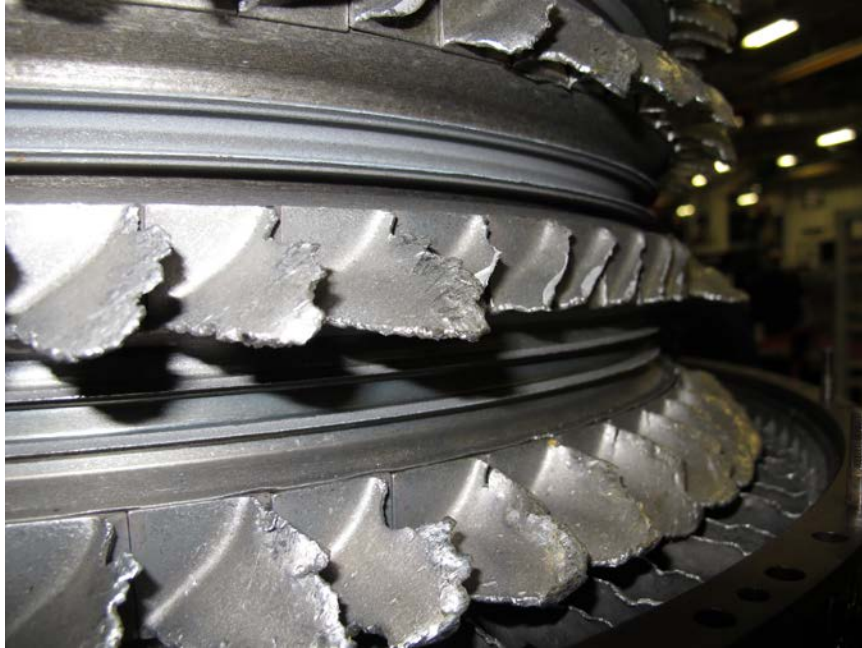
Photo No. 27: Close up view of damaged 12th stage compressor blades. (P&W)
