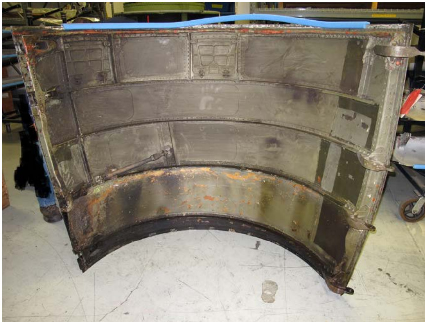
Photo No. 72: View of the inboard core cowl interior showing no penetrations. (P&W)
