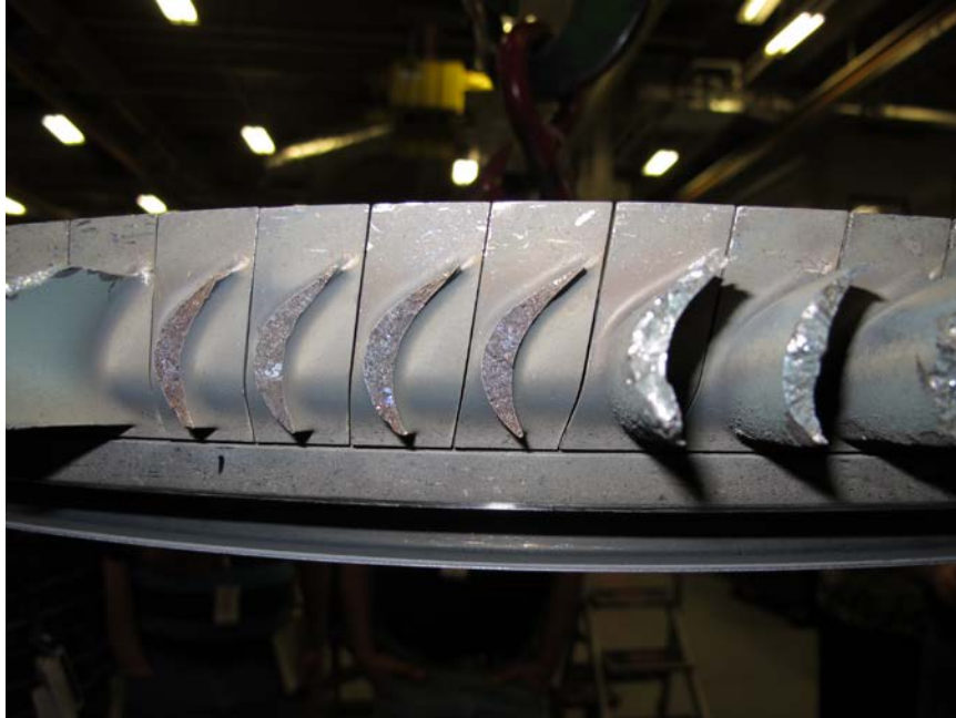
Photo No. 58: Close up view of 3rd stage turbine blades showing coarse fracture surface. (P&W)
