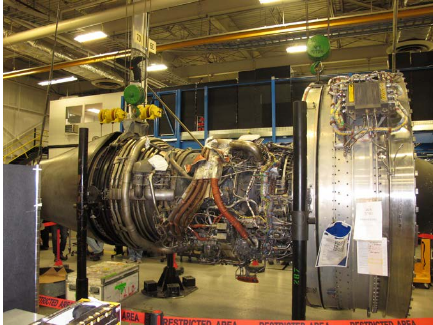
Photo No. 11: View of right side of engine showing no indications of an uncontainment, case rupture, or an undercowl fire. (P&W)
