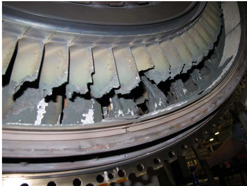
Photo No. 44: View of 2nd stage turbine blades showing they were in place and had coarse fractured ends. (P&W)
