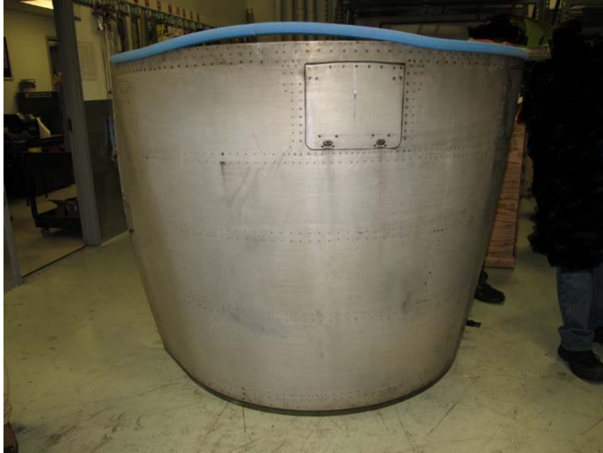
Photo No. 71: View of the inboard core cowl exterior showing no penetrations. (P&W)
