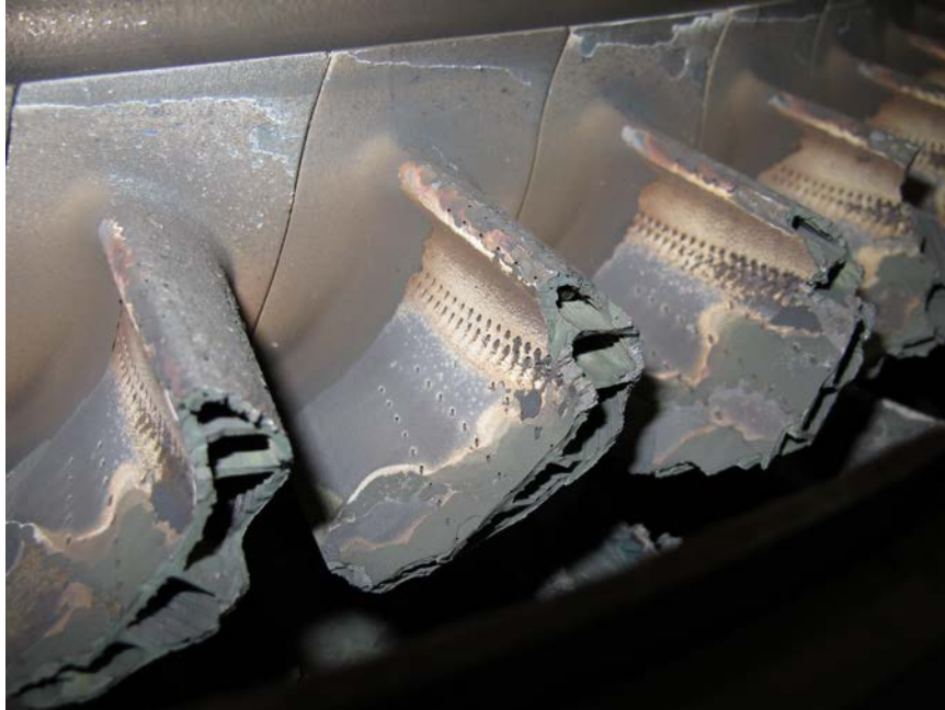
Photo No. 42: Close up view of 1st stage turbine blades showing coarse fracture surface on ends of the blades. (P&W)
