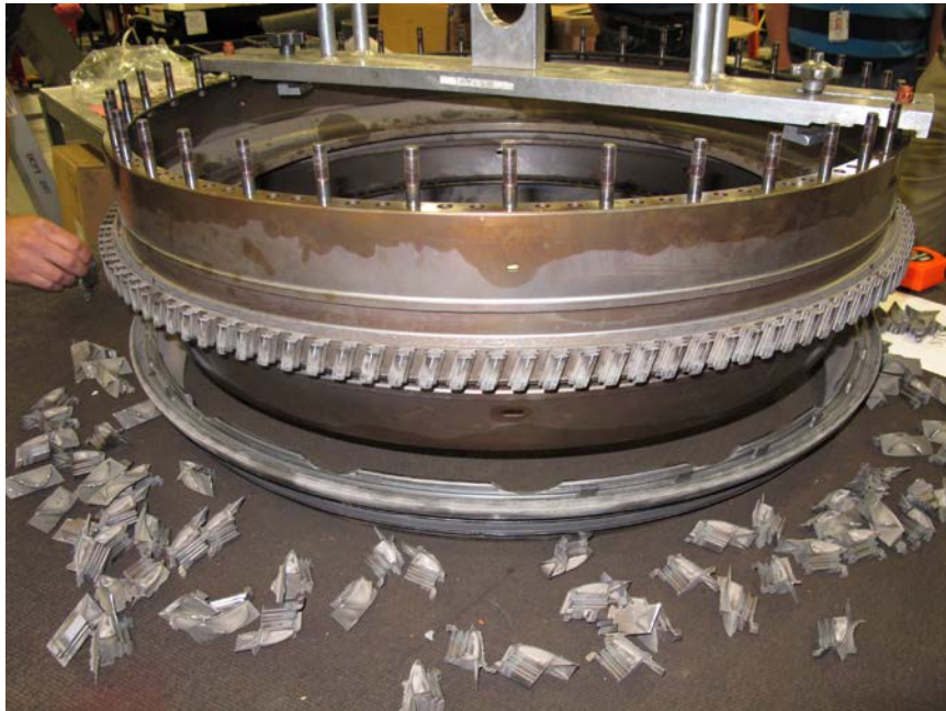
Photo No. 55: View of the 4th stage turbine disk showing that it was intact. (P&W)
