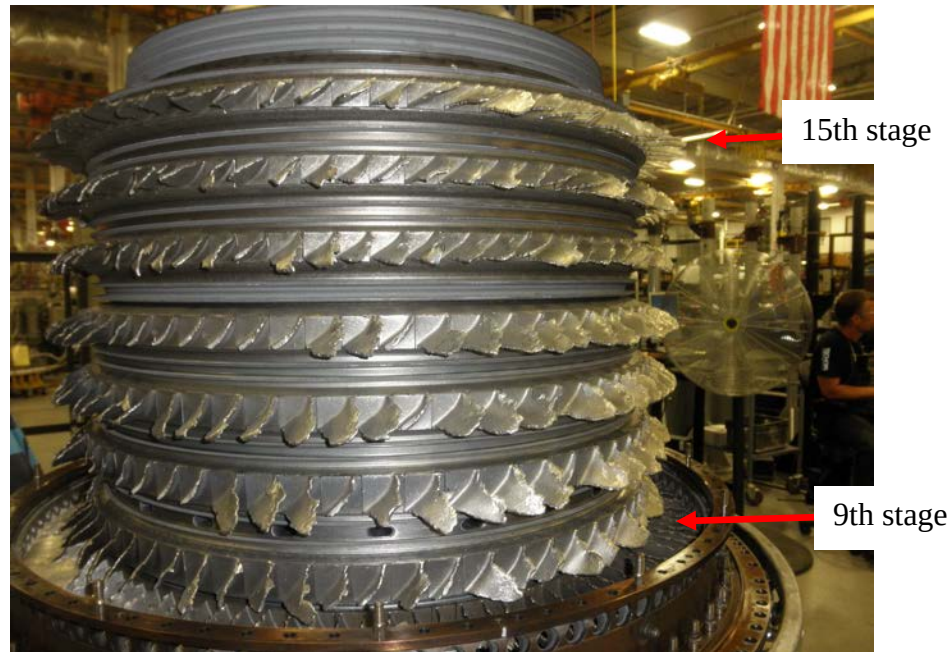
Photo No. 6: View of HPC stages 9 through 15 showing damaged, fractured, and bent airfoils. (P&W)
