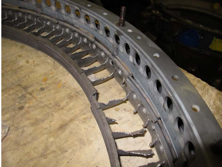
Photo No. 28: Close up view of damaged 12th stage compressor stator. (P&W)
