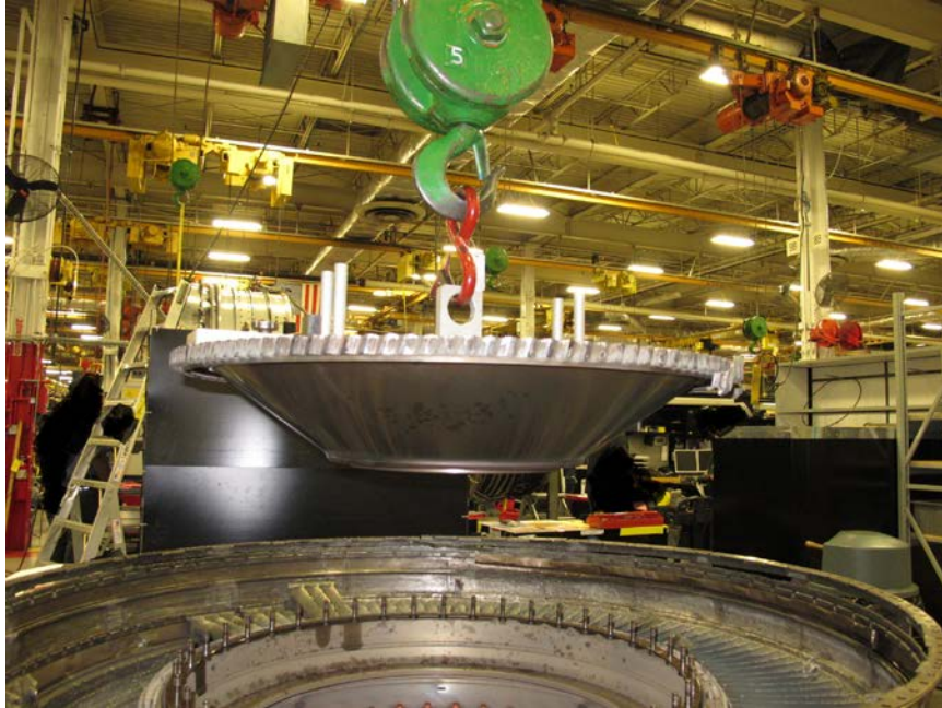
Photo No. 56: View of the 5th stage turbine disk showing that it was intact. (P&W)
