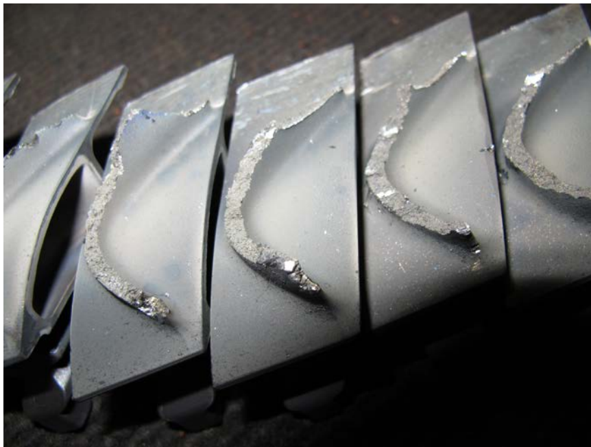
Photo No. 59: Close up view of 4th stage turbine blades showing coarse fracture surface. (P&W)
