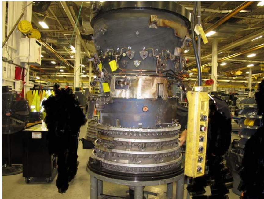
Photo No. 19: View of HPC showing all of the VSV rings were in place and no exterior damage to the front and rear compressor cases. (P&W)
