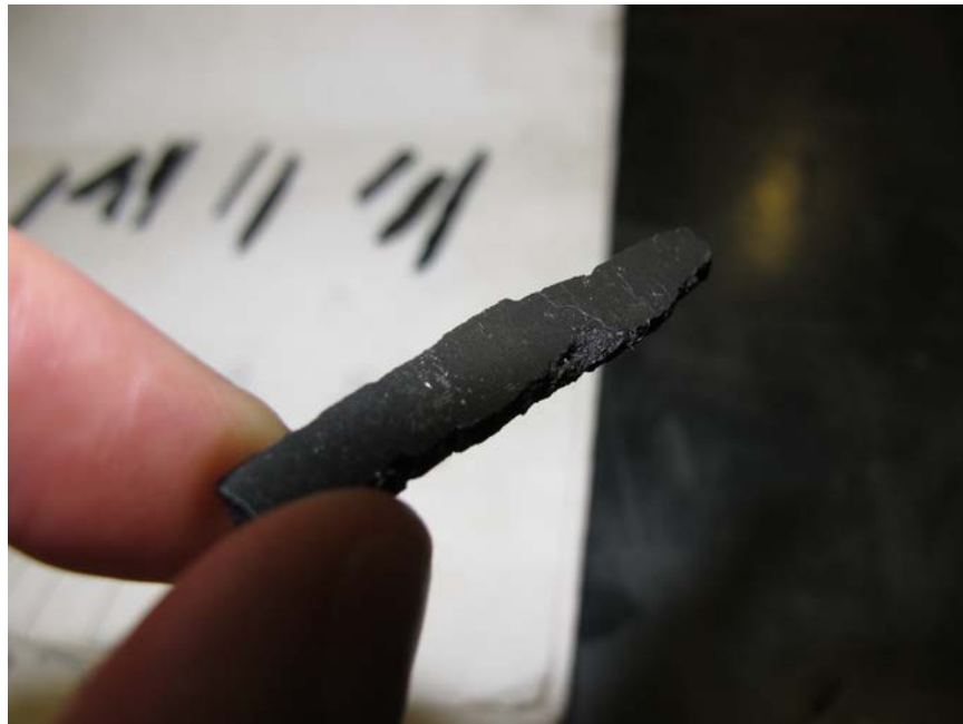
Photo No. 51: Close up view of metal shard found in turbine debris that had machining marks similar to machining marks on outside of LPT case. (P&W)
