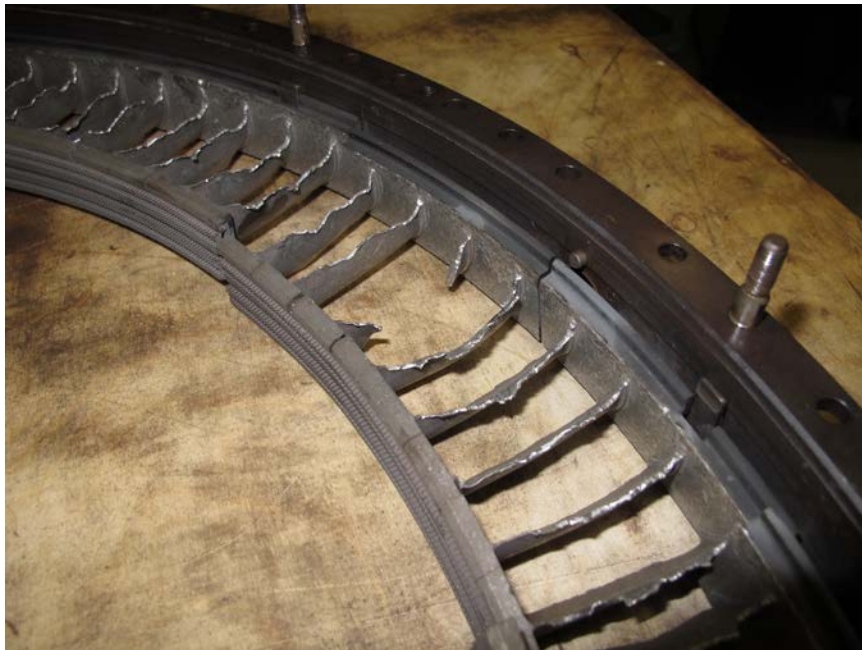
Photo No. 24: Close up view of the damaged 10th stage compressor stator. (P&W)
