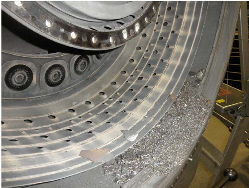
Photo No. 36: View of interior of outer combustion chamber liner showing no thermal distress.
