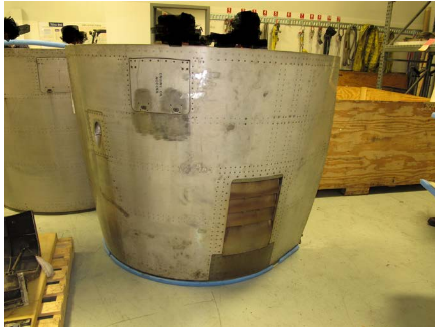
Photo No. 69: View of the outboard core cowl exterior showing no penetrations. (P&W)
