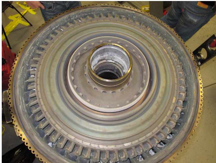
Photo No. 41: View of front of HPT stage 1 disk and front side plate showing disk intact and front side plate in place with no oil staining. (P&W)
