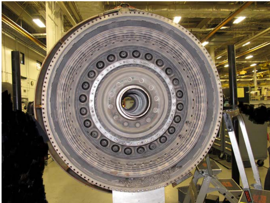
Photo No. 38: View of combustor liner showing all of the fuel nozzles were in place. (P&W)
