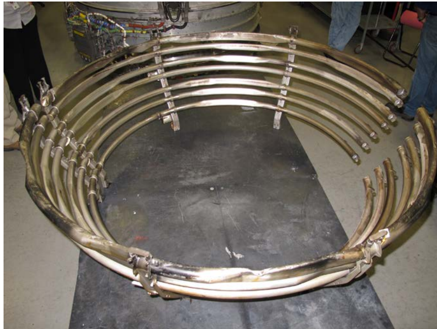
Photo No. 52: View of the upper and lower turbine case cooling air manifolds showing no damage to manifolds Nos. 1 through 6, but damage to manifold No. 7. (P&W)
