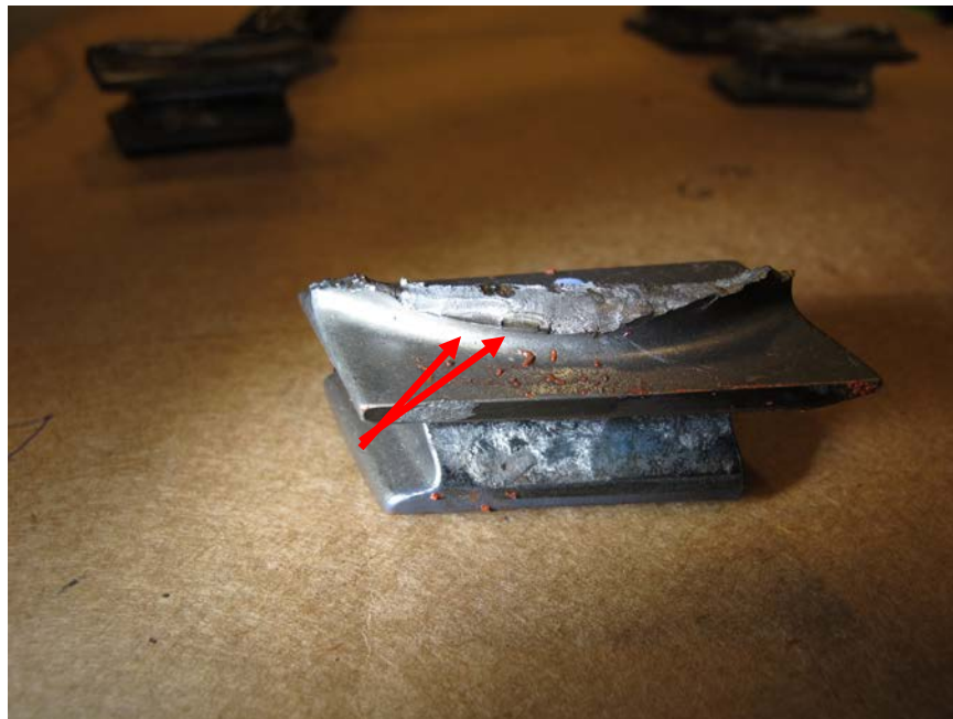
Photo No. 3: Close up view of a 6th stage compressor blade showing two elliptical-shaped areas on the convex side of the fracture surface. (P&W)
