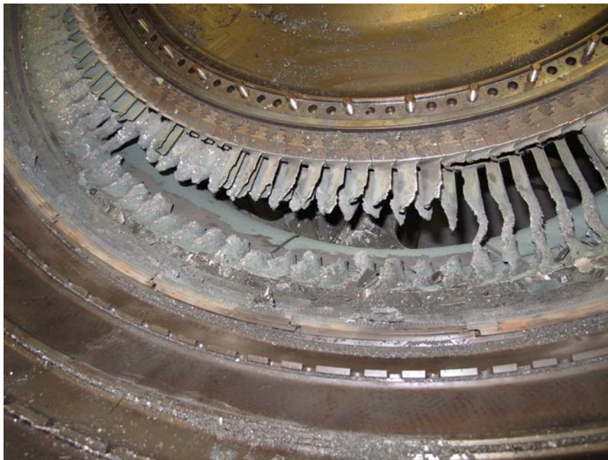
Photo No. 63: View of 3rd stage turbine vanes trailing edges showing section burned out completely and other vanes partially burned away. (P&W)
