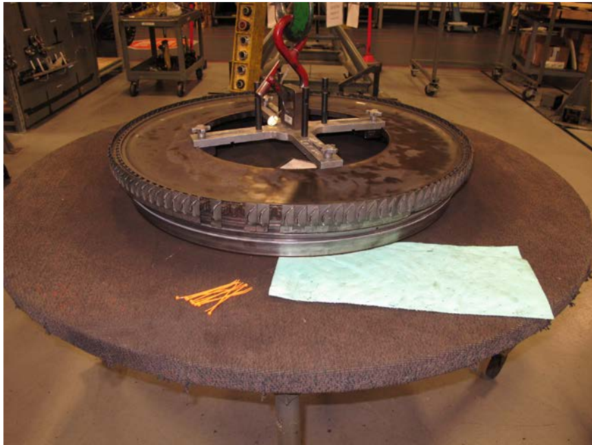
Photo No. 57: View of 6th stage turbine disk showing that it was intact. (P&W)
