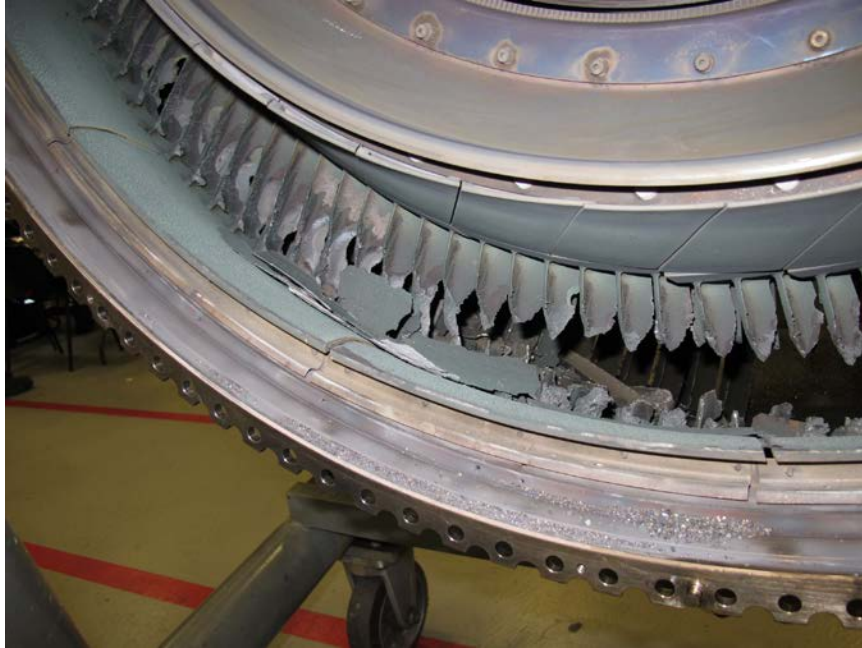
Photo No. 53: View of outer transition duct segments showing green-tinted metal spray material on segments as well as metal spray material on the bottom of the engine. (P&W)
