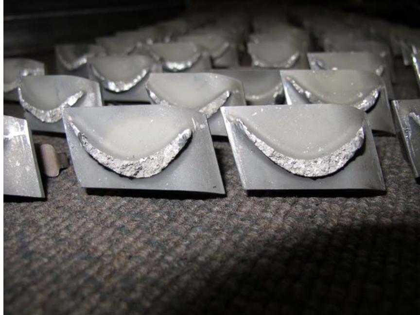
Photo No. 60: Close up view of 5th stage turbine blades showing coarse fracture surface. (P&W)
