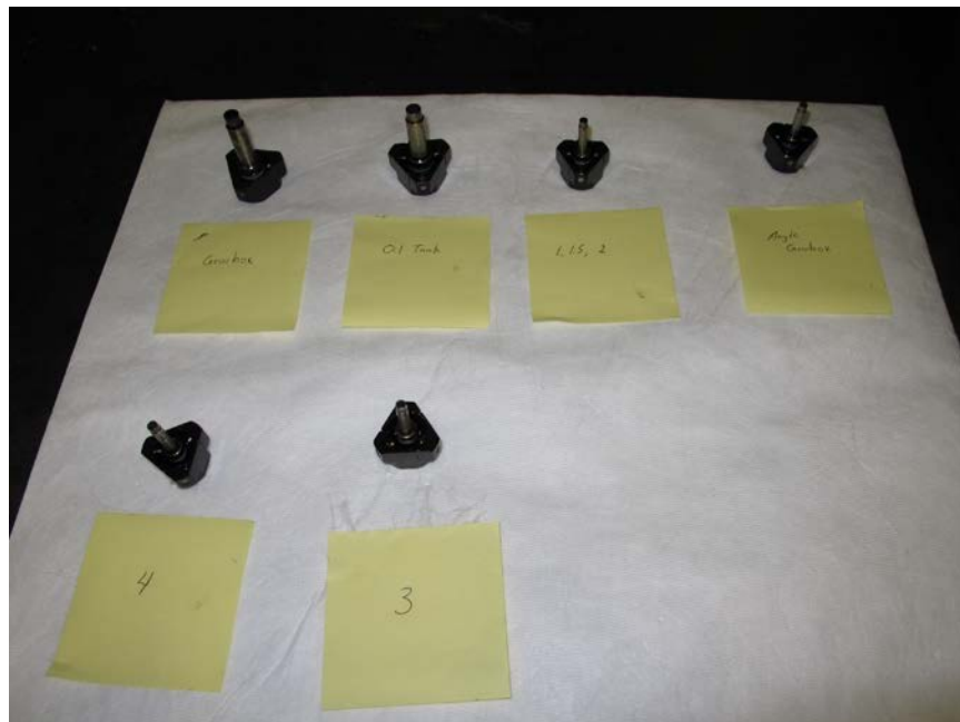
Photo No. 68: Magnetic chip detectors with minute bits of debris. (P&W)
