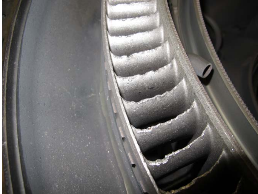
Photo No. 34: Close up view of damaged 15th stage compressor stator vanes. (P&W)
