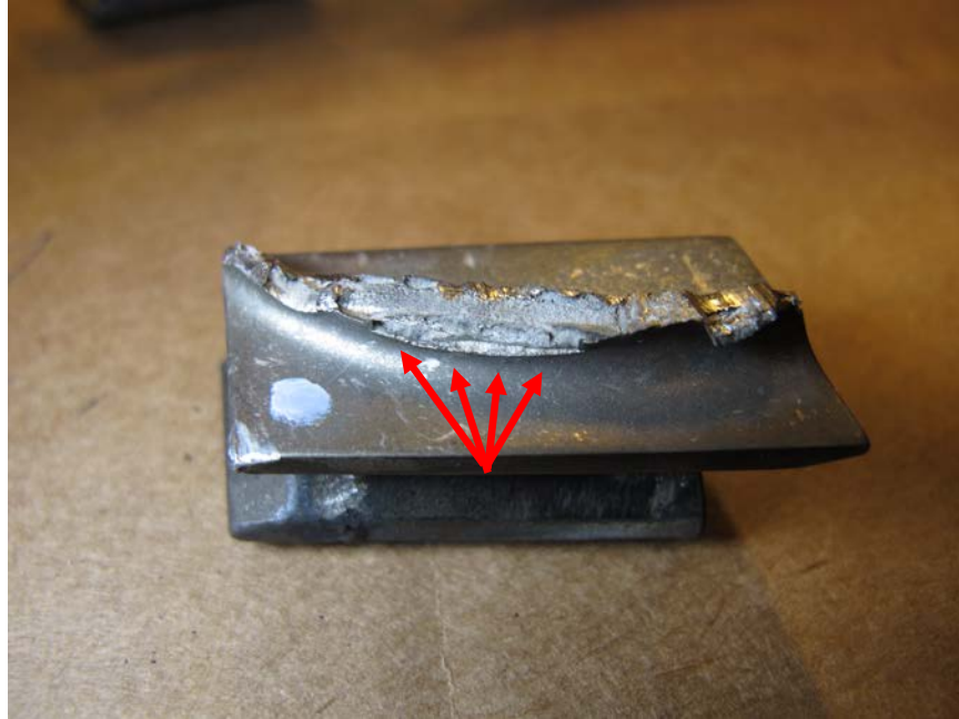
Photo No. 4: Close up view of a 7th stage compressor blade showing elliptical-shaped area on the convex side of the fracture surface. (P&W)
