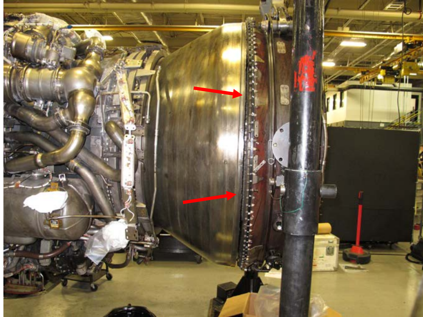
Photo No. 47: Left side of engine showing circumferential split in LPT case. (P&W)
