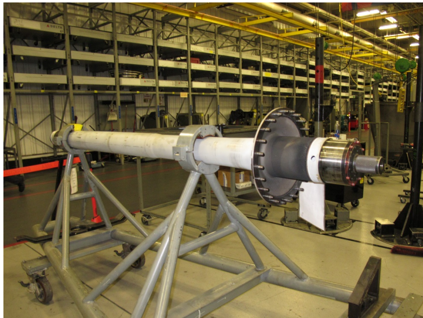
Photo No. 45: View of LPC drive shaft after it was removed from the engine and separated from the LPT showing it was intact and did not have any rub marks. (P&W)
