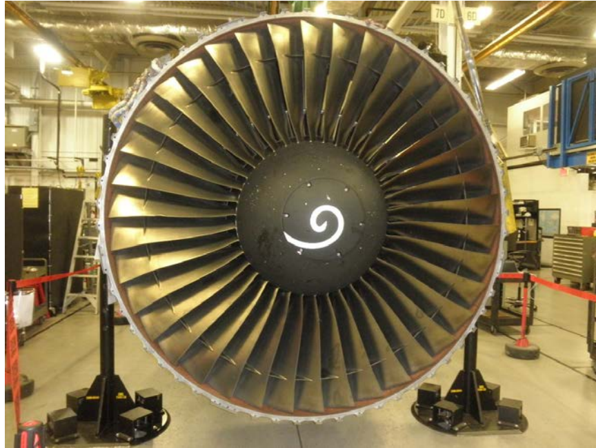
Photo No. 14: View of front of the engine showing the spinner, spinner cap, and all of the fan blades were in place and that there was no damage to any of those components. (P&W)
