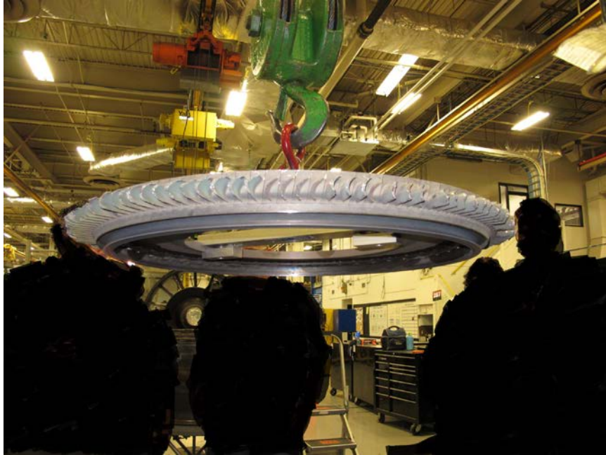
Photo No. 54: View of 3rd stage turbine disk showing that it was intact. (P&W)
