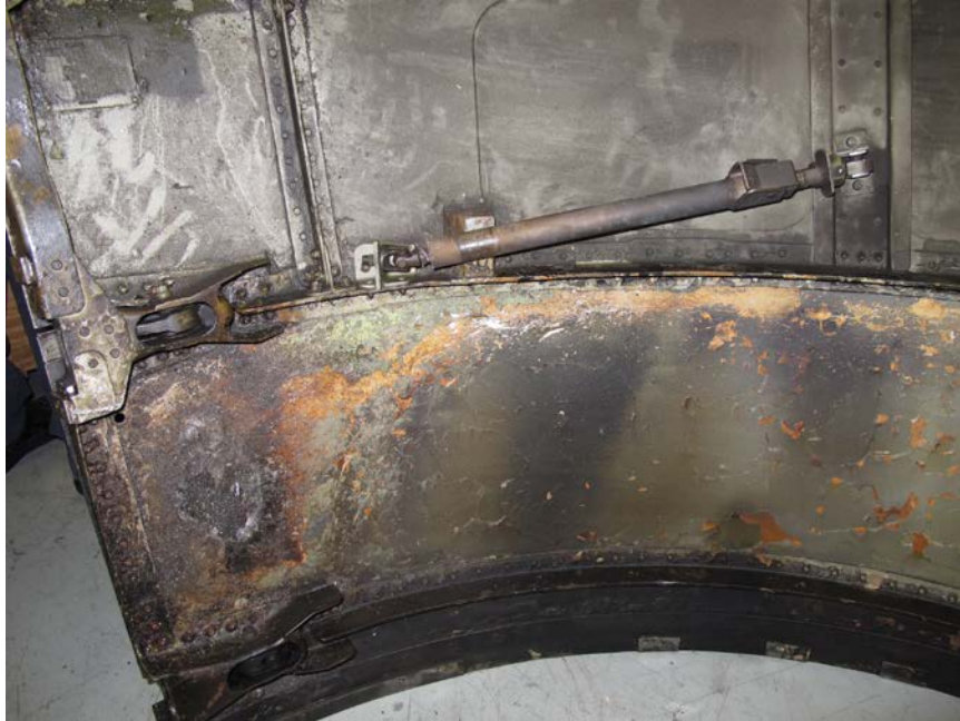
Photo No. 75: View of damage to inside of inboard core cowl. (P&W)
