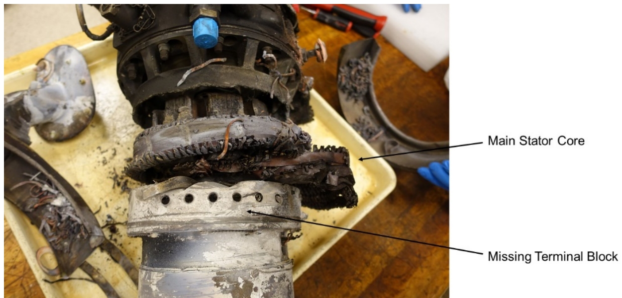
Photo 8- Generator Case Damage
