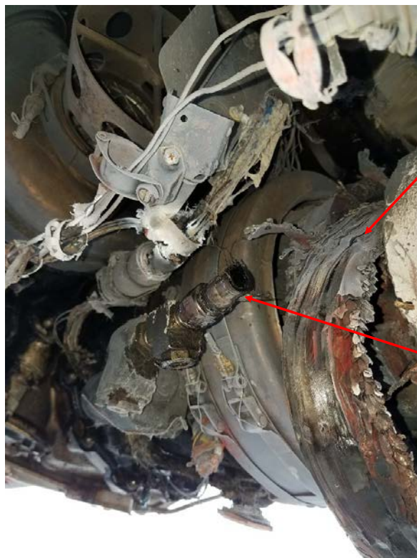
Photo 2- Oil Cooler Return Line and Generator Case Damage
