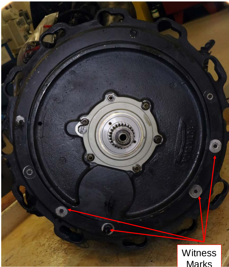
Photo 5- CSD Mounting Pad Forward Face, Witness Marks
