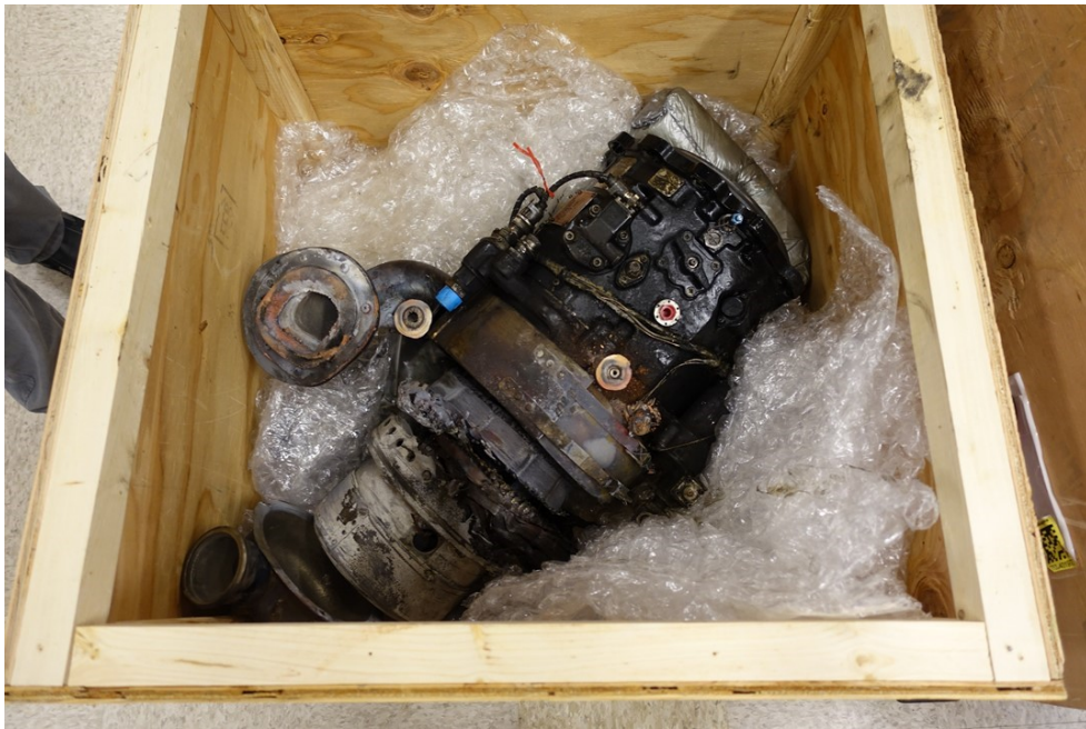
Photo 3- CSD and Generator, As Received
