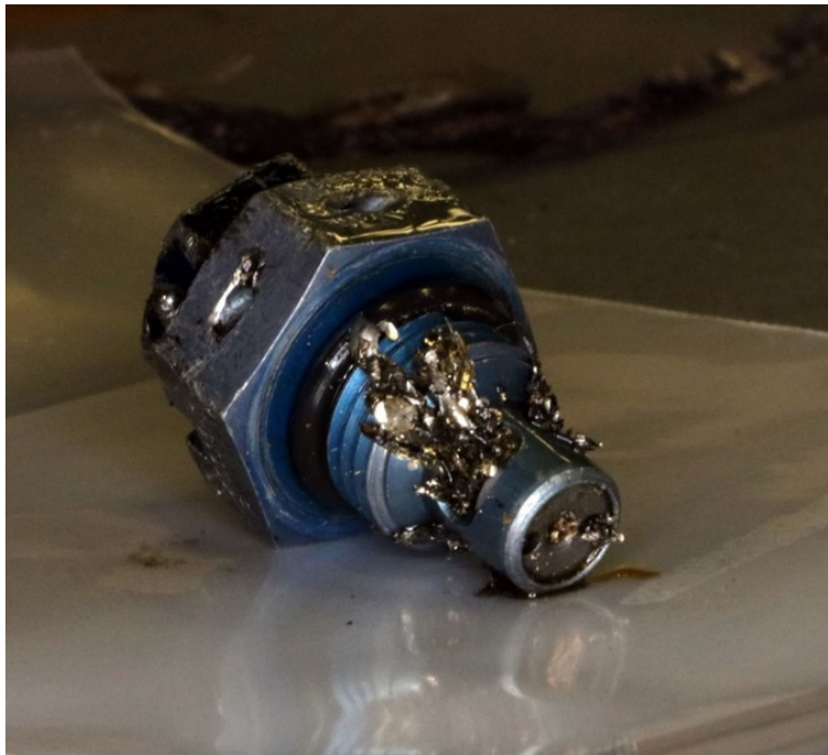
Photo 4- CSD Chip Detector Plug
