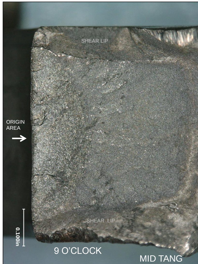
Views of the fracture surface on the mid tang after chemically removing the transferred aluminum. The white arrows indicate the location of the fatigue origins on the pin hole surface.
