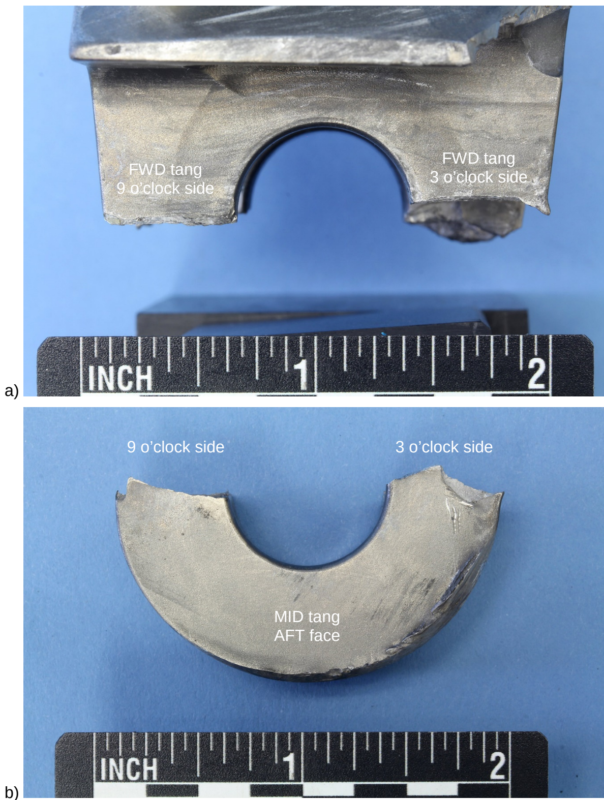
Figure 3: a) Image of the outboard portion of the fractured forward tang, viewed forward looking aft and b) image of the inboard portion of the fractured middle tang, viewed aft looking forward.
