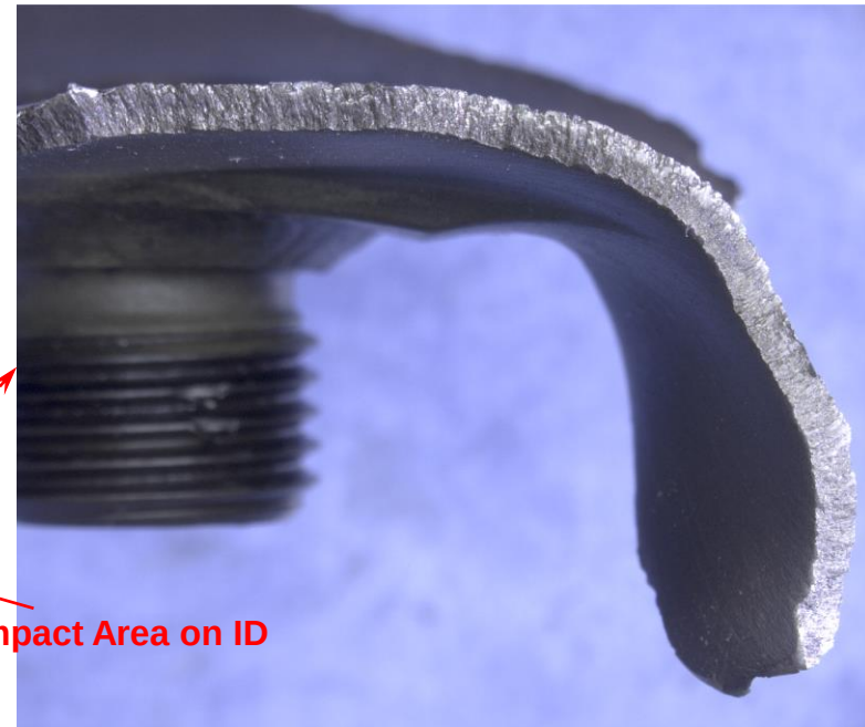
Figure 3: Optical views of the fracture surfaces of the liberated piece showing bulk deformation and rough/sheared fracture features consistent with instantaneous overstress/shear fracture.
