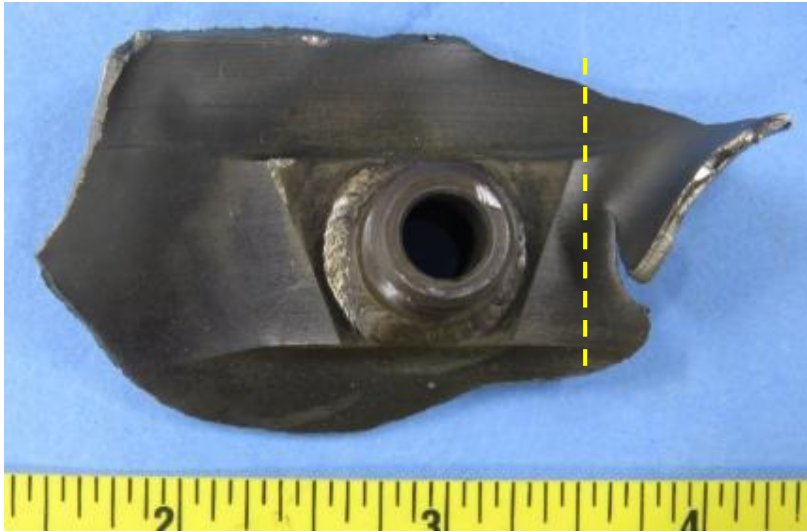
Figure 6 : A cross-sectional metallographic mount was made near the impact area showing a wrought structure with an average grain size of approximately ASTM 5, conforming to the requirement of AMS 5707. At the fracture (lower left) the wall was distorted and the grains were locally deformed consistent with a shear region.
