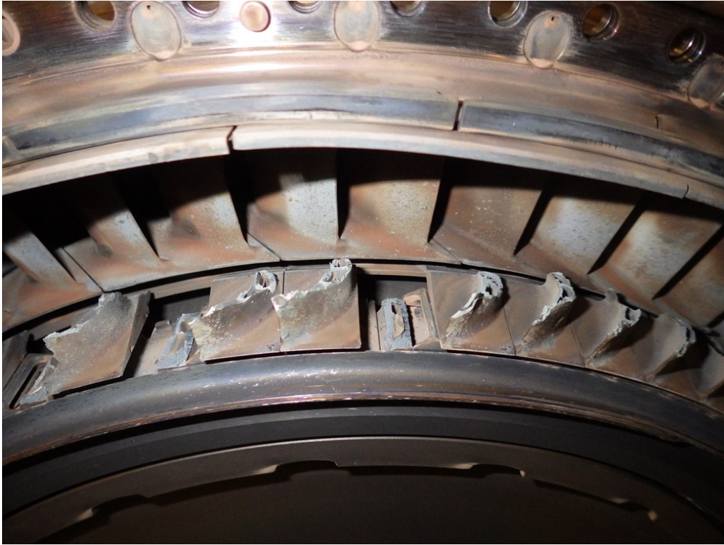
Photo 7- HPT 2 nd Stage Blade Damage
