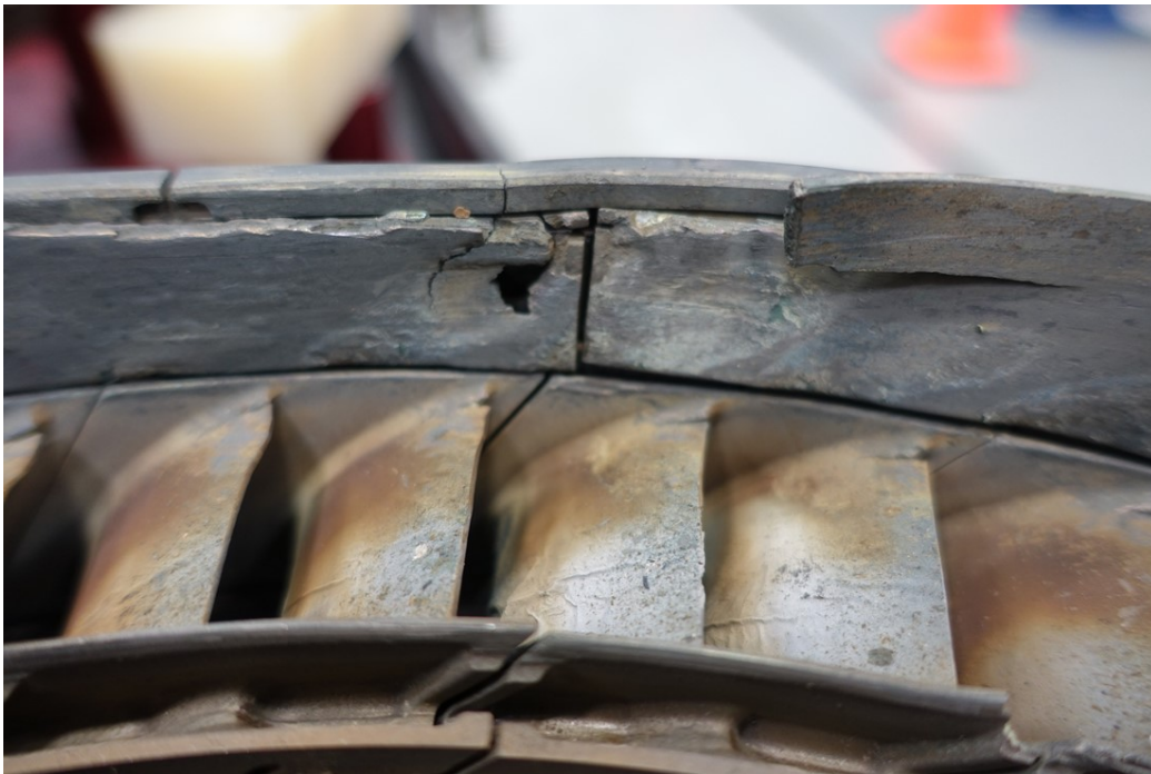
Photo 8- HPT 2 nd Stage Blade Shroud
