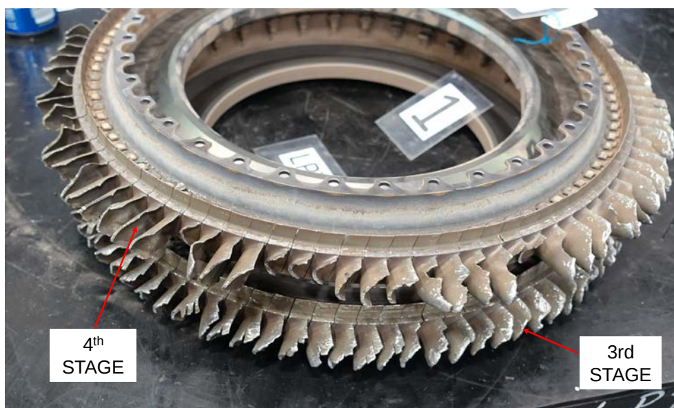
Photo 11- LPT 3 rd and 4 th Stage Rotor Blade Damage
