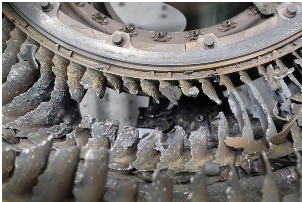
Photo 10- LPT 3 rd Stage Nozzle Vane Thermal Damage
