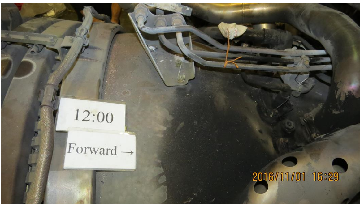
Photo 6- Localized Soot/Discoloration, 12 o'clock
