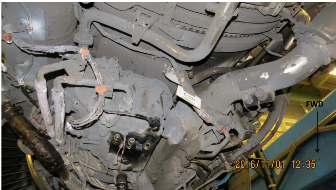
Photo 5- Soot/Discoloration and Thermal Damage, 6 o'clock
