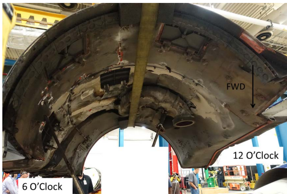
Photo 10- Outboard Thrust Reverser Cowl Damage
