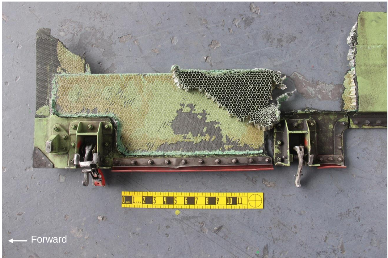
Figure 9: Forward lower portion of outer skin with number 1 latch still attached. The inner skin was disbonded from the core at the upper aft corner of the piece. The outer skin was disbonded from the core over the remainder of the piece. The skin separated along the edge of a doubler along the lower edge of the cowl.
