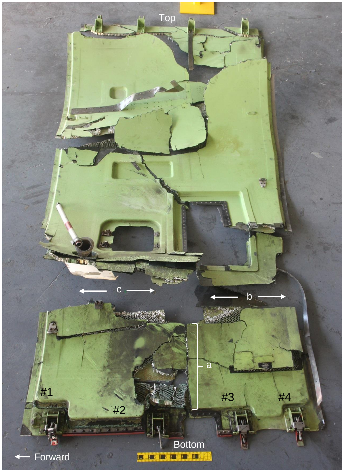
Figure 4: Inner view of the reconstructed right side fan cowl.
