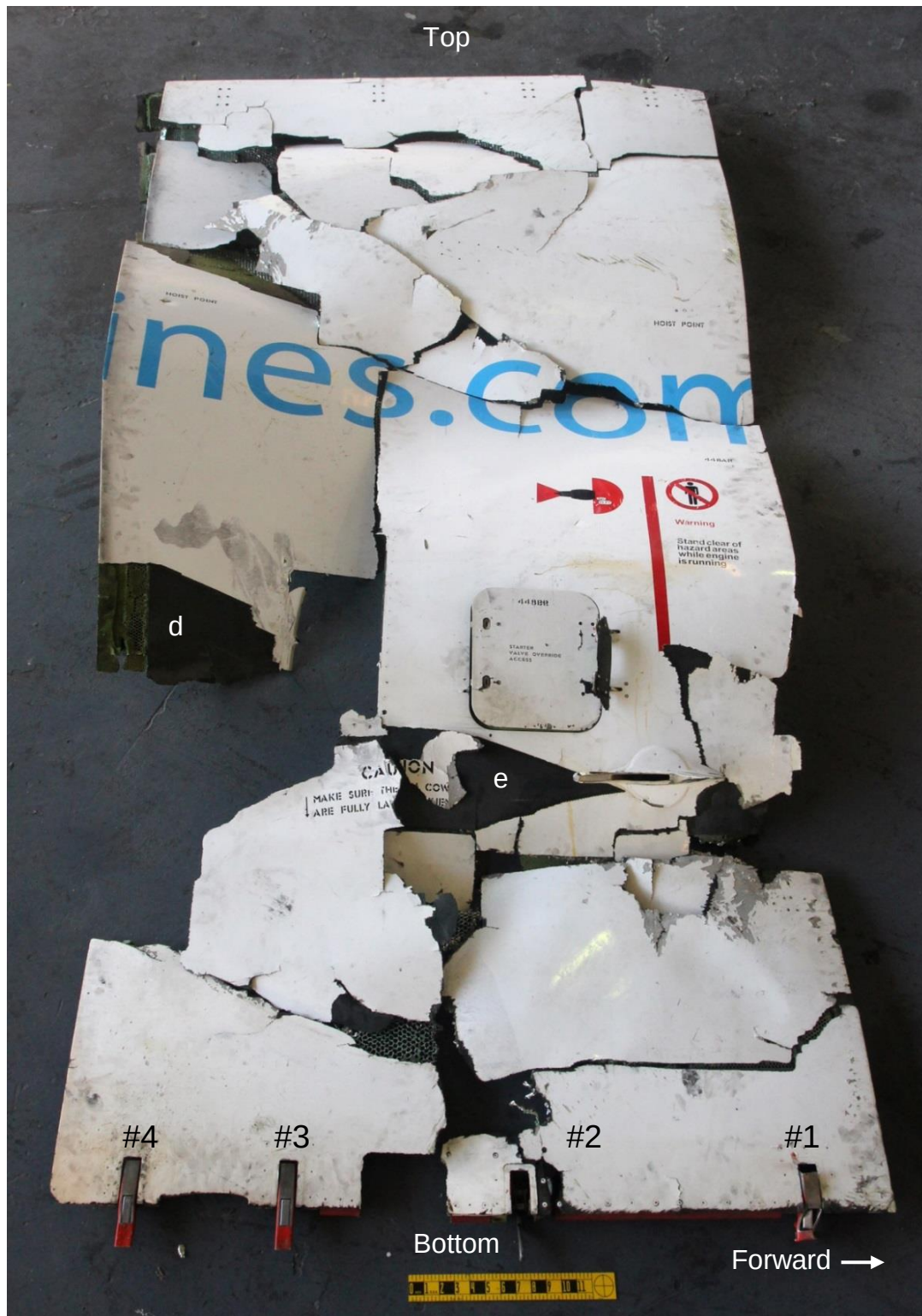
Figure 3: Outer view of the reconstructed right side fan cowl.
