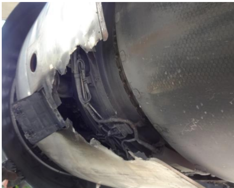
Figure 5. Right engine inboard core cowl burn-through
