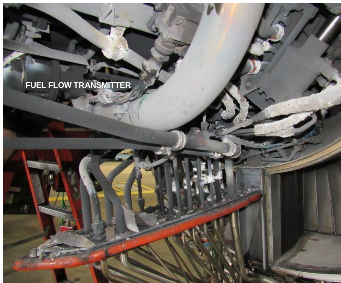
Figure 12. Right side of the FFT showing heavy sooting
