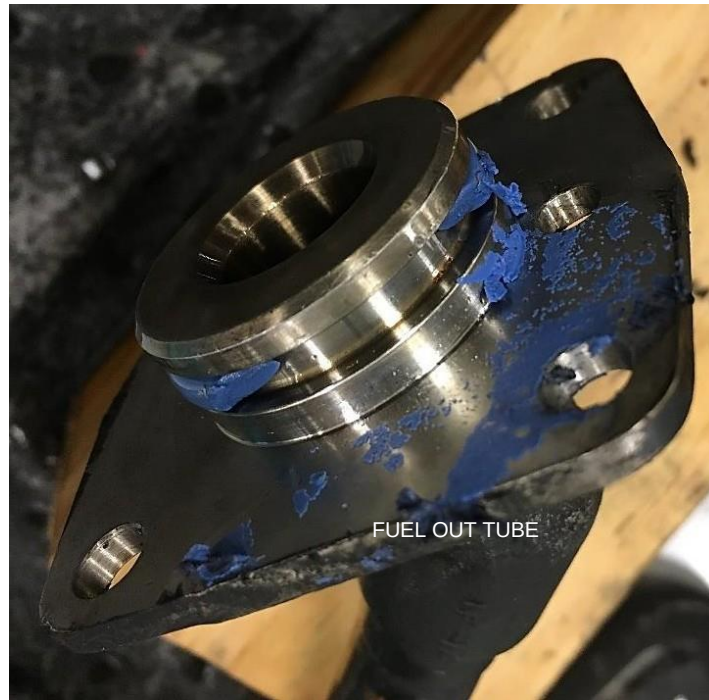
Figure 17. Fuel OUT tube showing damaged O-ring in tube gland and O-ring material deposited on flange surface
