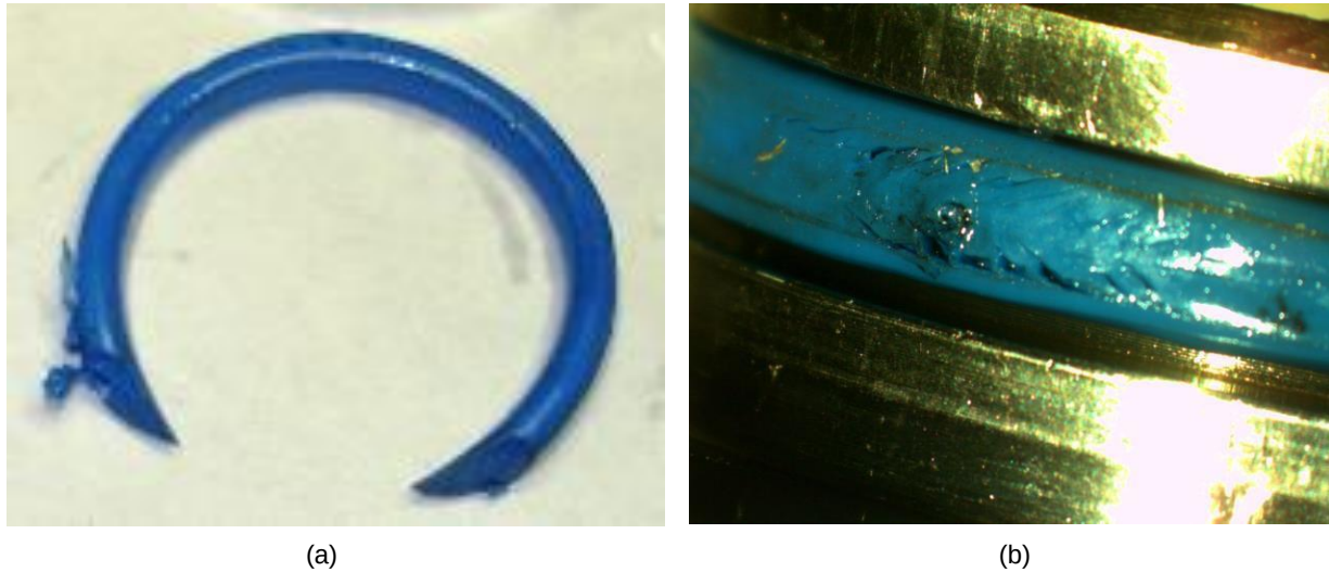
Figure 18. FFT fuel OUT tube O-ring showing (a) missing arc of material and (b) O-ring surface damage
