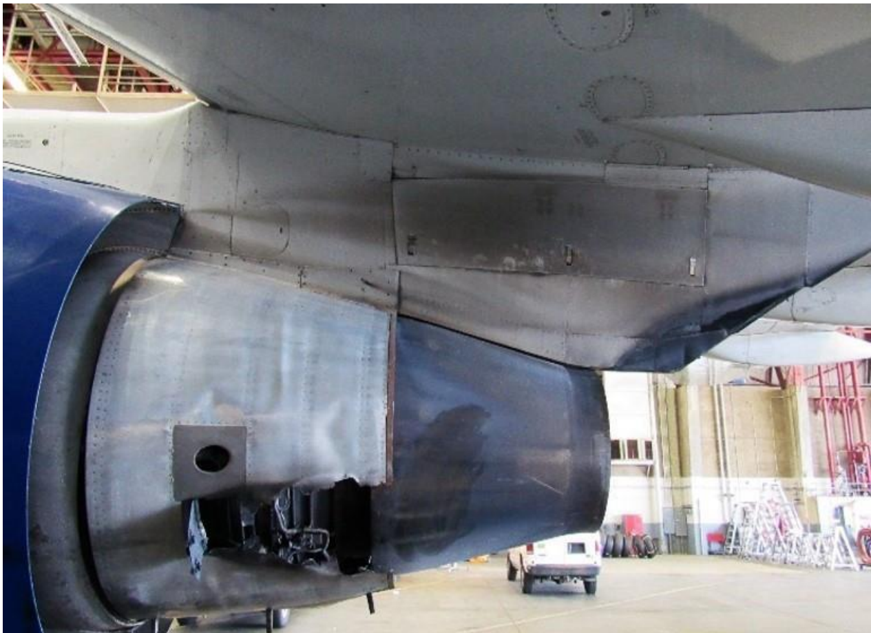
Figure 1. Right nacelle, showing cowling burn-through
