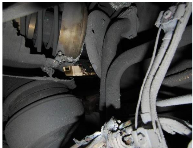
Figure 11. Partially-consumed fan air valve
