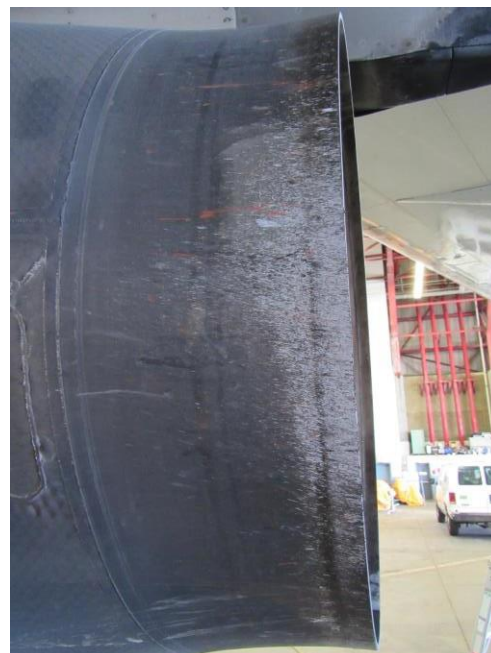
Figure 6. Exhaust nozzle deposits
