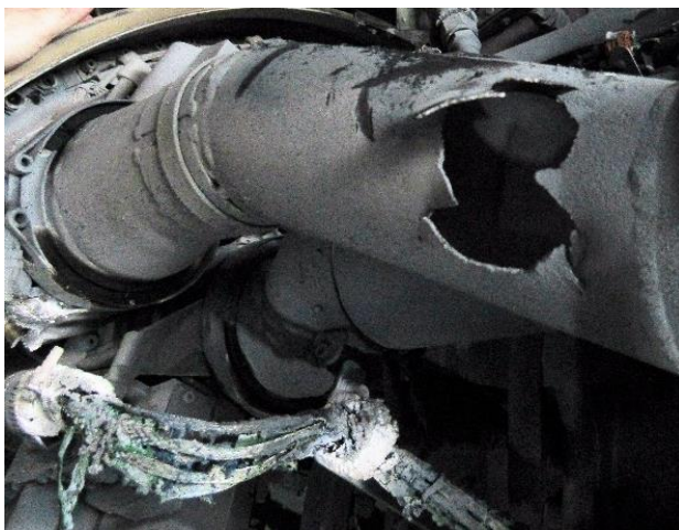
Figure 10. Ruptured TCC line
