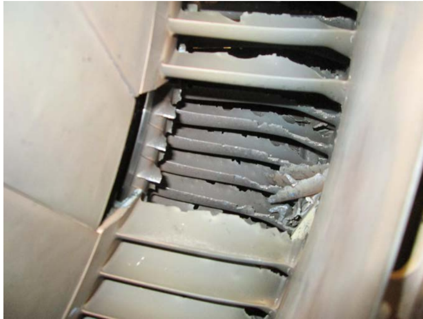
Photo No. 1: View from the front of the location of the missing 3rd stage turbine vane cluster. (Delta)
