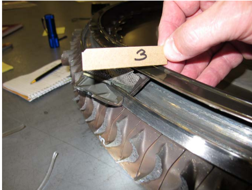
Photo No. 6: View of 3rd stage turbine vane cluster inner shroud showing relation between rub mark across the airfoils in relation to the 3rd stage rotating air seal. (P&W)
