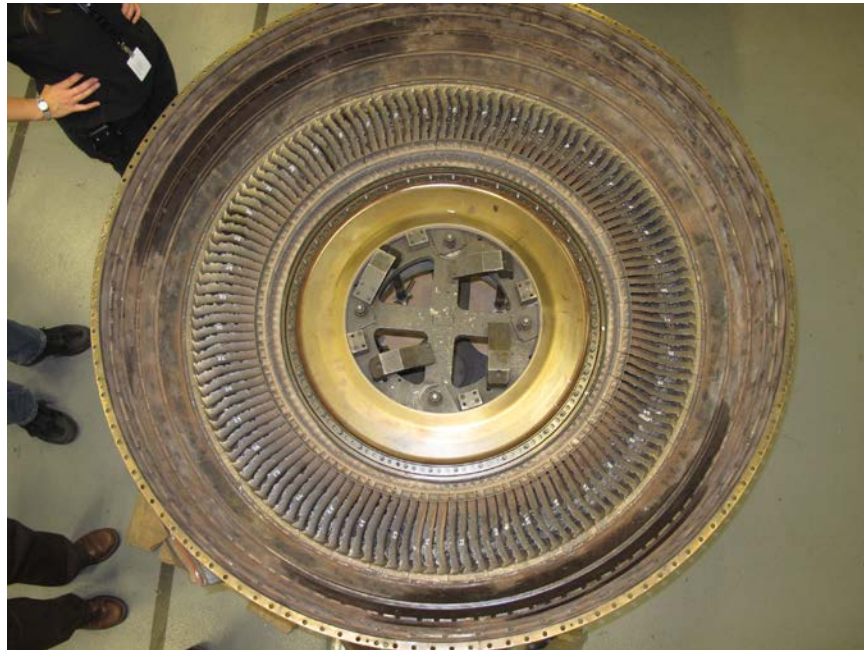
Photo No. 13: View of 4th stage turbine vane clusters showing all are in place in the LPT case. (P&W)
