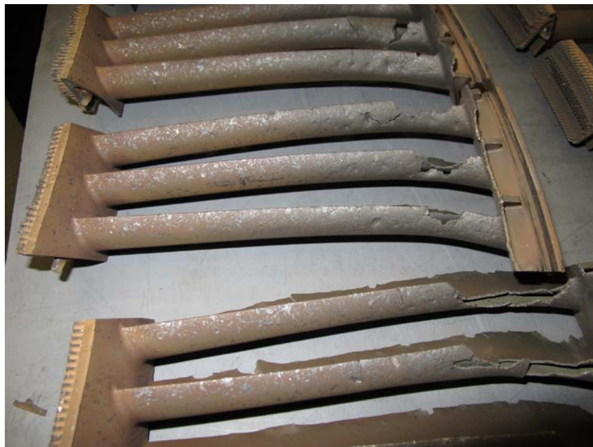
Photo No. 18: Close up view of damage to leading edges of 5th stage turbine vane clusters. (P&W)
