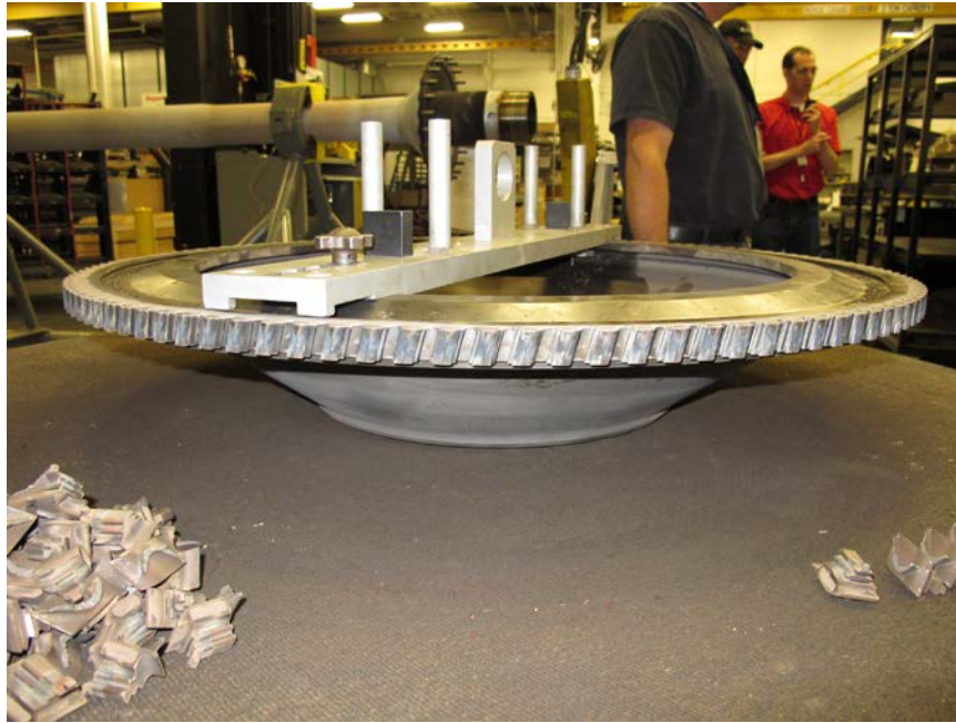
Photo No. 19: View of 5th stage turbine disk showing that it was intact. (P&W)
