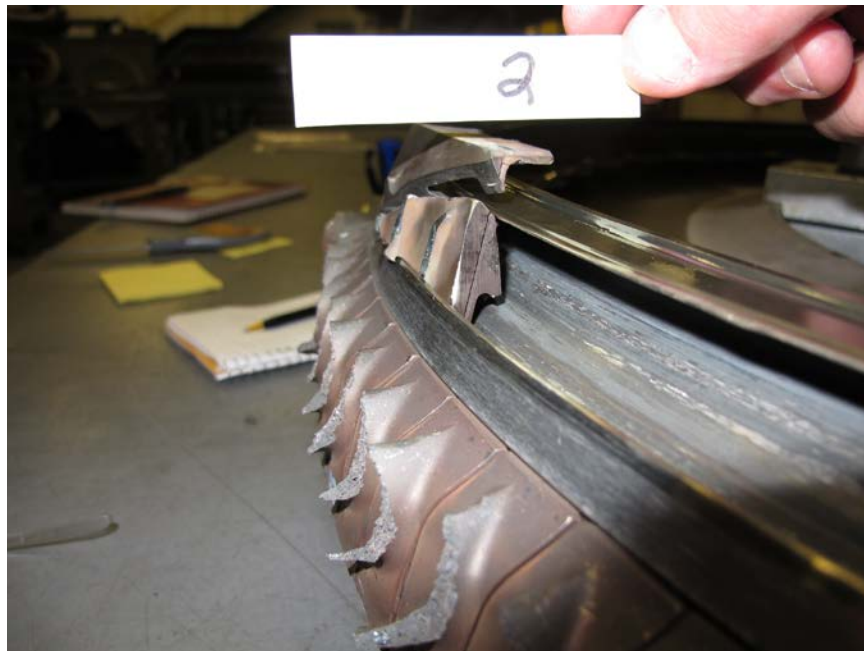
Photo No. 5: Side view of 3rd stage vane cluster inner shroud showing the circumferential rub mark on the rear of shroud in relation to the edge of the rim of the 3rd stage rotating air seal. (P&W)
