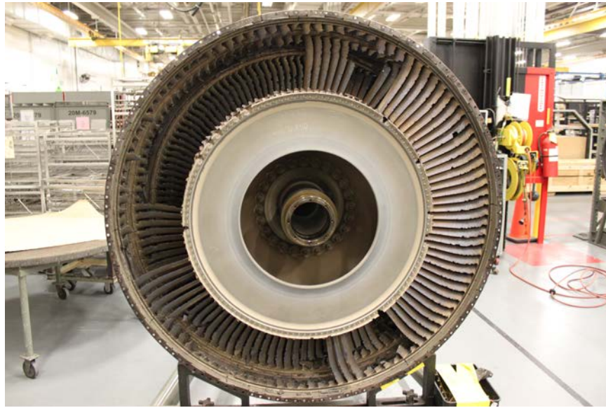
Photo No. 23: View of 6th stage turbine disk showing that it was intact. (Delta)
