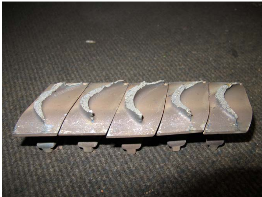
Photo No. 20: Close up view of 5th stage turbine blades showing coarse and grainy fracture surfaces. (P&W)
