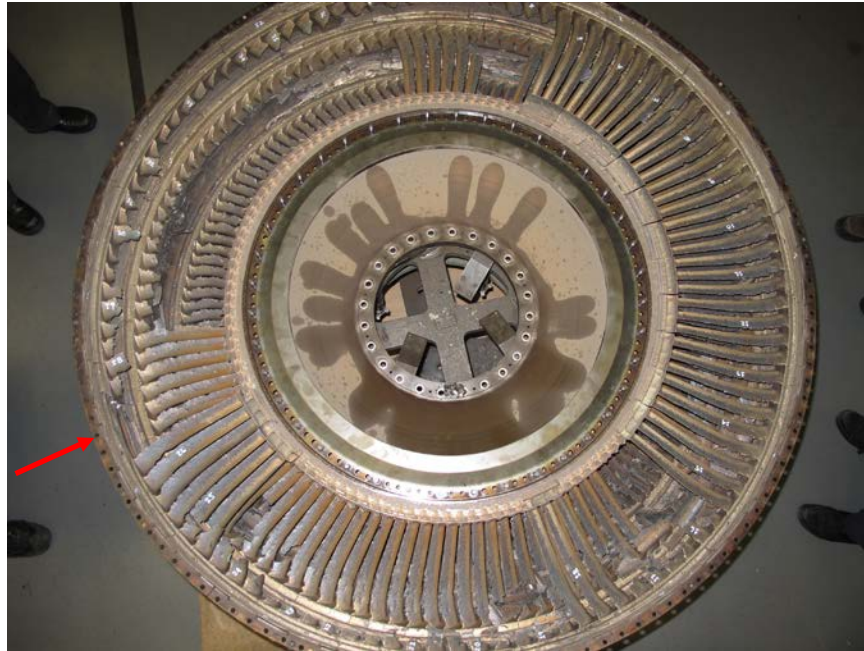
Photo No. 21: View of 6th stage turbine vane clusters with an arrow showing the location of the missing cluster. (P&W)
