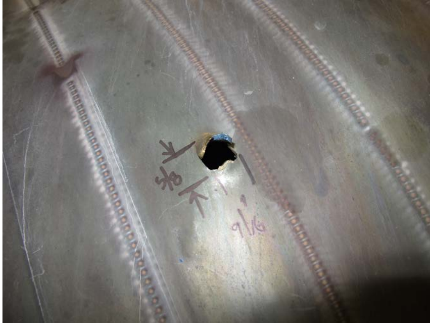
Photo No. 9: Hole in LPT case in plane of 3rd stage turbine rotor at 10:30 o'clock. (P&W)
