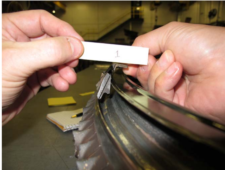
Photo No. 4: Side view of piece of 3rd stage turbine vane cluster inner shroud showing relation of circumferential rub mark on underside of shroud to 3rd stage rotating air seal knife edge. (P&W)
