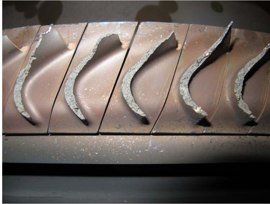
Photo No. 16: Close up view of fractured 4th stage turbine blades showing coarse fracture surface. (P&W)
