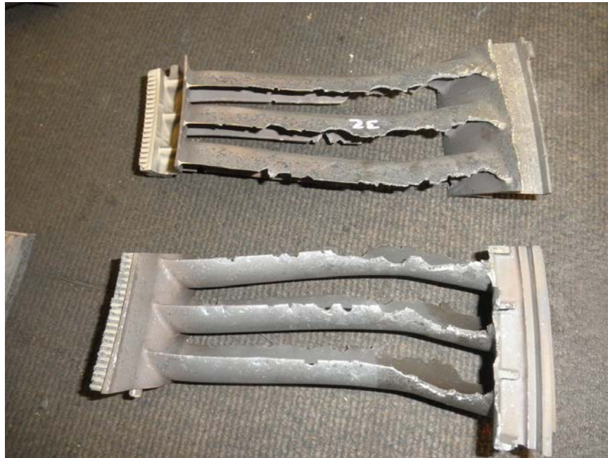
Photo No. 7: Other 3rd stage turbine vane clusters, trailing edge on the top and leading edge on the bottom.
