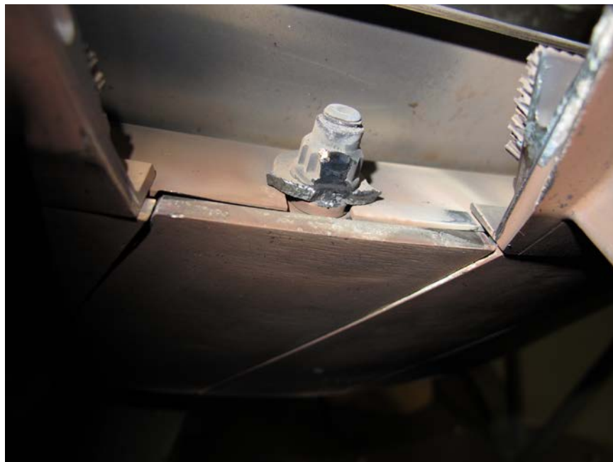
Photo No. 2: Close-up view of bolt hole tab and retaining nut that remained attached to the inner transition duct. (P&W)
