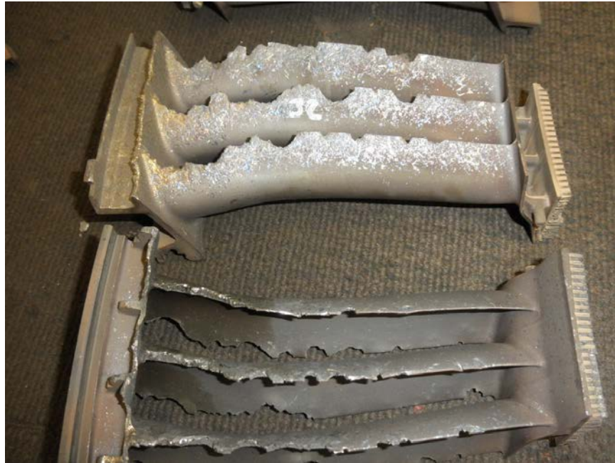
Photo No. 14: Close up view of 4th stage turbine vane clusters showing damage to the leading and trailing edges of airfoils.
