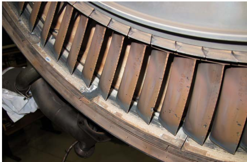
Photo No. 27: Close up view of 2nd stage turbine blades showing damage to trailing edges and the erosion to the blade outer air seals. (P&W)
