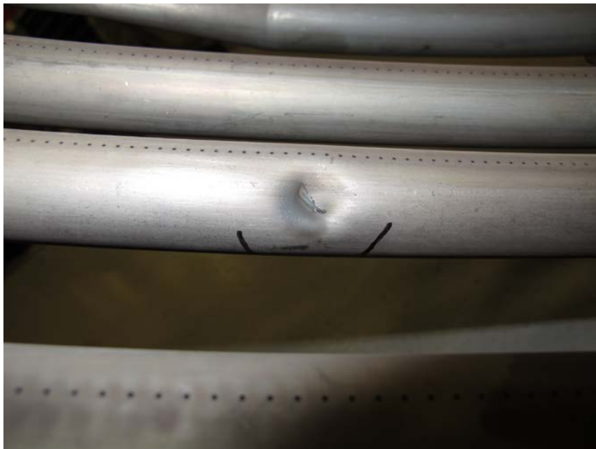
Photo No. 26: Close-up view of dent on inner surface of turbine cooling air manifold. (P&W)
