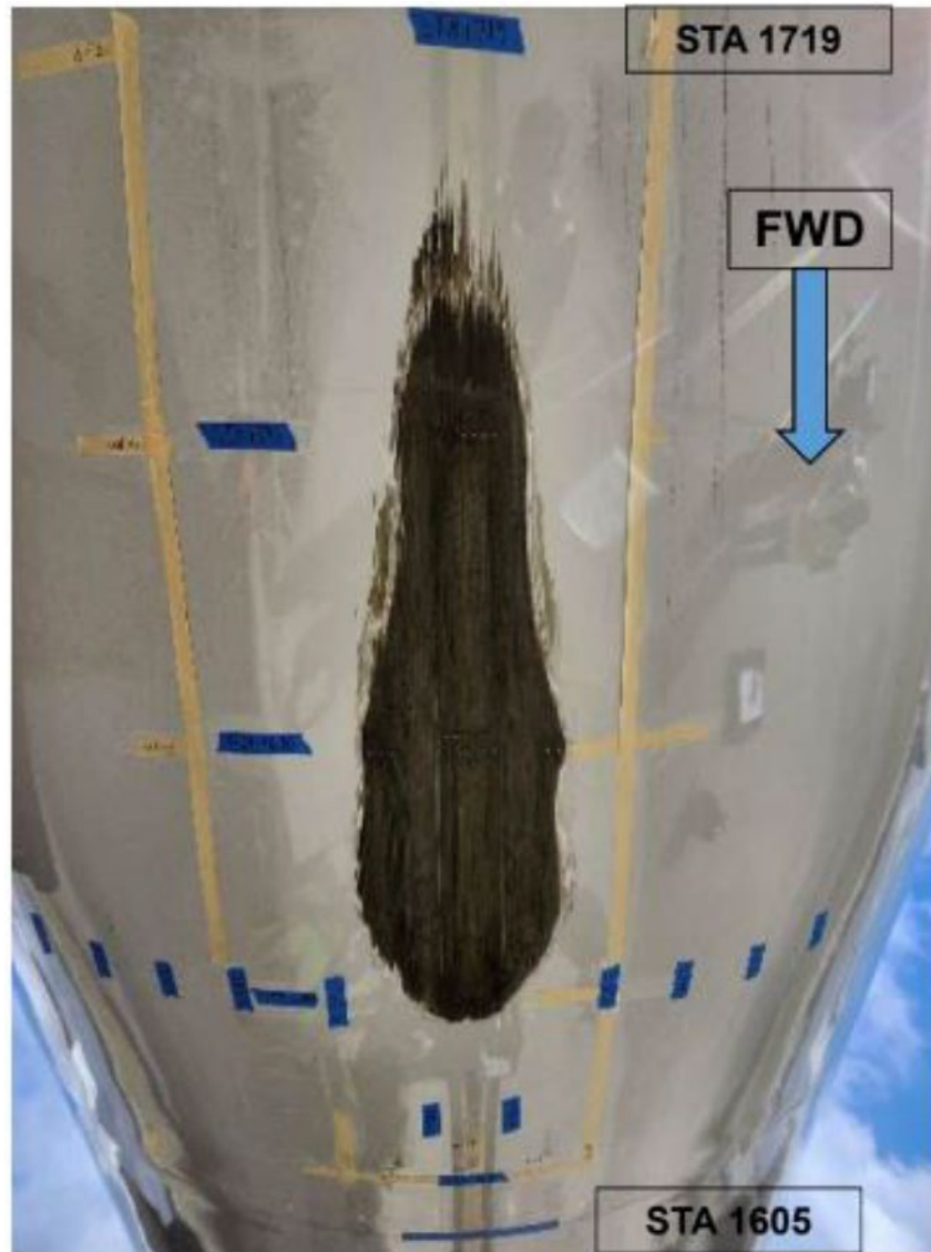
Photograph 2 - Damage to the lower fuselage between stations 1605 and 1719. (Courtesy of ANA)
