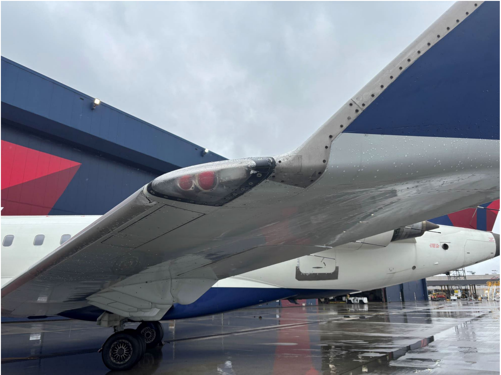
Photo 2 – Right-wing leading-edge slat damage. (Source Endeavor Air)
