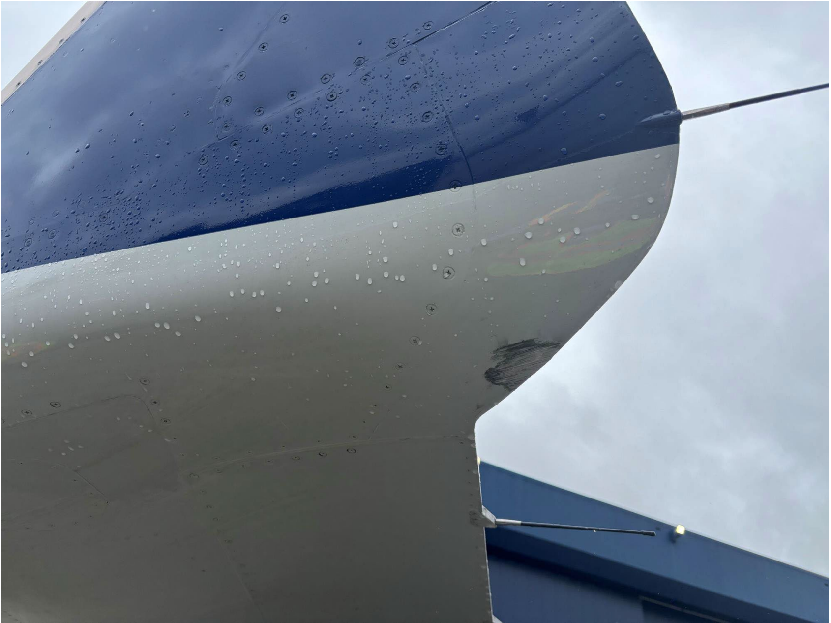
Photo 1 – Minor damage to right wing. (Source Endeavor Air)
