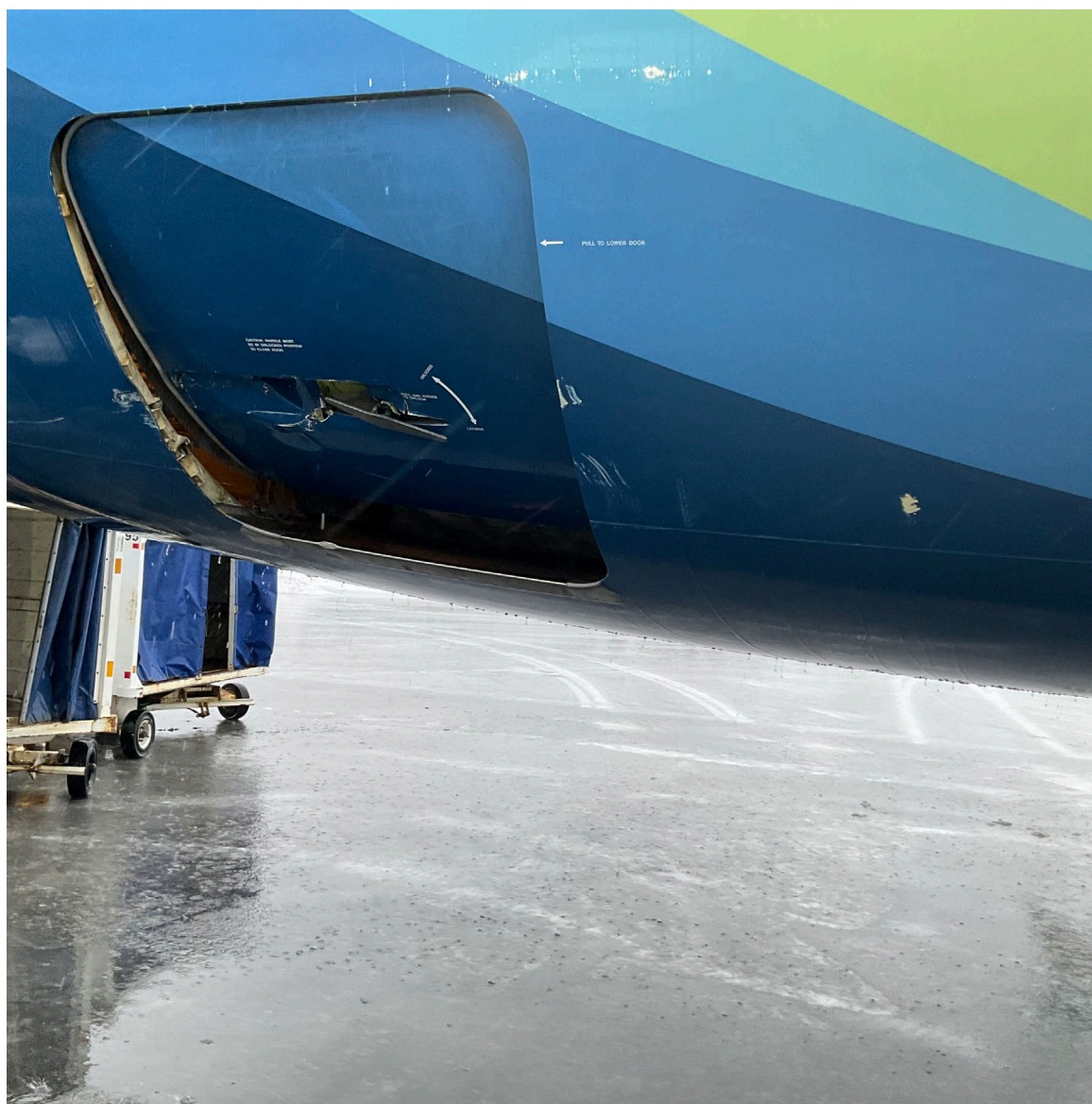
Photograph 1 - Damage to AFT Right Cargo Door and Frame (Courtesy of Alaska Airlines)
