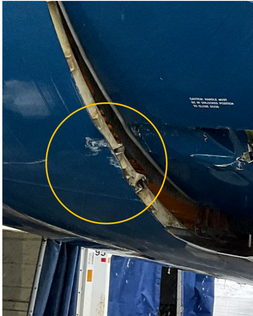
Photograph 2 - Damage to Door Frame (Courtesy of Alaska Airlines)
