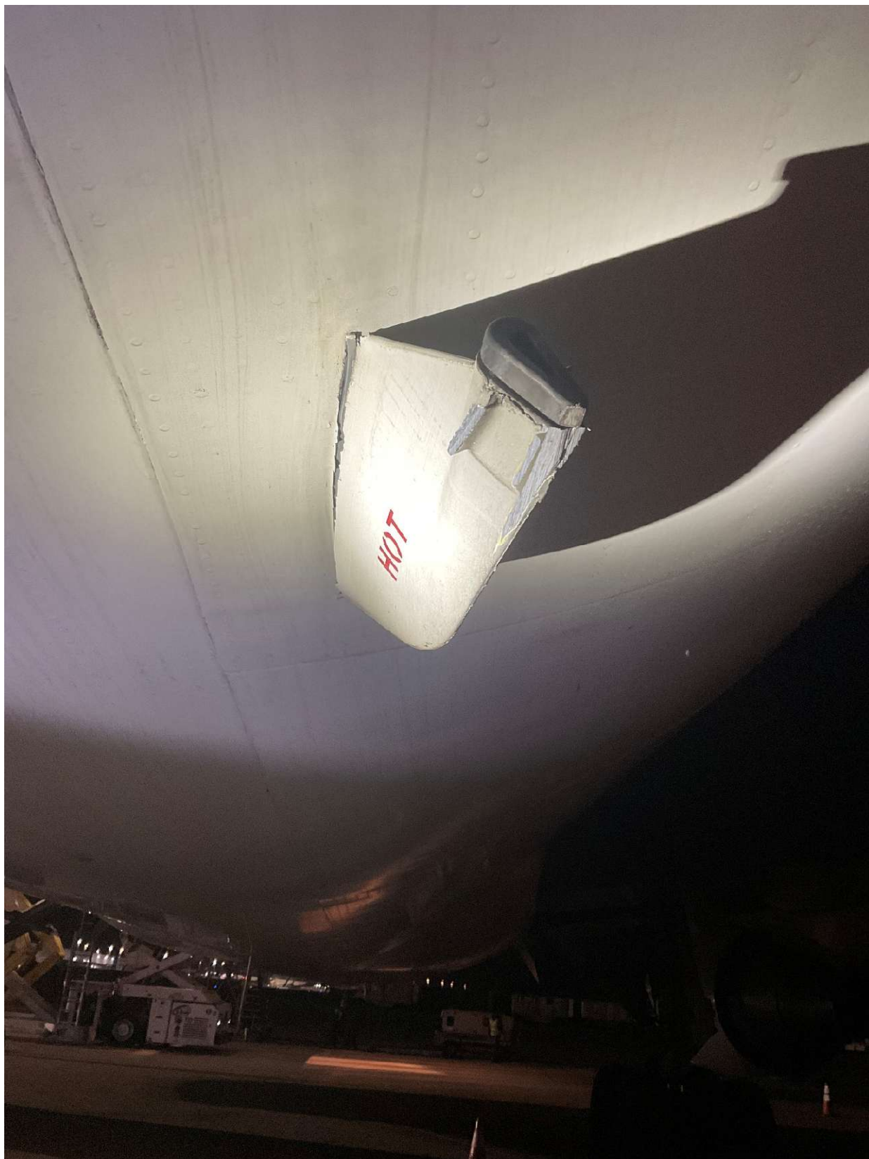
Photograph 5 - Drain mast damage.
