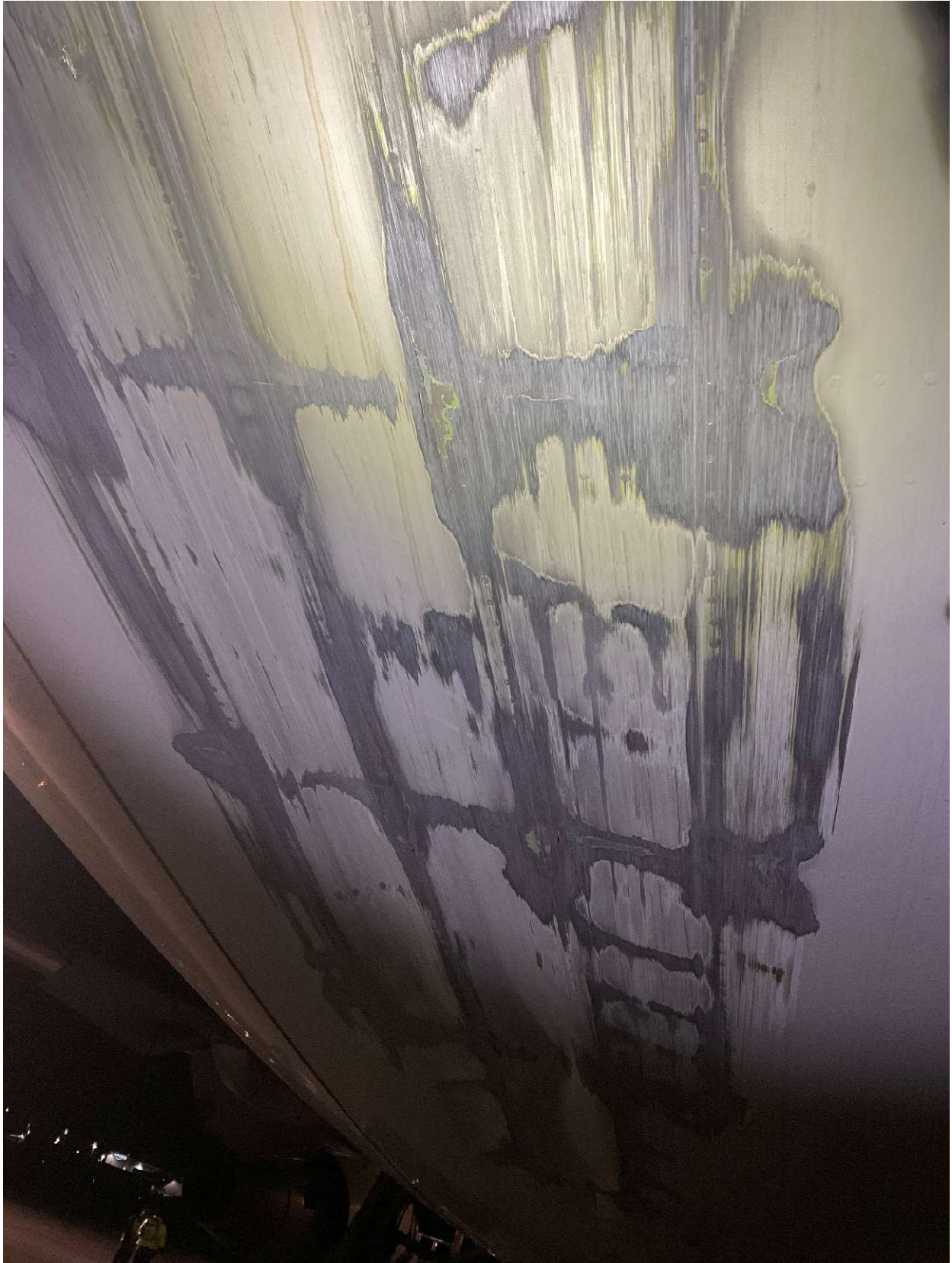
Photograph 4 - Lower fuselage damage near tail.
