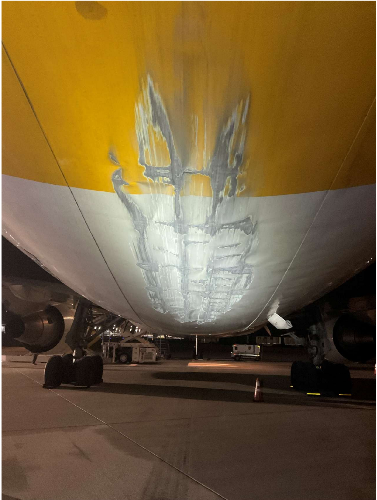
Photograph 1 - Lower fuselage damage near tail.
