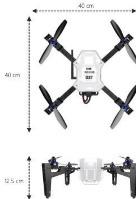
Figure 1. Technical specification for the UVify IFO drone (courtesy of Sky Elements).
