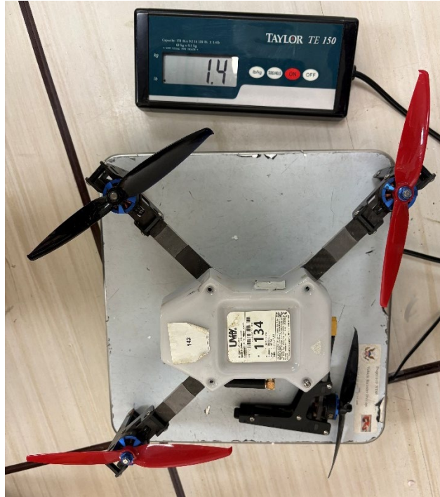
Figure 3. Weight of accident drone without battery.
