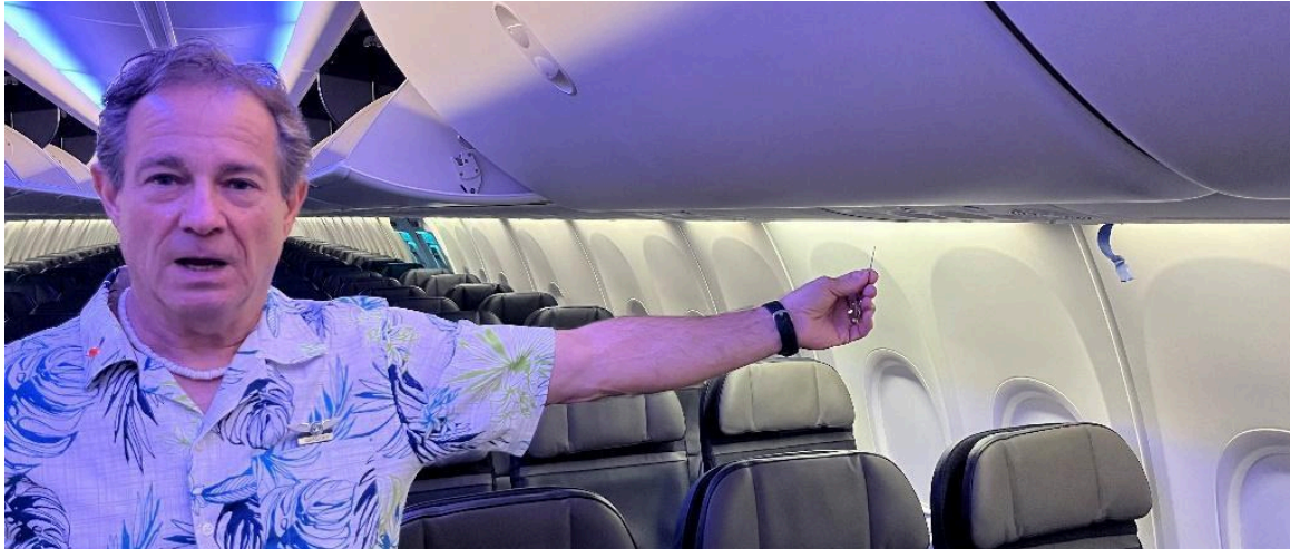
Figure 11. Actual reach to the manual release pinhole used to release the oxygen mask in a 737 with push-up bins (pinhole indicated by blue tape).
