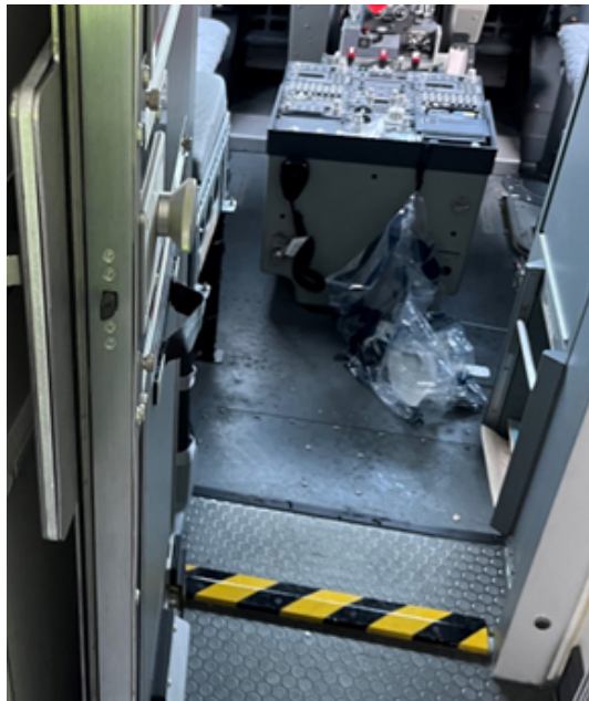
Figure 2. Photograph of entry to flight deck from cabin looking into the flight deck. The striped metal plate was added to the 737 MAX but is not present on the 737 NG.
