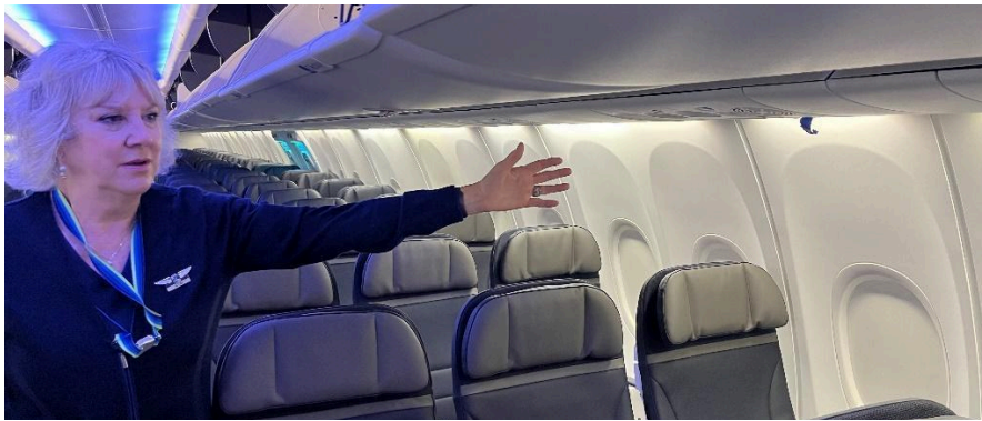
Figure 7. Reach from the aisle in premium class located in the main cabin of a 737 with push-up bins (a piece of blue tape marks the center of the oxygen compartment). Distance from the aisle armrest to the center of the oxygen mask compartment in the main cabin is 43", and the average measured Flight Attendant reach is 22".
