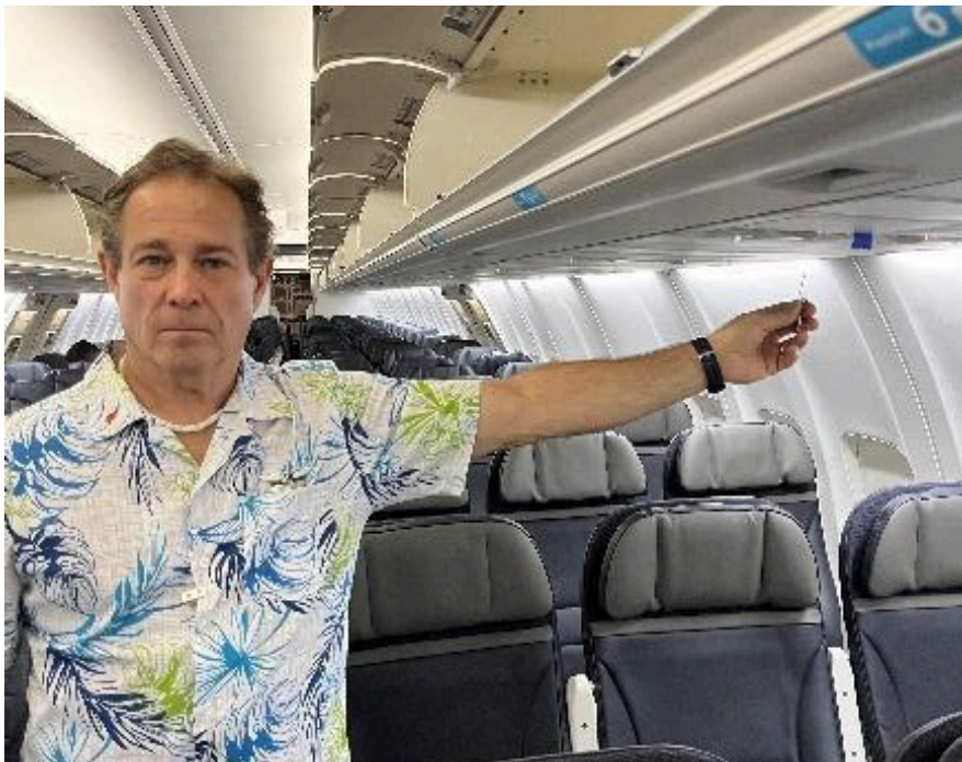
Figure 12. Actual reach to the manual release pinhole used to release the oxygen mask in a 737 with shelf-style bins (pinhole indicated by blue tape).
