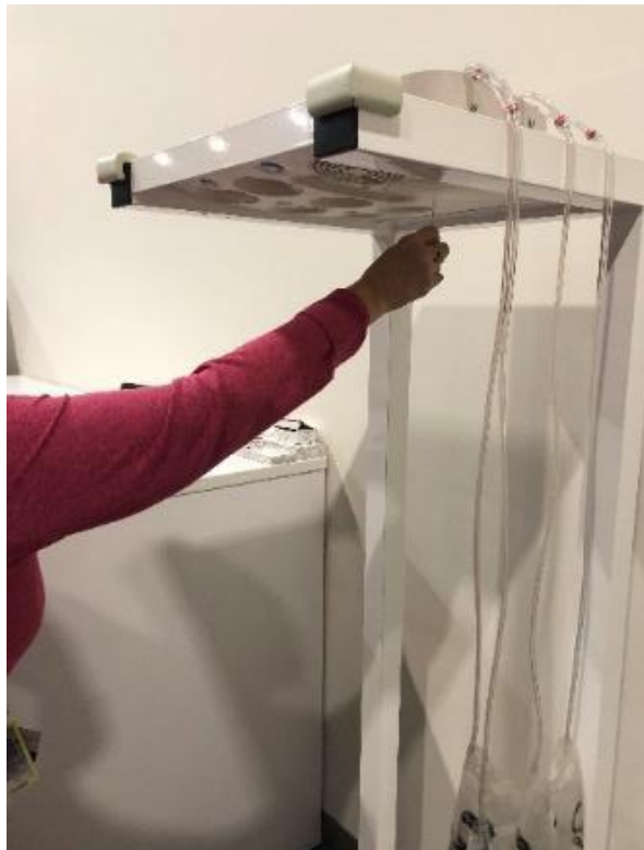
Figure 10. Training device used to simulate manual opening of oxygen mask compartments.
