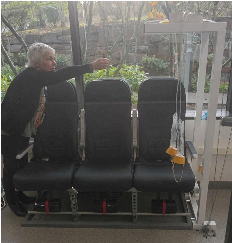
Figure 13. Training device with a row of seats which is more representative of the actual aircraft environment. Note that this does not demonstrate the additional restrictions caused by seat pitch or occupied seats.
