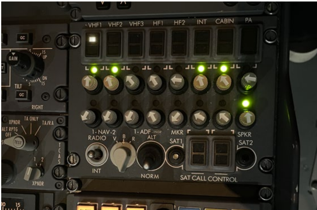
Figure 5. Establishing communication on the audio control panel (MAX)
