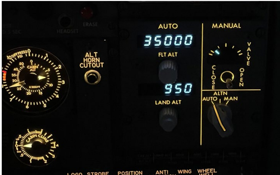
Figure 1. Cabin Altitude and Differential Pressure prior to Rapid Depressurization at FL350 (MAX)
