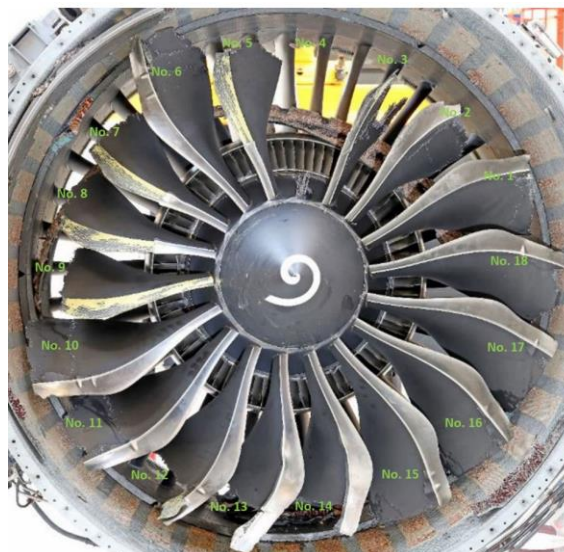
Figure 2: Fan Blade and Fan Case Damage
