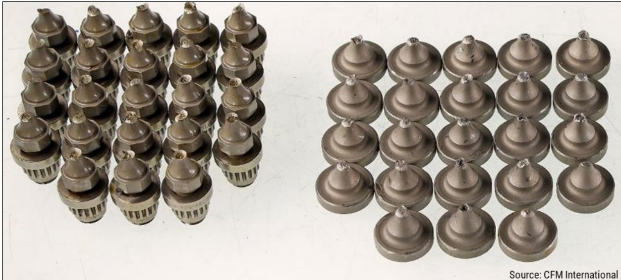
Figure 6: Fractured No. 1 bearing housing support shear bolts
