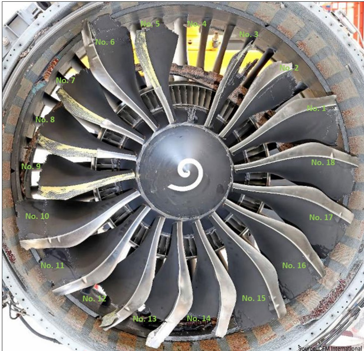
Figure 5: Fan blade and fan case damage
