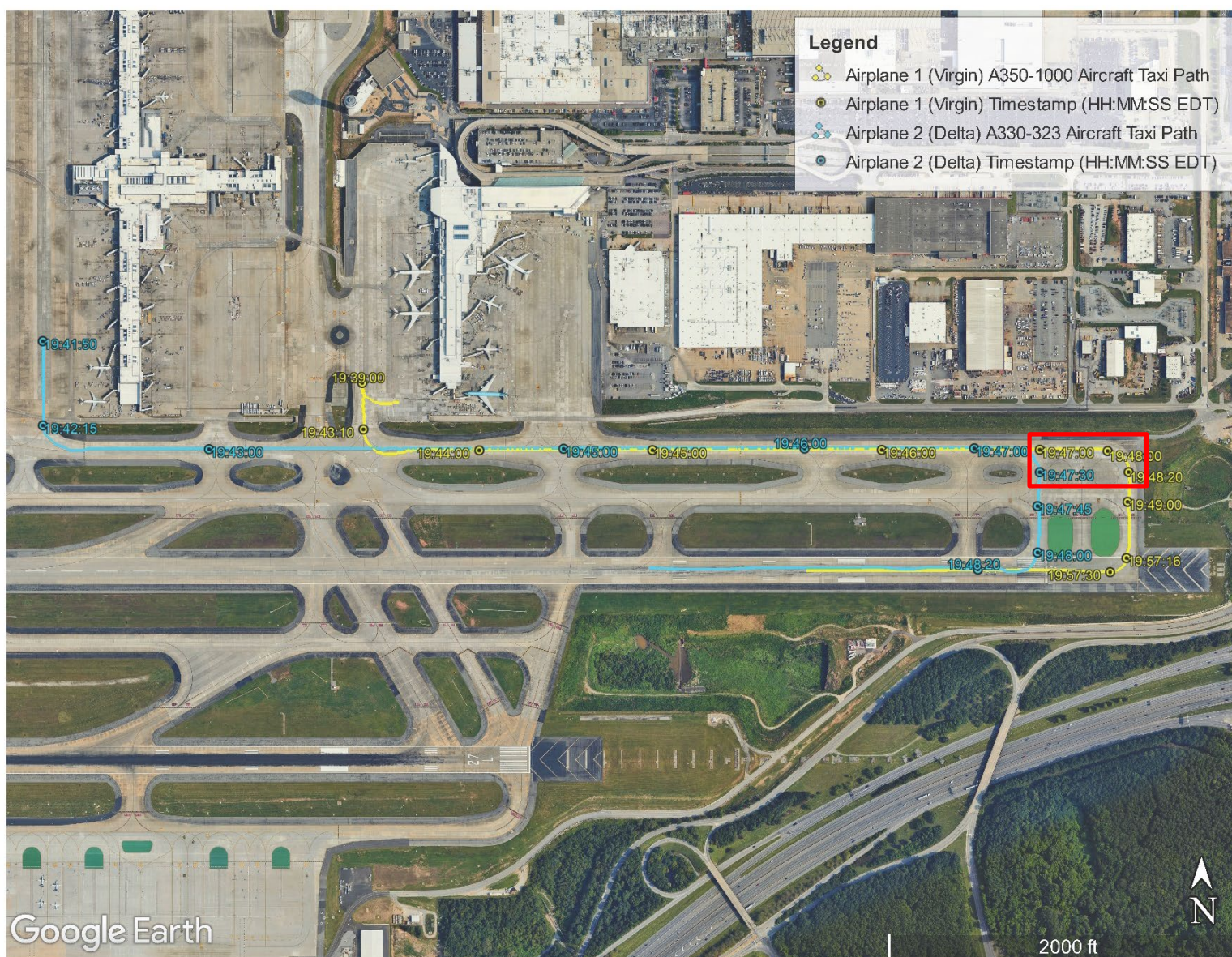
Figure 5. Google Earth overlay of the taxi for both aircraft to runway 27R using ADS-B data. The red box represents approximate location where the wingtip of Airplane 2 (Delta) struck the horizontal stabilizer of Airplane 1 (Virgin).
