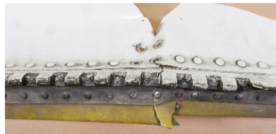
Figure 71: Bend and fracture common to RH APU door section
