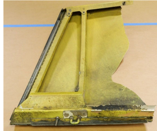
Figure 8: Aft section of LH APU door, inboard surface
