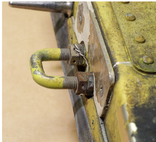
Figure 19: U-bolt on the aft LH APU door section
