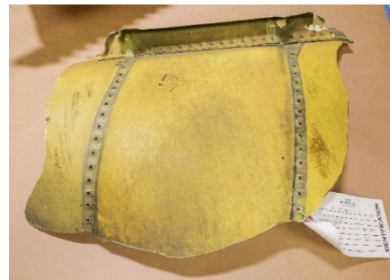
Figure 64: Remaining LH APU door section, inboard side
