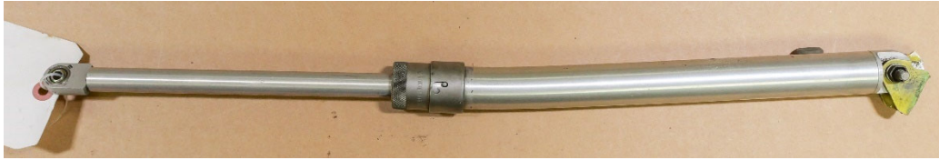
Figure 76: Bend in body of hold open strut
