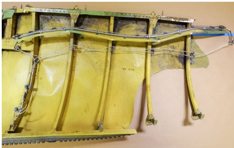
Figure 22: Missing section of skin and support ribs
