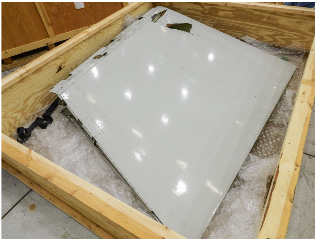
Figure 42: Overview image of damaged RH elevator assembly
