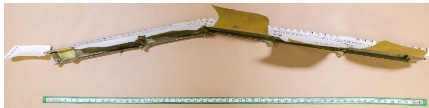
Figure 68: RH APU door section, placed on hinged edge
