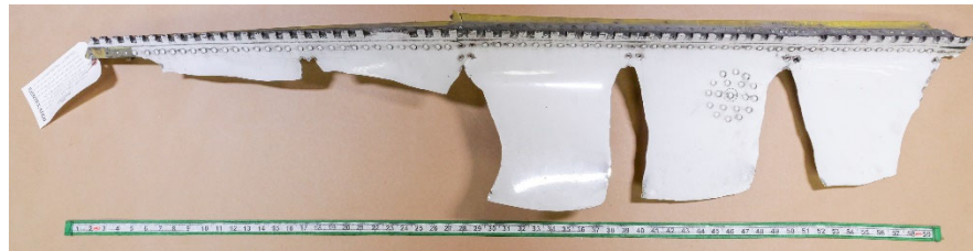
Figure 67: RH APU door section, outboard side
