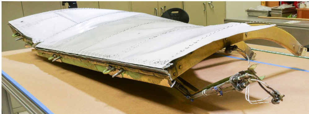
Figure 24: Forward LH APU door section, aft-inboard corner
