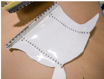
Figure 63: Remaining LH APU door section, outboard side
