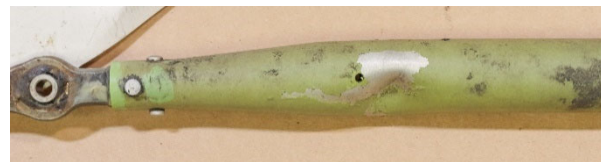
Figure 74: Dent in rod assembly, rotated approximately 90 degrees
