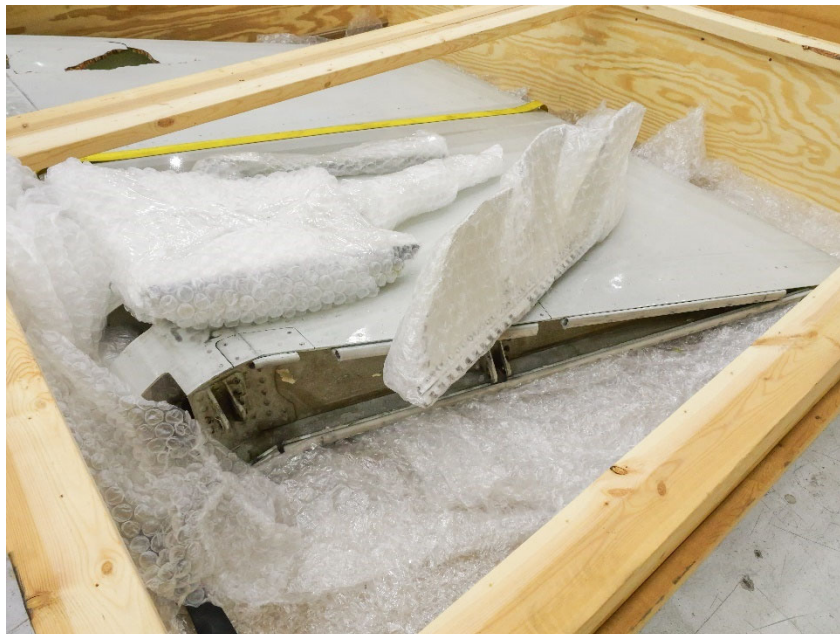
Figure 40: RH elevator assembly and seven additional parts
