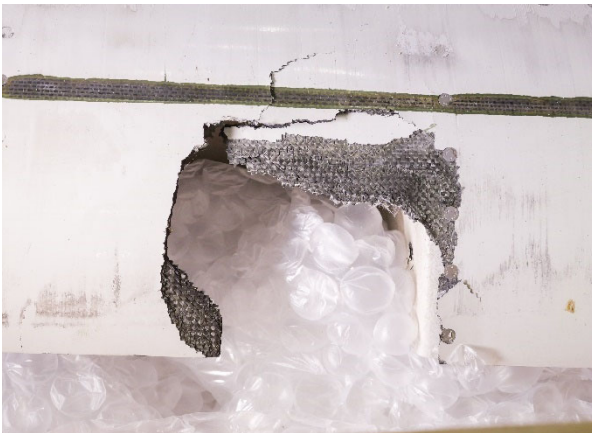
Figure 58: Missing section of material on LH elevator
