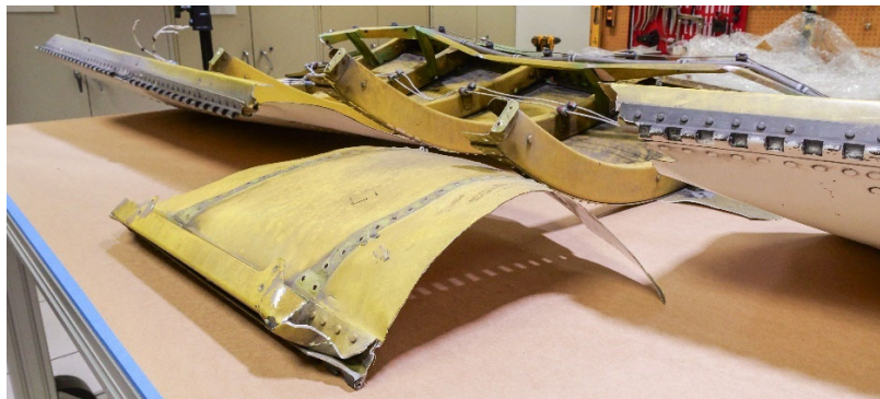
Figure 66: End view of LH APU door section
