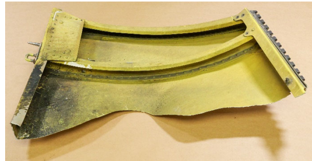
Figure 10: Aft section of LH APU door, inboard surface
