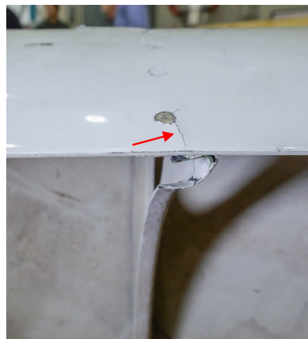
Figure 50: Crack on lower surface of RH elevator
