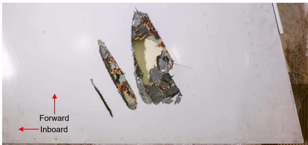
Figure 60: Damage on lower aft outboard surface of LH elevator
