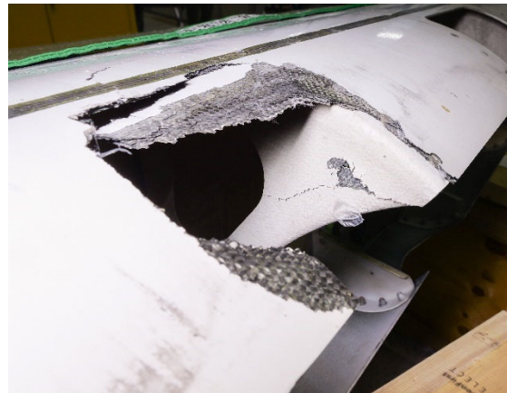
Figure 59: Missing section of material on LH elevator
