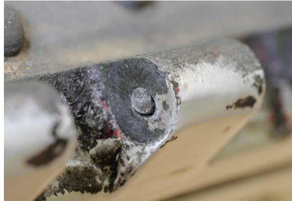
Figure 18: Example of ovalized hinge barrel hole
