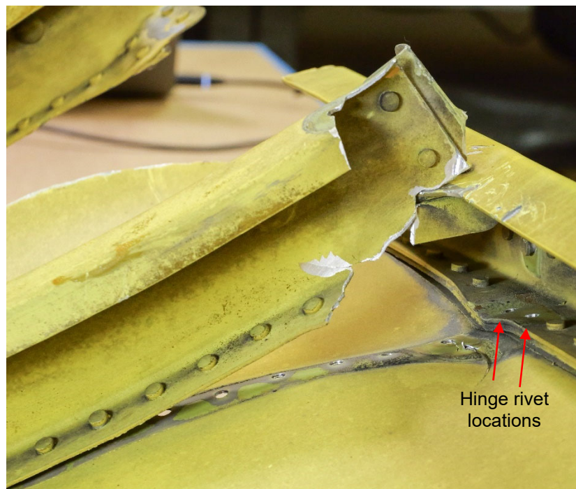
Figure 28: Fourth support rib separated from skin and hinge
