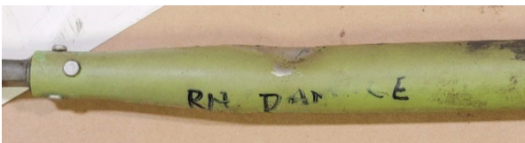
Figure 73: Dent in rod assembly
