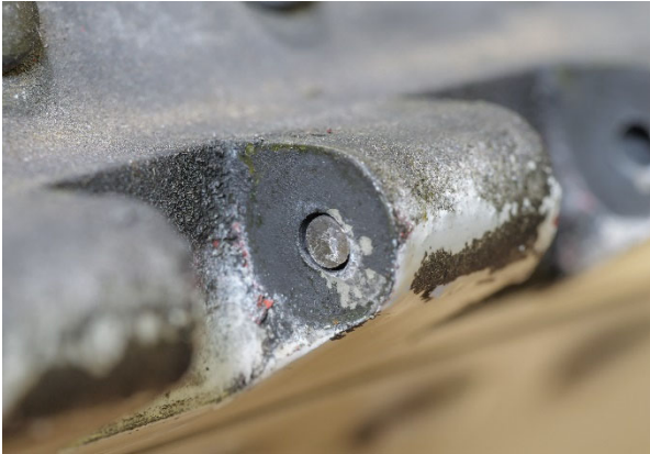
Figure 17: Example of ovalized hinge barrel hole
