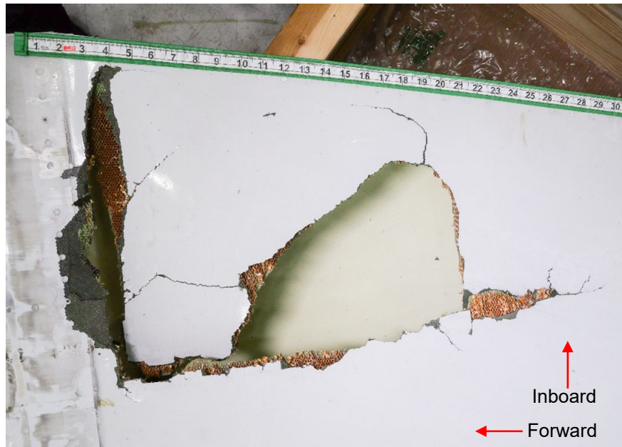
Figure 44: Damage on lower forward inboard surface of RH elevator
