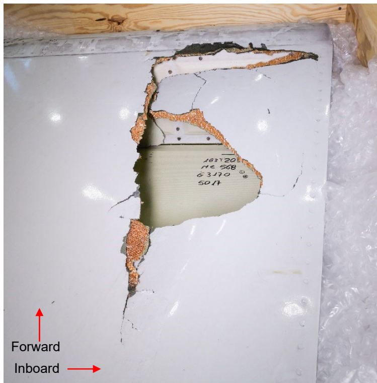
Figure 45: Damage on lower forward inboard surface of RH elevator
