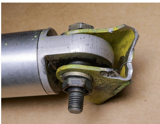
Figure 79: Fractured attachment bracket on the hold open strut
