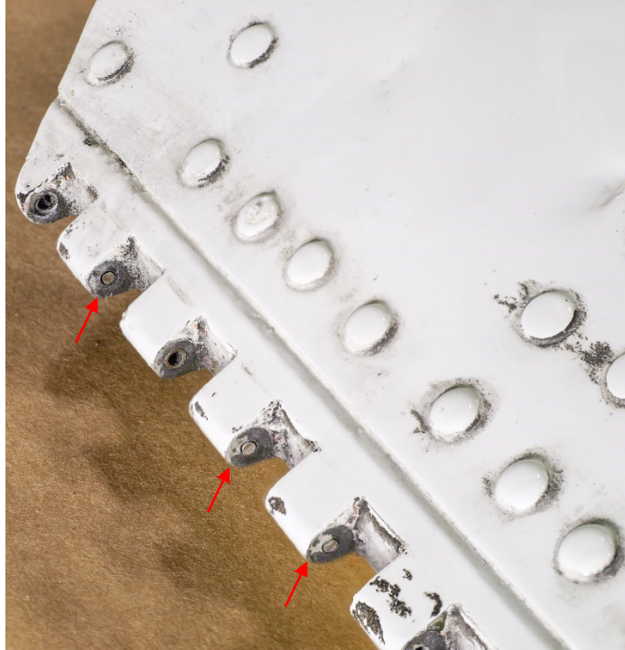
Figure 15: Hinge pin pieces within hinge barrels of the aft LH APU door section
