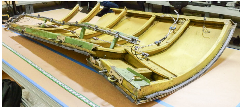
Figure 30: Forward-inboard corner of the forward LH APU door section
