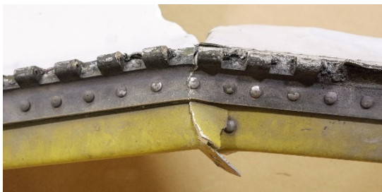
Figure 70: Bend and fracture common to RH APU door section
