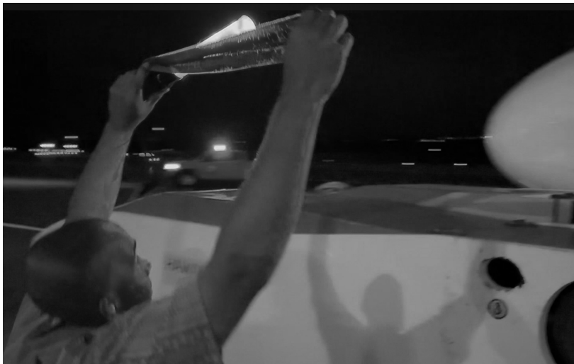
Figure 4. A ramp agent displaying the pin and ribbon with a lighted wand. (Not the accident agent)
