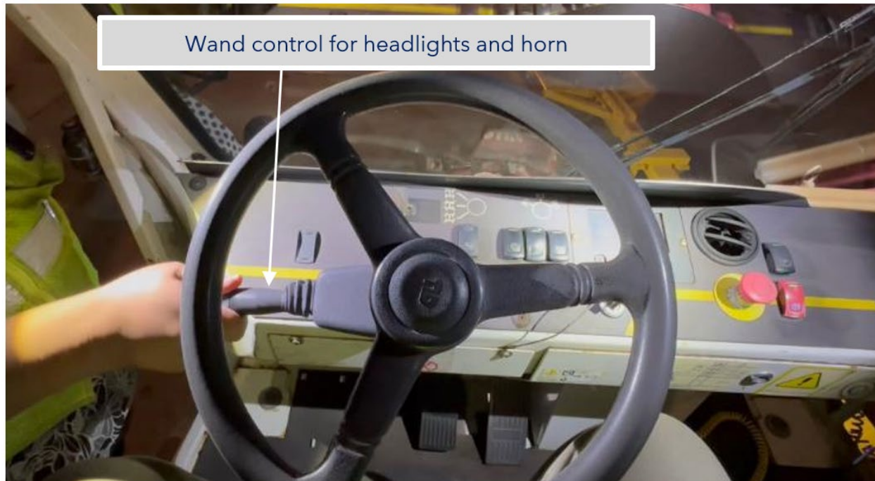
Figure 8: Wand control for the vehicle's headlights with a horn button on the tip.
