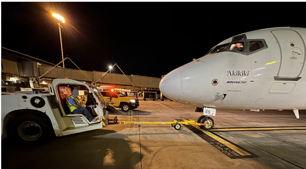
Figure 2. Tow tractor connected to the airplane. (Not the accident flight)
