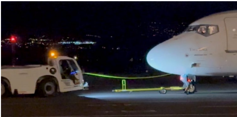
Figure 8: Escort disconnecting towbar from airplane.
