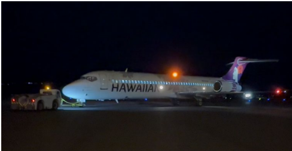
Figure 5: Exemplar B717 exterior lighting during pushback.
