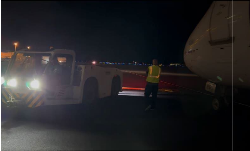
Figure 22: Tug positioned 13 ft from the airplane.
