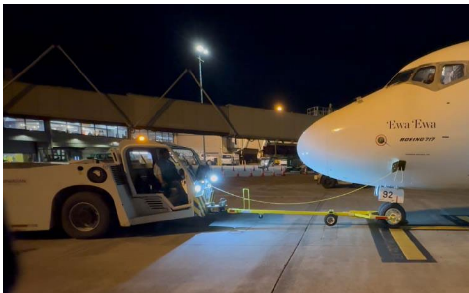
Figure 4: Tug connected to airplane by towbar and communications cable.
