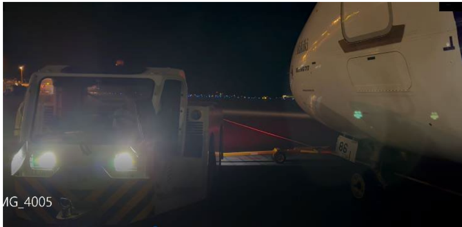
Figure 24: Tug positioned 5 ft from the side of the airplane.
