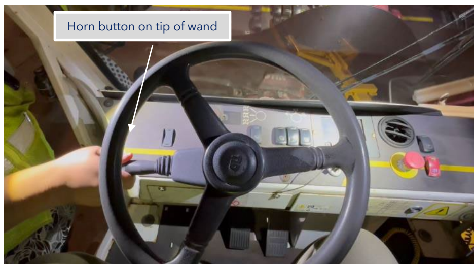
Figure 2: Tug steering wheel and wand with horn button.
