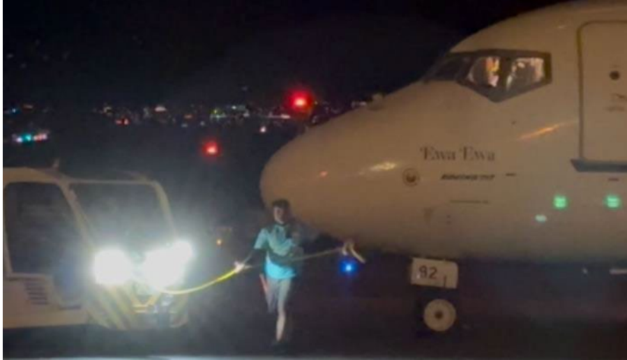
Figure 11: Escort disconnecting communication cable.
