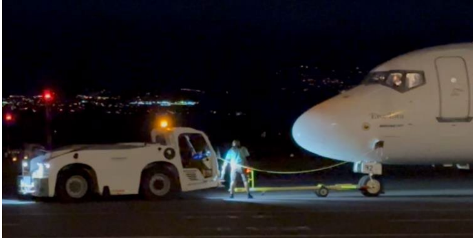
Figure 7: Escort disconnecting towbar from tug.
