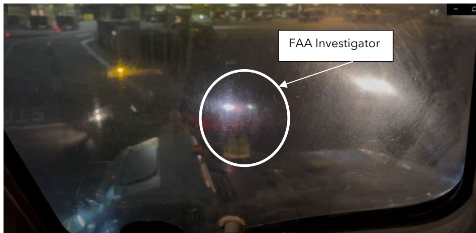
Figure 18: FAA investigator simulating display of nosewheel steering bypass pin with ribbon illuminated by a handheld flashlight.
