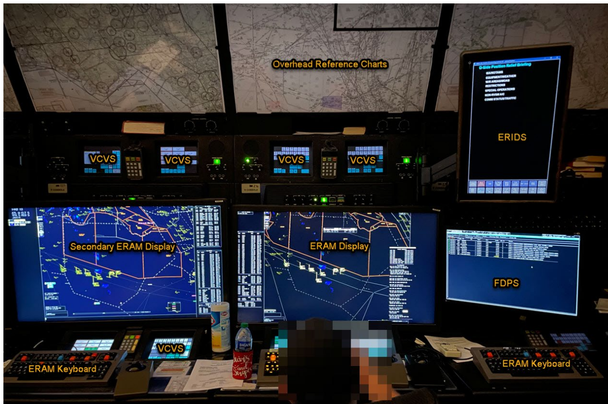
Figure 5. Photograph of the R30 / NEPTA sector position with equipment identified.
