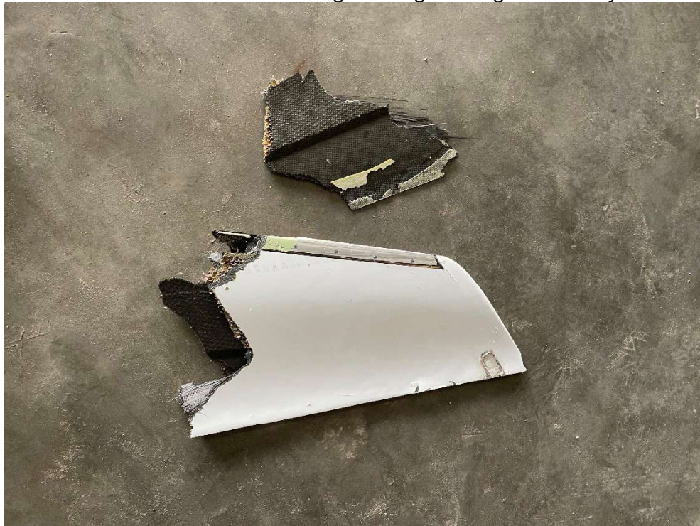
ASI-23-CQ-041 – Left Winglet Top Separated Section
