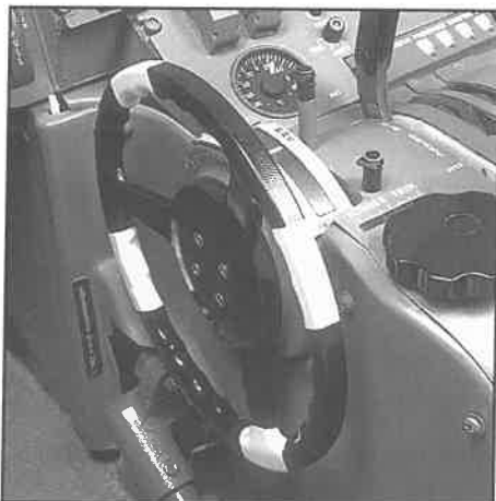
Figure 5E-9: Manual Pitch Trim System
