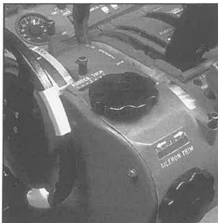
Figure 5E-12: Rudder Trim System
