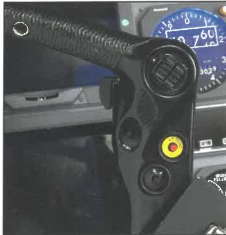
Figure 5E-10: Electric Pitch Trim System
