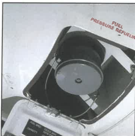
Figure 5F-15: Single-Point Coupling (Pressure Refueling)
