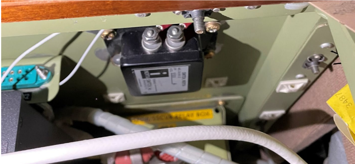
Figure 6. Impact switch on N269AA located in the aft baggage compartment/radio rack.
