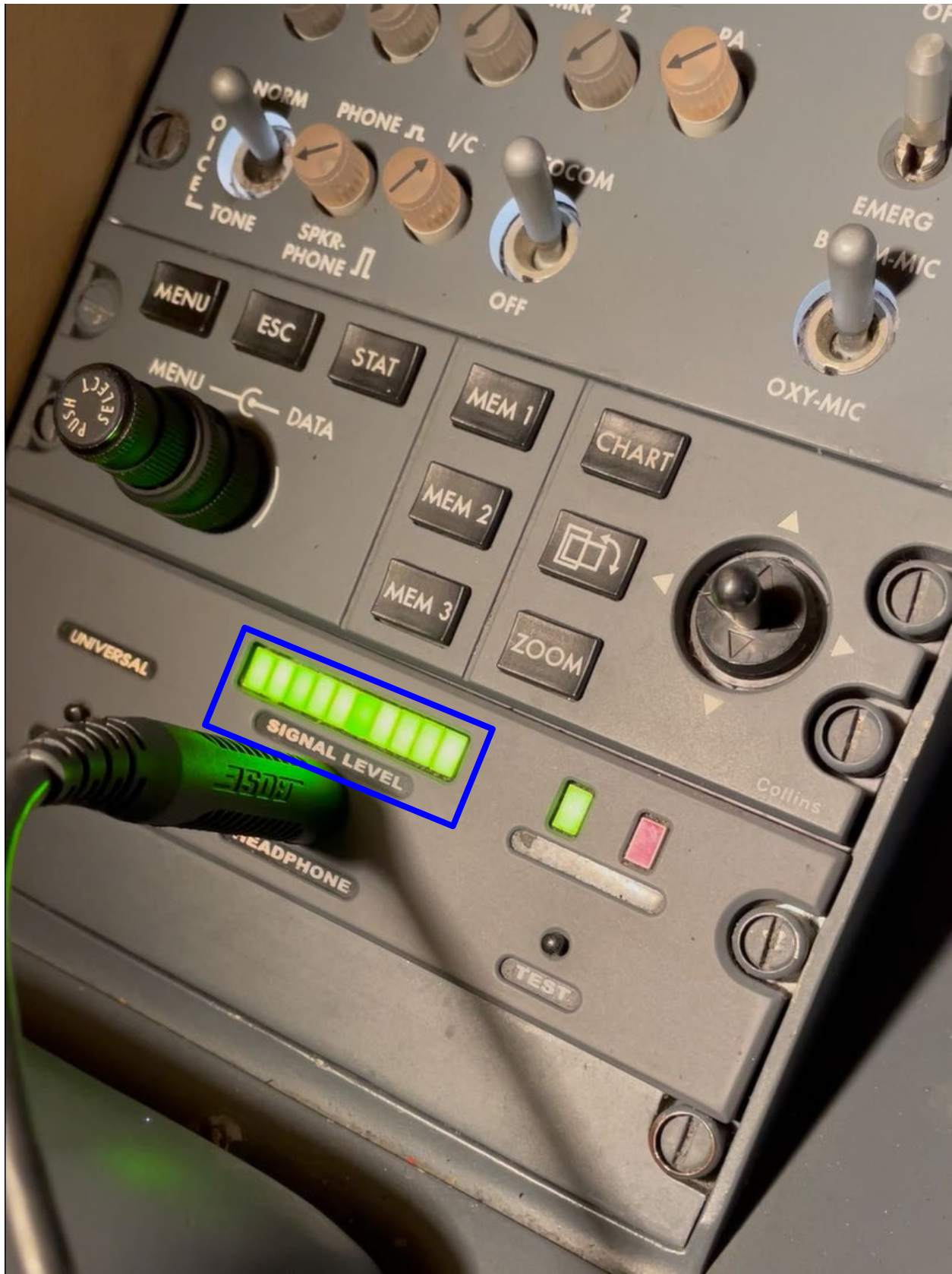
Figure 8. Control unit completing successful self-test after impact switch reset.
