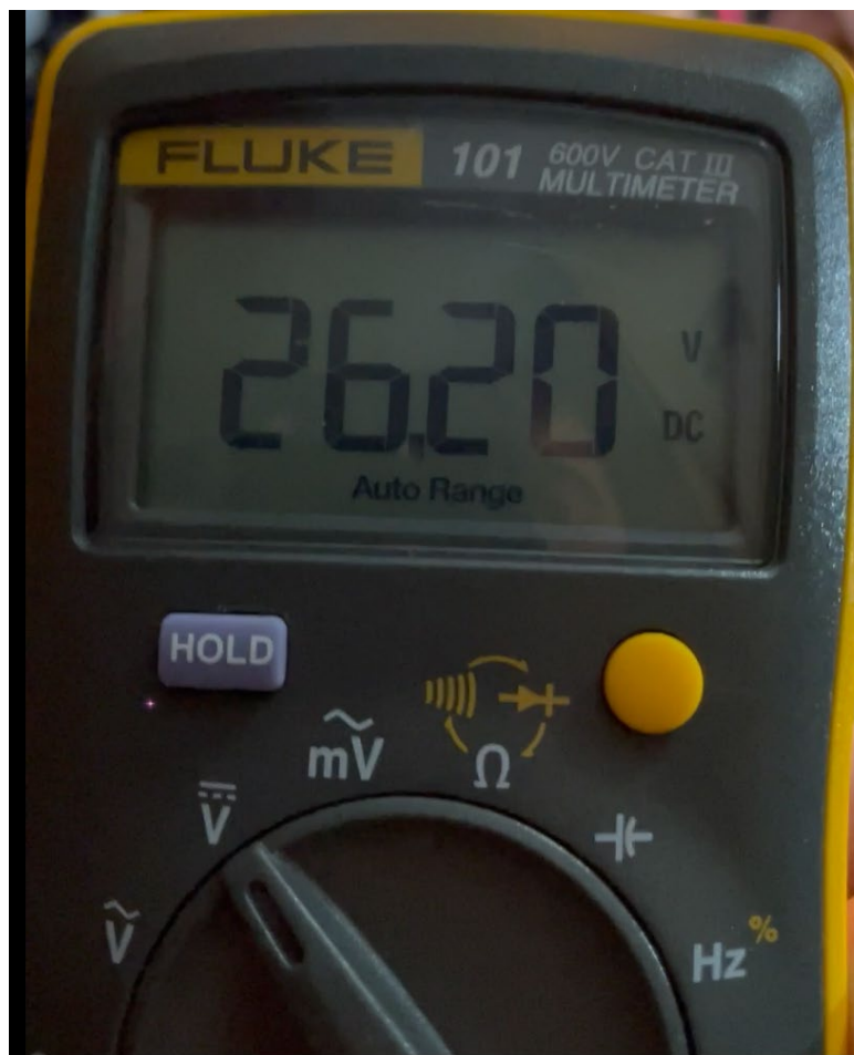
Figure 7. DC power indicated at CVR after the impact switch was reset.
