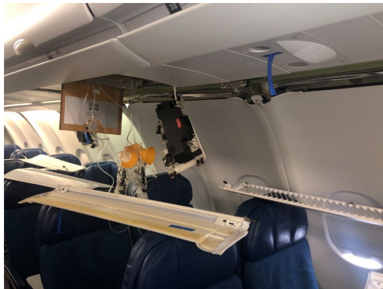
Figure 2. A passenger service unit in row 39 that fell during the turbulence.
