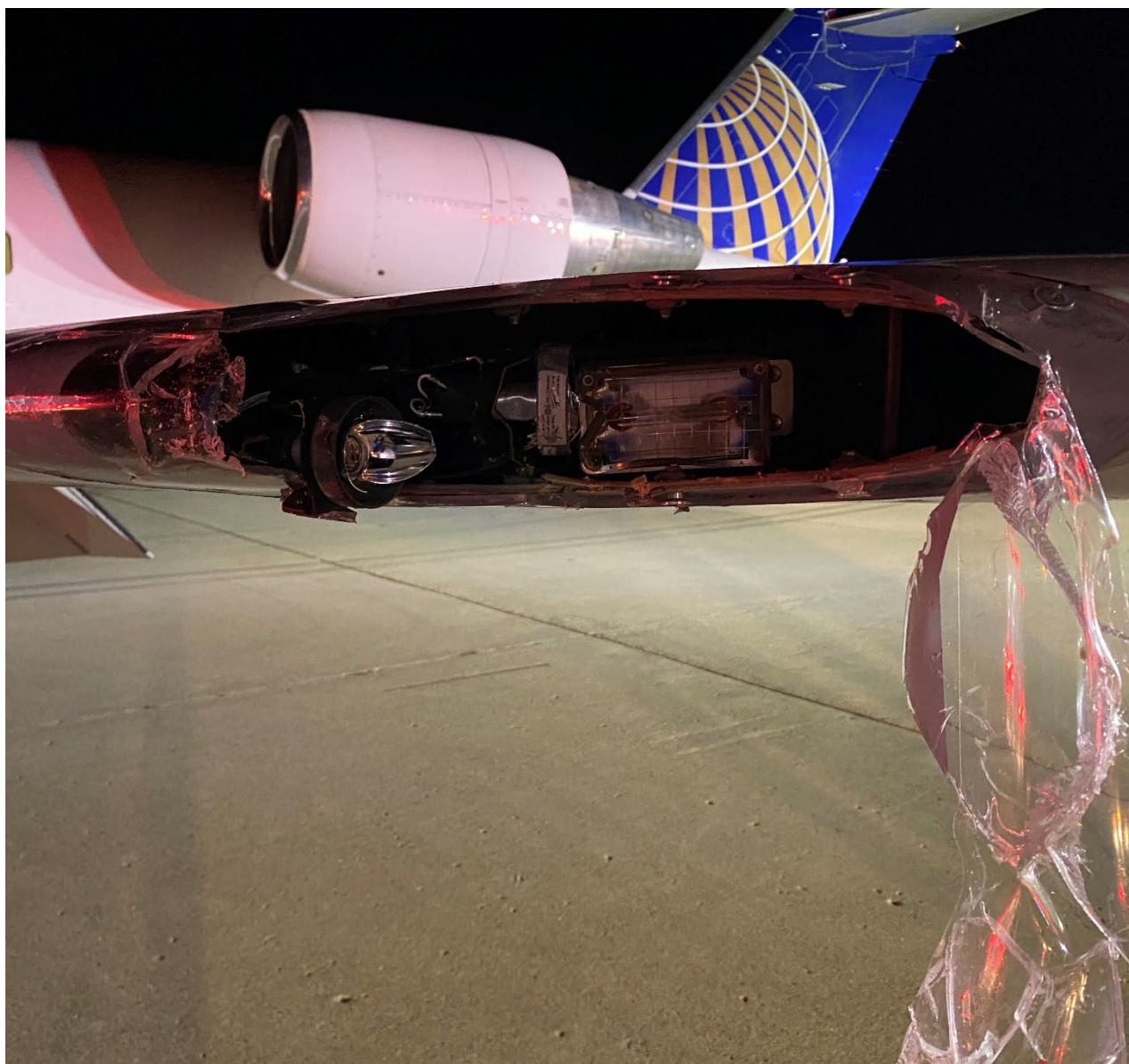
Photograph 7 - View of Minor Damage to Left Wing Tip (Courtesy Air Wisconsin)
