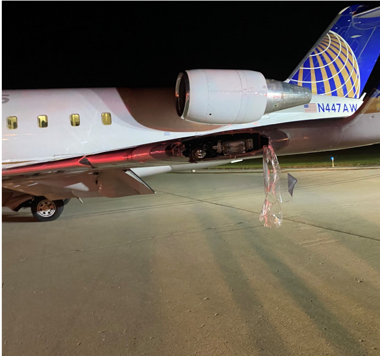
Photograph 6 - View of Minor Damage to Left Wing (Courtesy Air Wisconsin)
